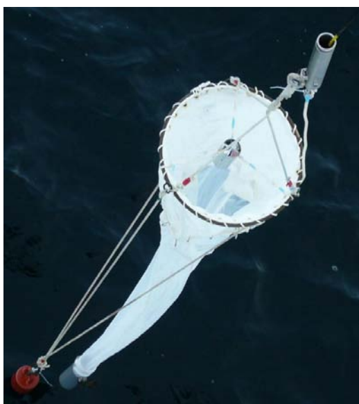
Fig. 3.1-2 NORPAC net with closing system
