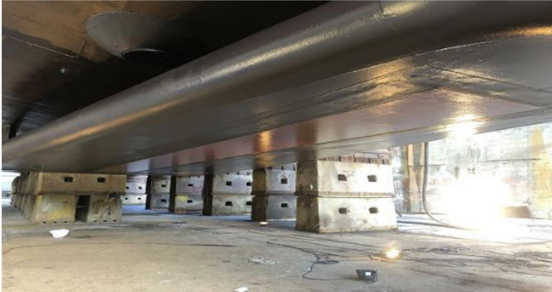
Figure 3: Kongsberg EM 124 gondola attached to the hull of the DSSV Pressure Drop (image: Tony Dahlheim).
