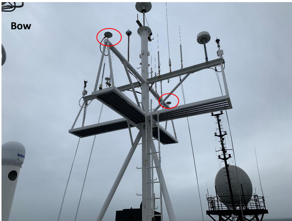
Figure 5: GPS antennas mounted at the top of the ship near the bow.
