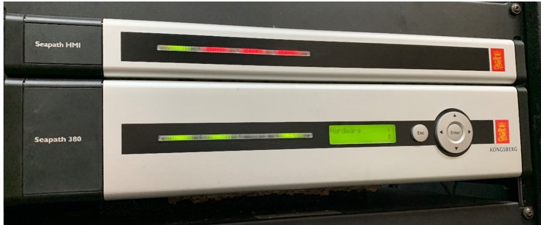
Figure 4: Kongsberg Seapath 380 in the systems rack of the electronics lab on the DSSV Pressure Drop.
