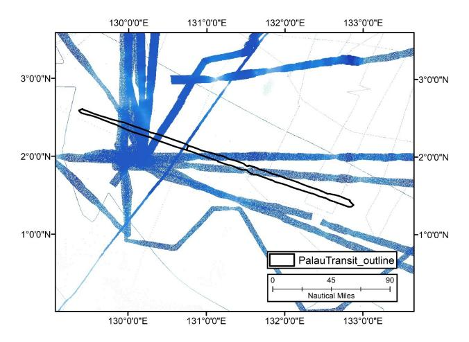
Majority of the transit data did not intersect sounding data from multibeam and single beam. Specifically, 70% of these transit data covered previously interpolated areas and are new data to the world.
