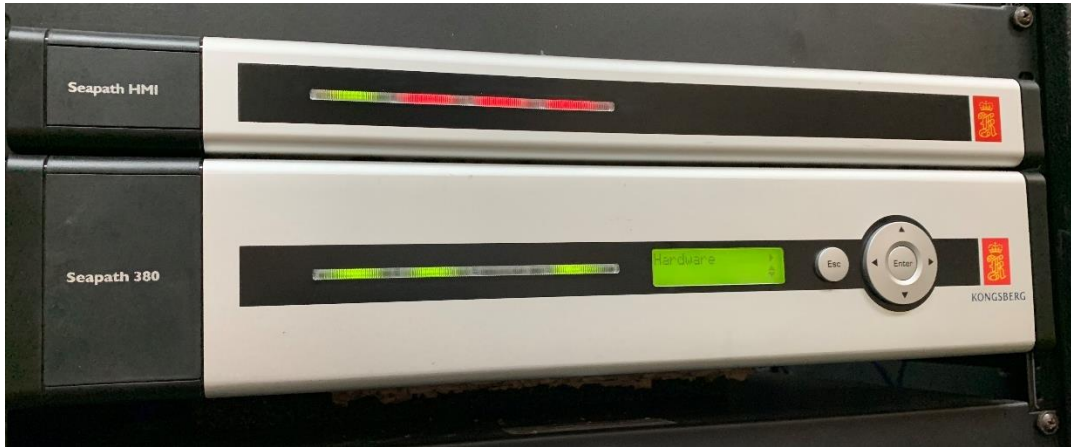
Figure 4: Kongsberg Seapath 380 in the systems rack of the electronics lab on the DSSV Pressure Drop.
