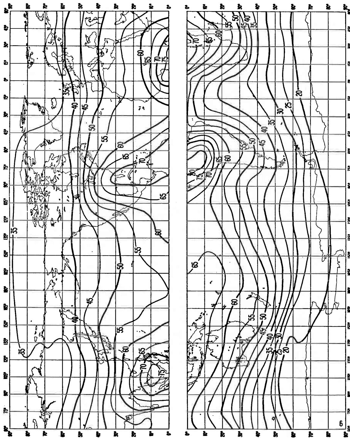
FIGURE 9a – Expected values of atmospheric radio noise,  $F_{am}$  (dB above  $kT_0b$  at 1 MHz)
