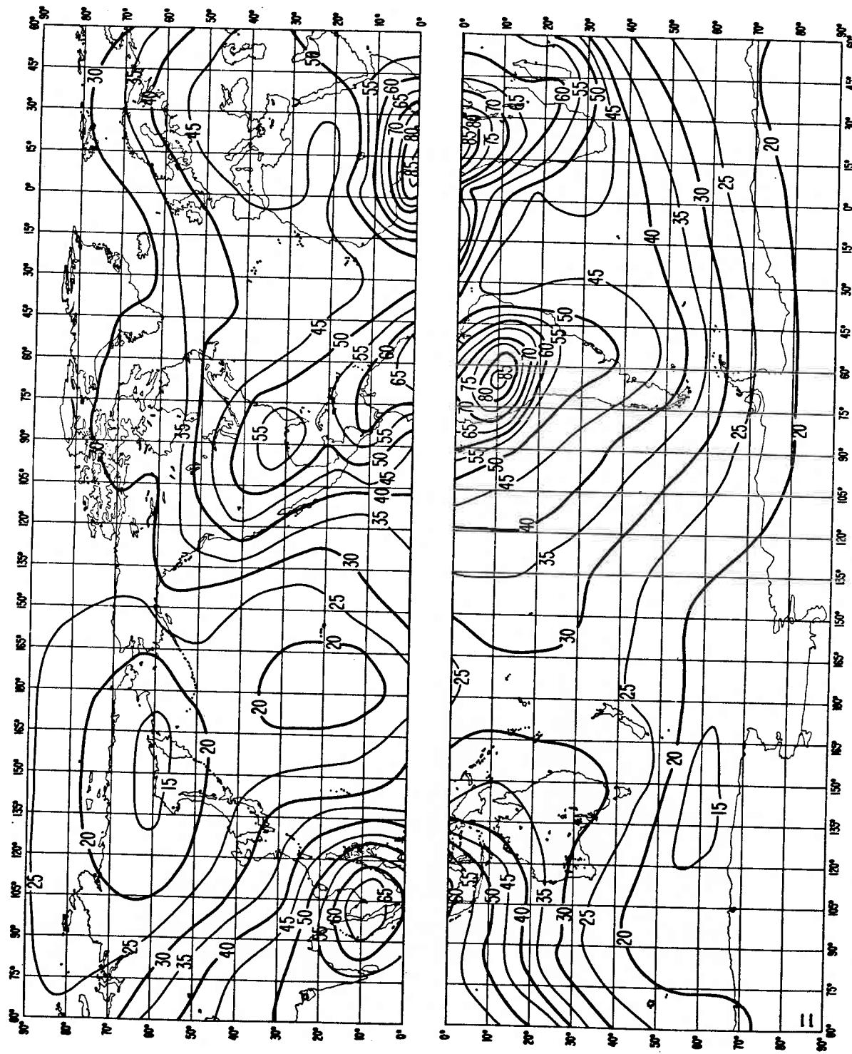
FIGURE 11a – Expected values of atmospheric radio noise,  $F_{am}$  (dB above  $kT_{ob}$  at 1 MHz)
