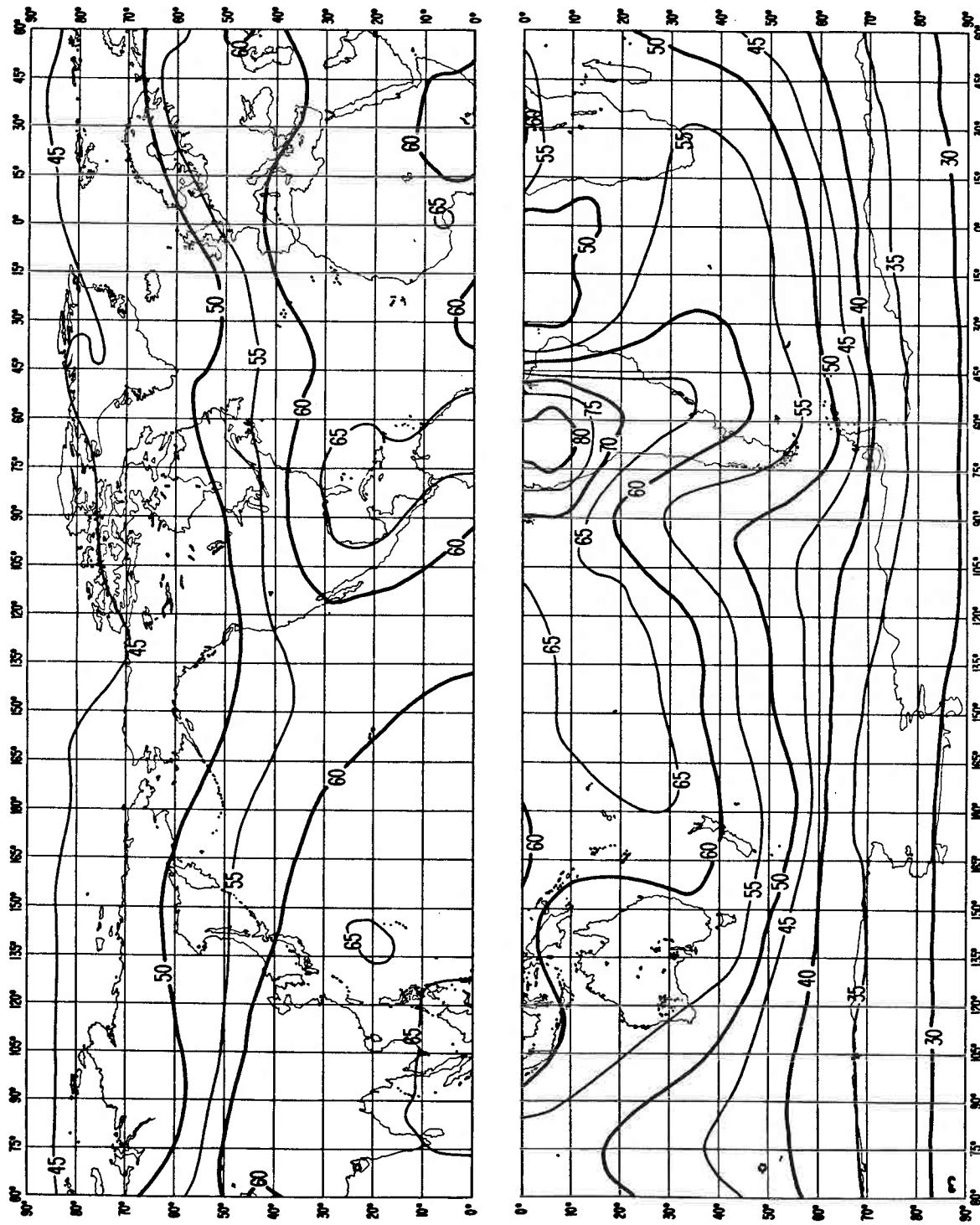
FIGURE 3a - Expected values of atmospheric radio noise,  $F_{am}$  (dB above  $kT_0b$  at 1 MHz)
