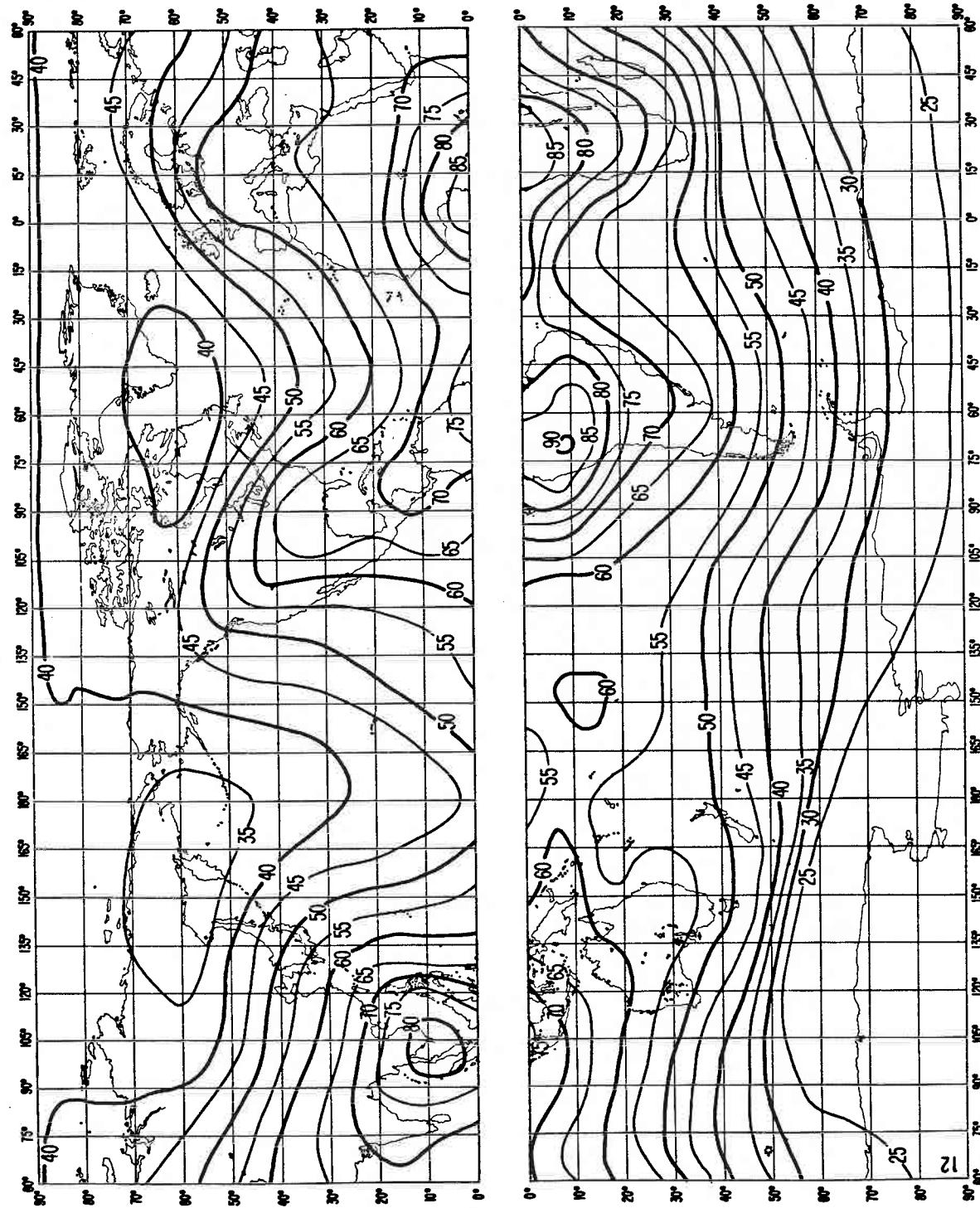
FIGURE 12a - Expected values of atmospheric radio noise,  $F_{mn}$  (dB above  $kT_{ob}$  at 1 MHz)
