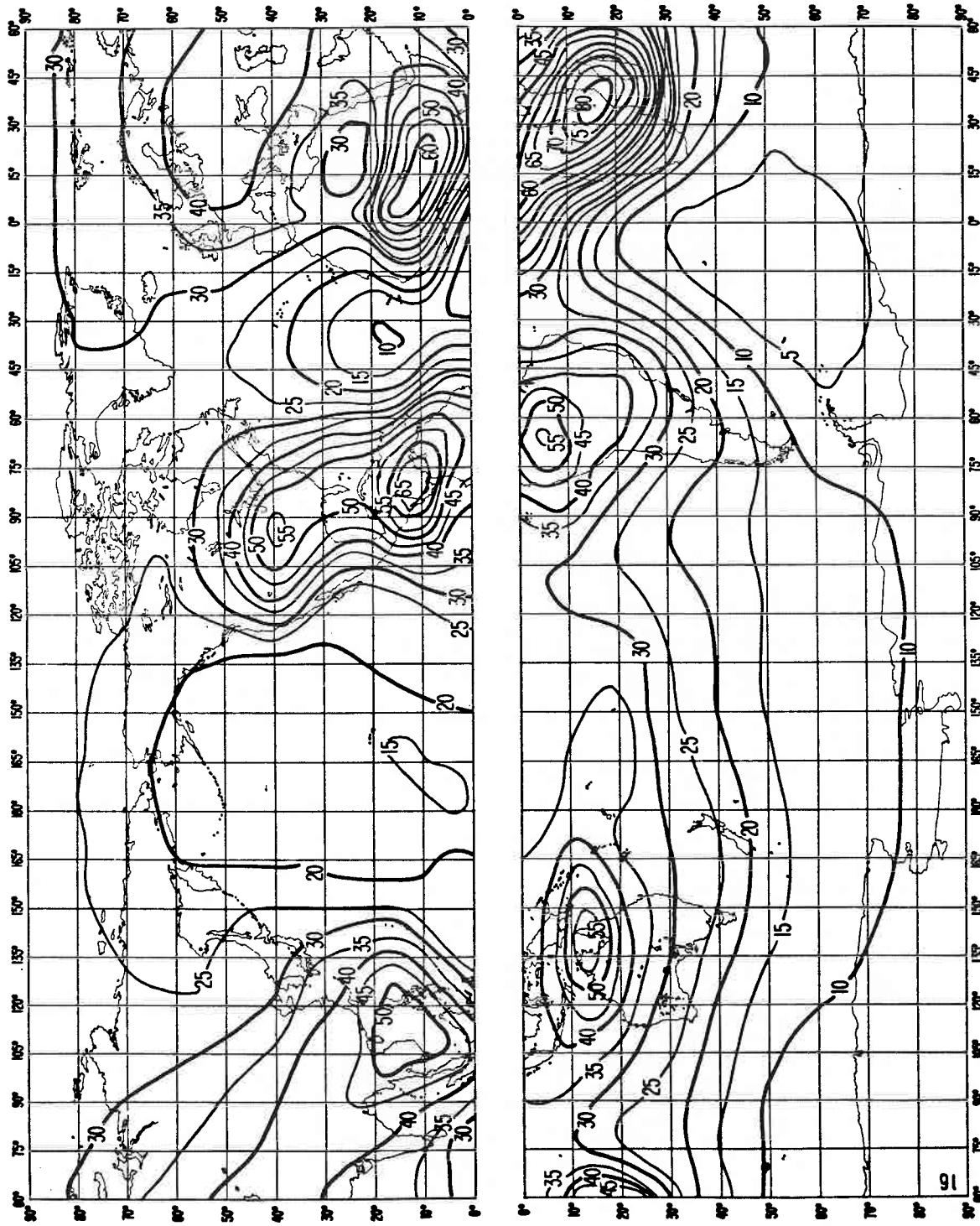
FIGURE 16a – Expected values of atmospheric radio noise,  $F_{am}$  (dB above  $kT_0b$  at 1 MHz)
