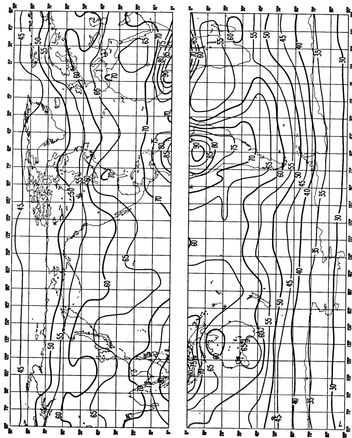
FIGURE 7a - Expected values of atmospheric radio noise,  $F_{am}$  (dB above  $kT_0b$  at 1 MHz)
