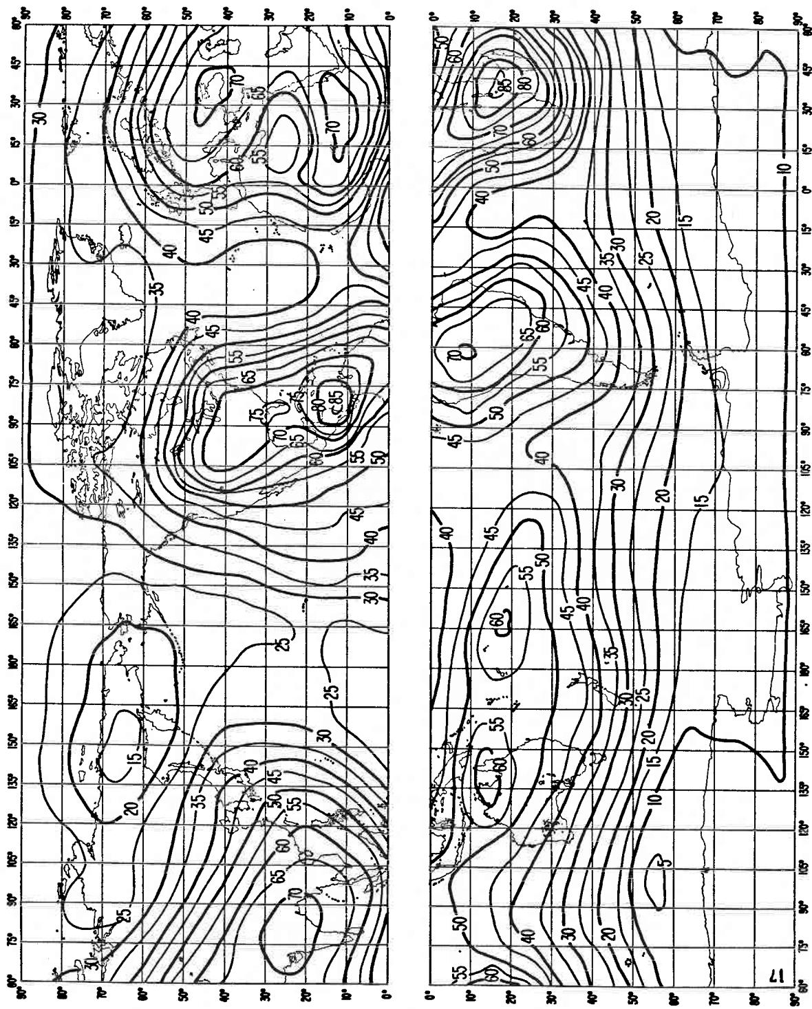
FIGURE 17a - Expected values of atmospheric radio noise,  $F_m$  (dB above  $kT_0b$  at 1 MHz)
