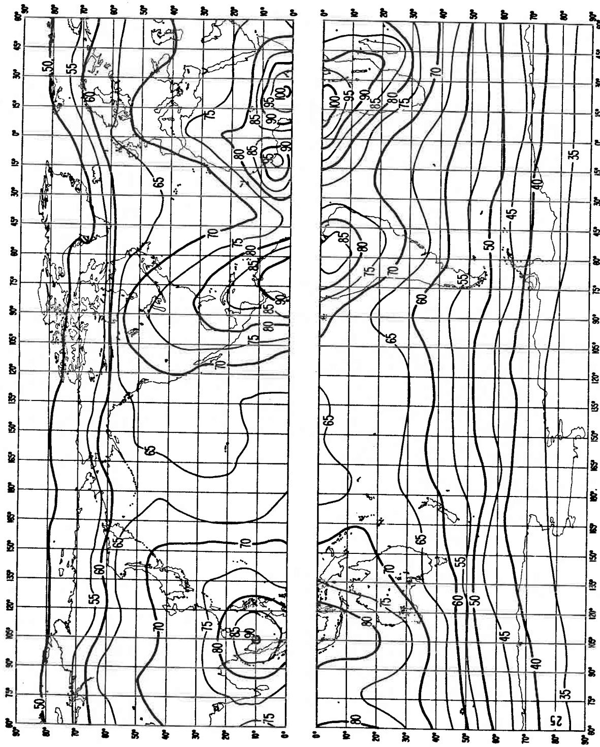
FIGURE 25a - Expected values of atmospheric radio noise,  $F_{atm}$  (dB above  $kT_0b$  at 1 MHz)
