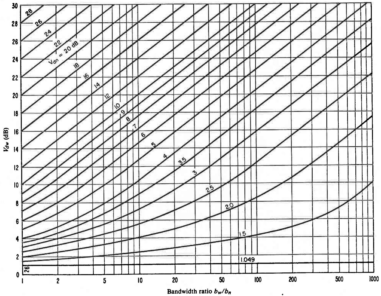
FIGURE 26 – Conversion of  $V_d$  in one bandwidth to  $V_{dw}$  in another bandwidth
