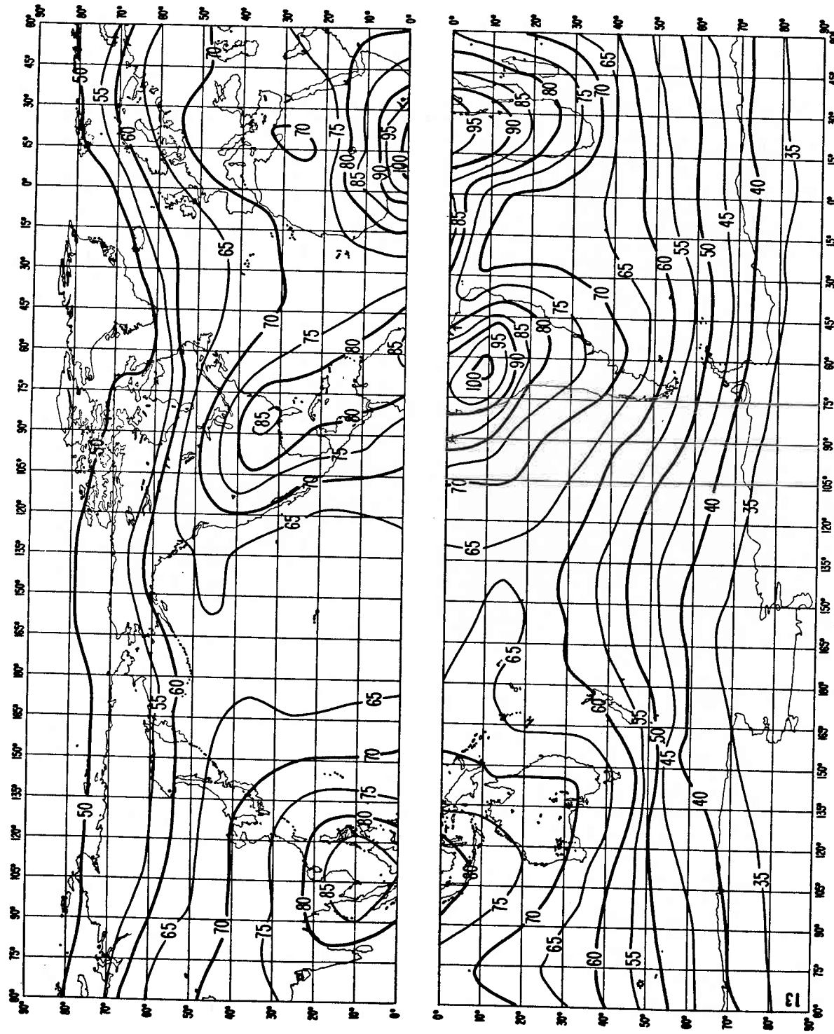
FIGURE 13a - Expected values of atmospheric radio noise,  $F_{am}$  (dB above  $kT_0b$  at 1 MHz)
