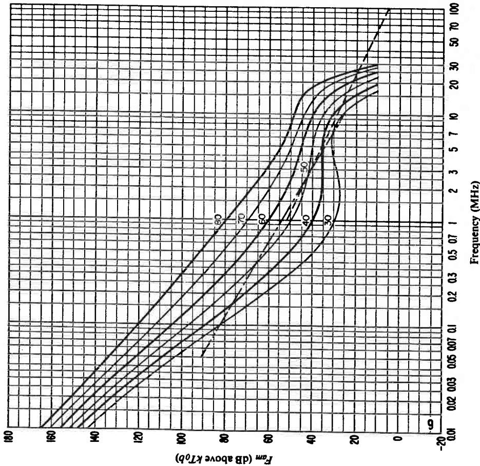
FIGURE 6b – Variation of radio noise with frequency
