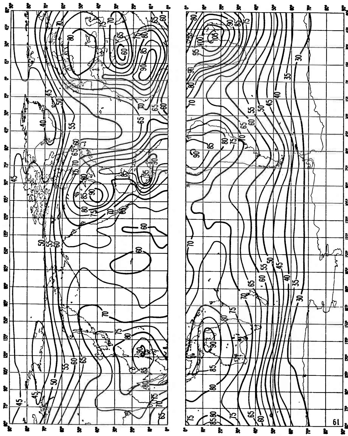
FIGURE 19a – Expected values of atmospheric radio noise,  $F_{am}$  (dB above  $kT_0b$  at 1 MHz)
