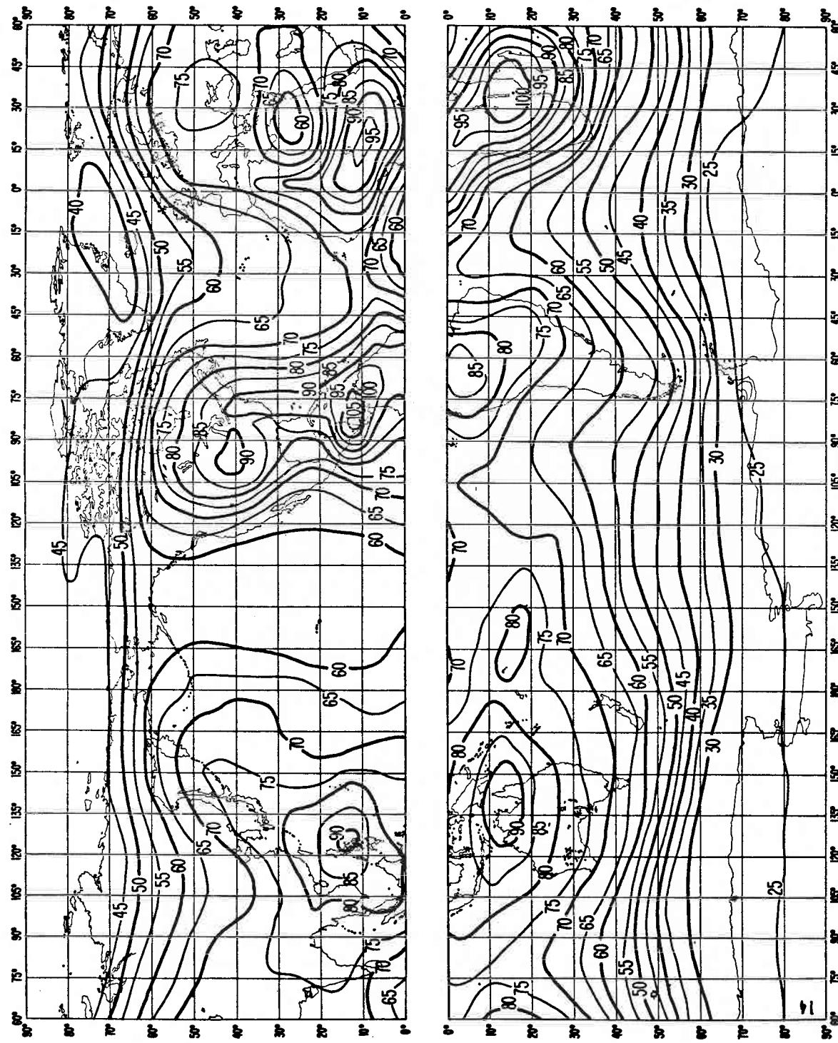
FIGURE 14a - Expected values of atmospheric radio noise,  $F_m$  (dB above K10b at 1 MHz)
