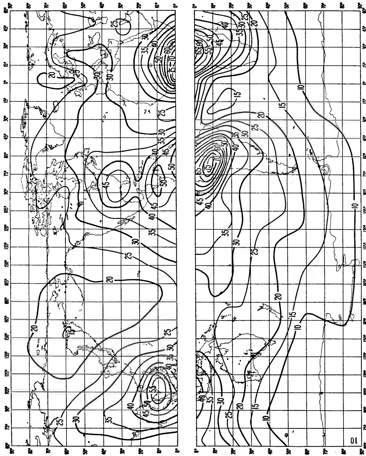
FIGURE 10a - Expected values of atmospheric radio noise,  $F_{am}$  (dB above  $kT_0 b$  at 1 MHz)
