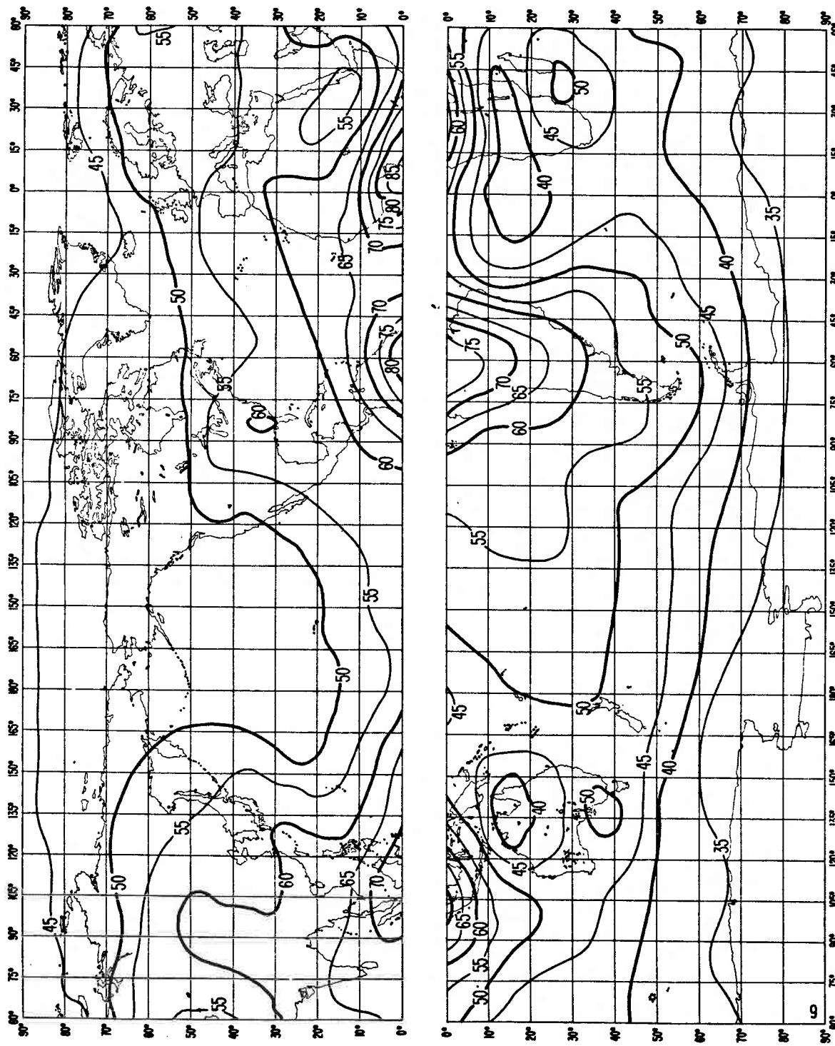
FIGURE 6a - Expected values of atmospheric radio noise,  $F_{amb}$  (dB above  $kT_0b$  at 1 MHz)
