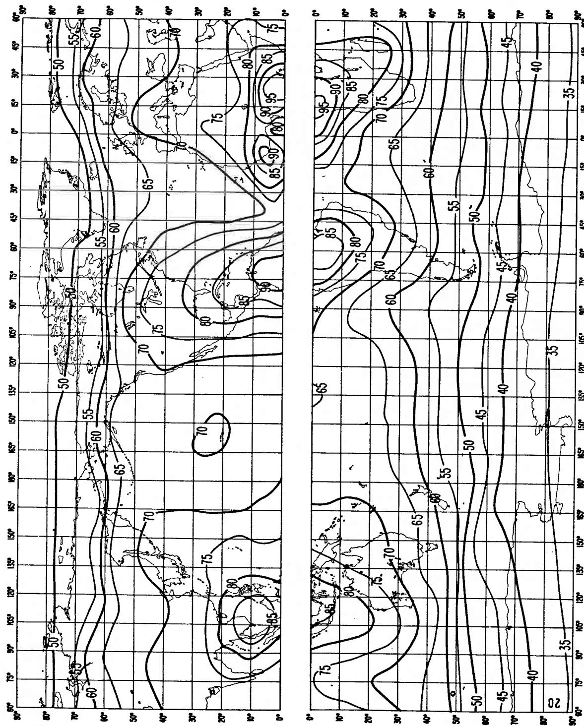
FIGURE 20a - Expected values of atmospheric radio noise,  $F_{att}$  (dB above  $kT_0b$  at 1 MHz)
