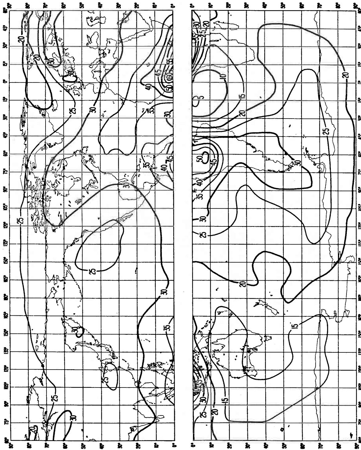
FIGURE 4a - Expected values of atmospheric radio noise,  $F_{am}$  (dB above  $kT_0 b$  at 1 MHz)
