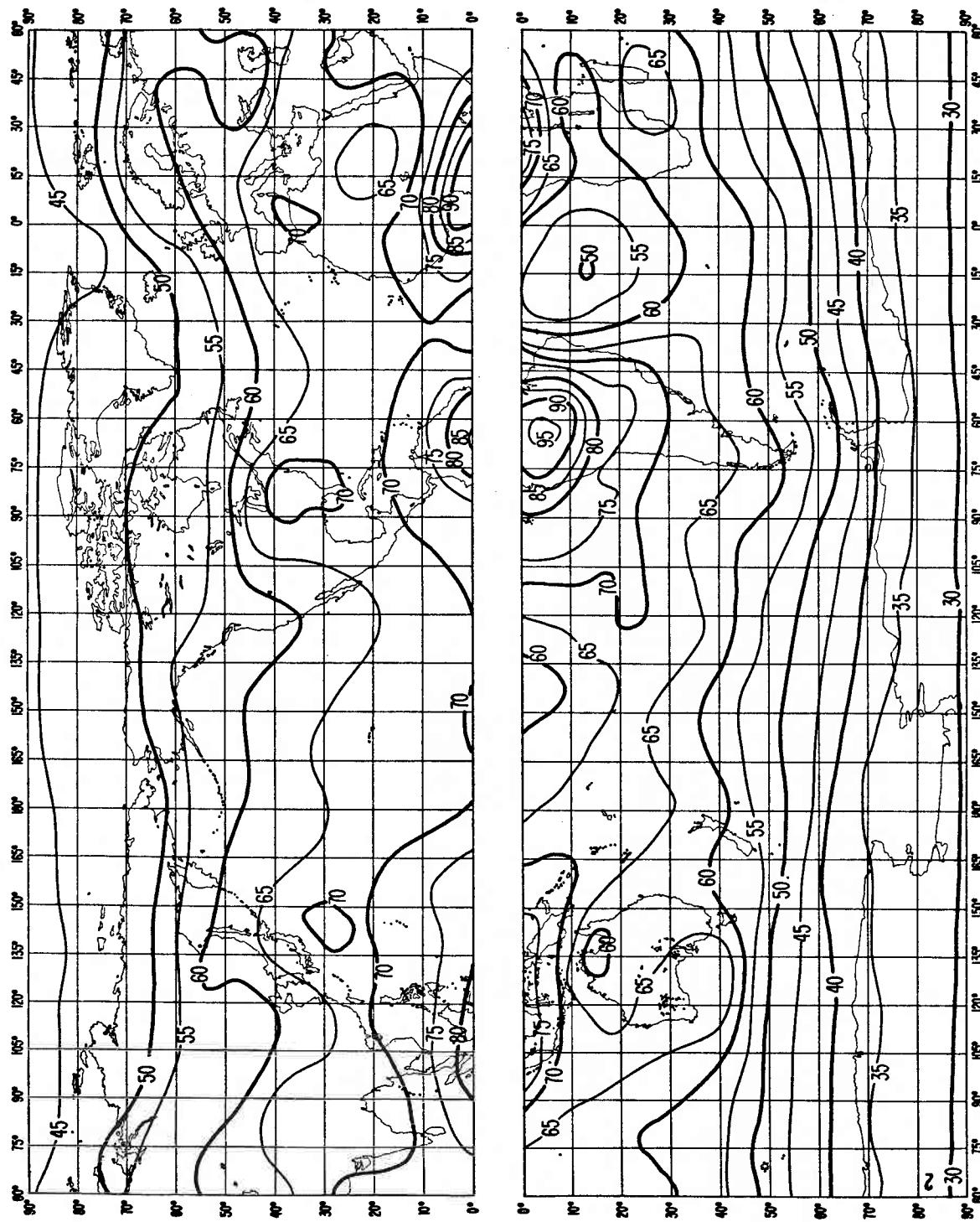
FIGURE 2a – Expected values of atmospheric radio noise,  $F_{atm}$  (dB above  $kT_0 b$  at 1 MHz)
