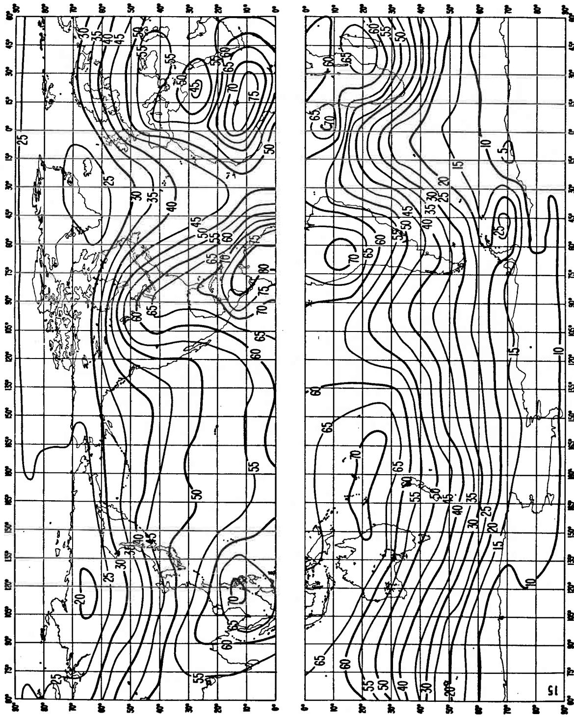
FIGURE 15a – Expected values of atmospheric radio noise,  $F_m$  (dB above  $kT_0B$  at 1 MHz)
