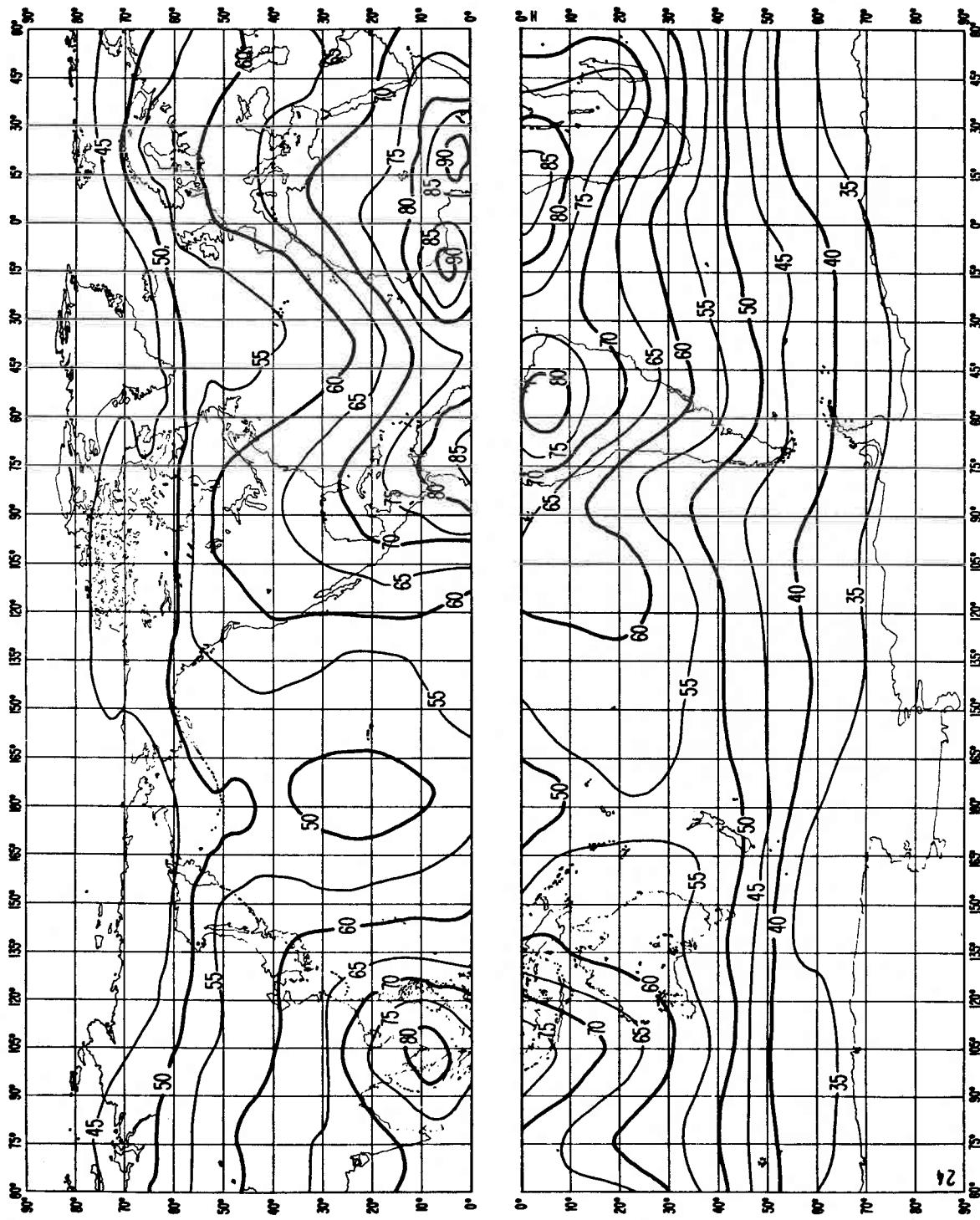
FIGURE 24a - Expected values of atmospheric radio noise,  $F_m$  (dB above  $kT_0b$  at 1 MHz)
