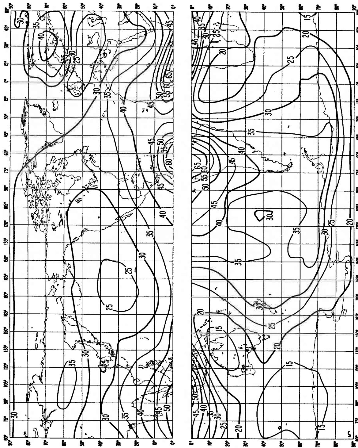
FIGURE 5a – Expected values of atmospheric radio noise,  $F_{am}$  (dB above  $kT_0b$  at 1 MHz)
