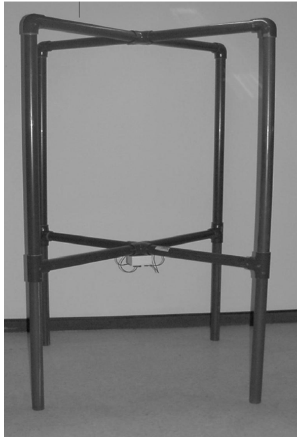
Figure 1-1B Magnetic Loop Turnstile Antenna with attached preamp module
