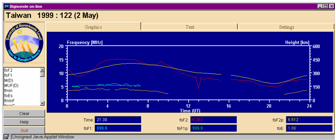
Figure 4-8 Time series of ionospheric characteristics obtained using local archive of SAO files.
