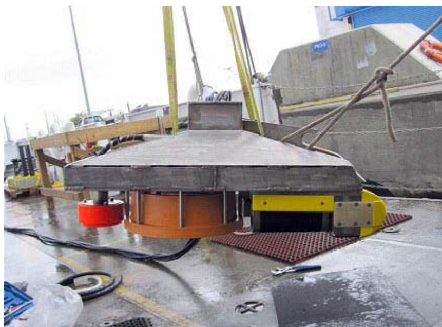
Fig 4: Reson 7125 SV mounted onto moonpool sled
