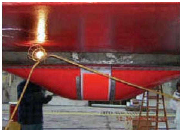
Fig 2: EM1002 transducer fairing
