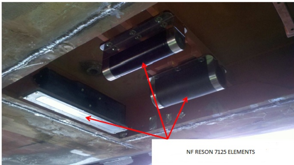
Fig 4: Reson 7125 mounted onto the hull of the Nancy Foster
