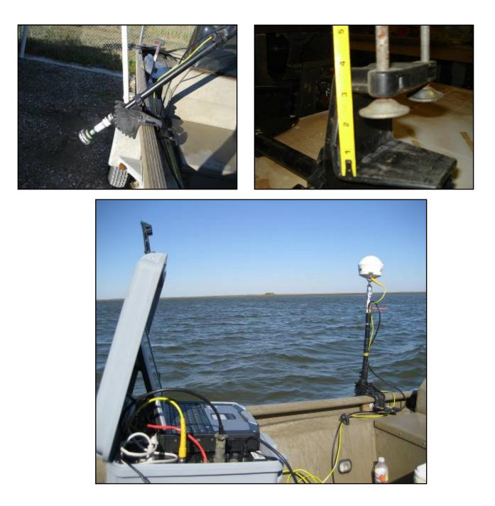
The pole mount was secured to the gunwale of the vessel using hand tightened thumb screws displayed in the image(s) above. The mounting pole was constructed of a heavy grade composite material and ran through the fitted opening of the mount and secured in place with an additional hand tightened thumb screw. Once mounted, the arm and mount remained in the same location for the duration of the project.
