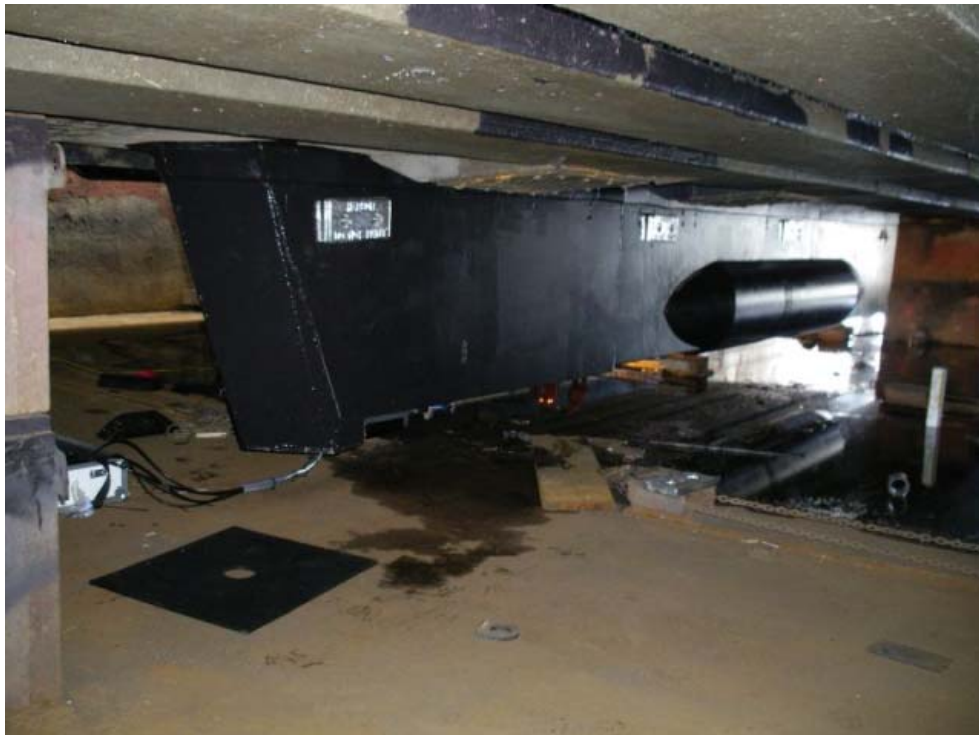
Figure 7 – F/V Pacific Star Drop Keel with 7125 and 8111 Sonar Heads
