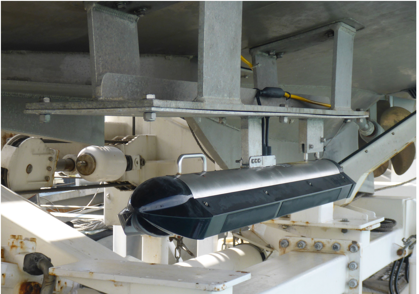
Figure 9: The EdgeTech model 4200 (300/600kHz) side scan sonar fish as hull-mounted on 2804 (RA6).
