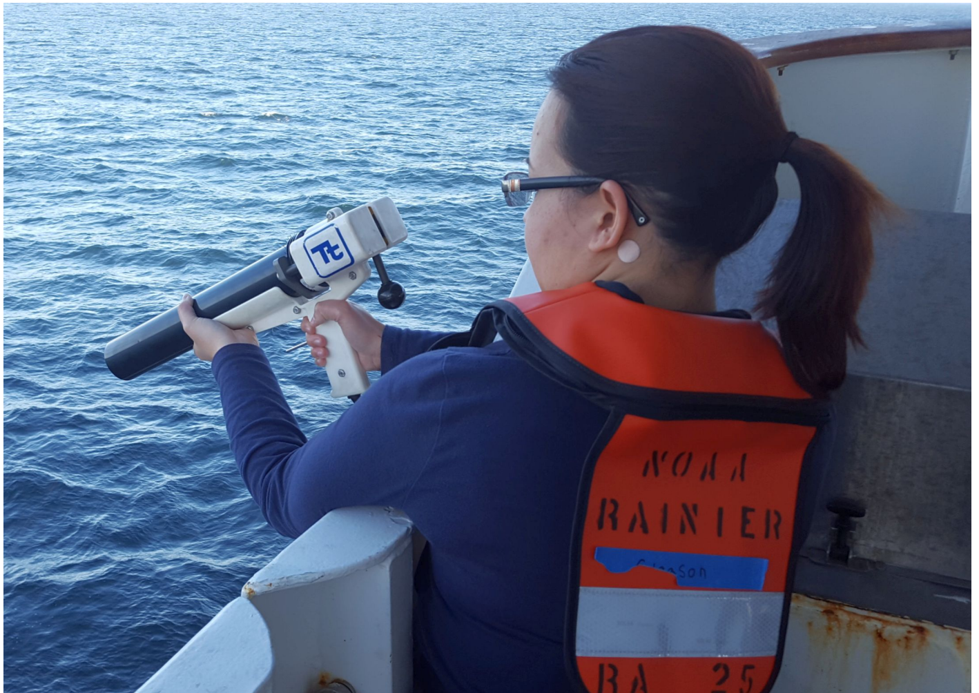
Figure 17: Deploying a XBT from the port-side bridge wing of Rainier.
