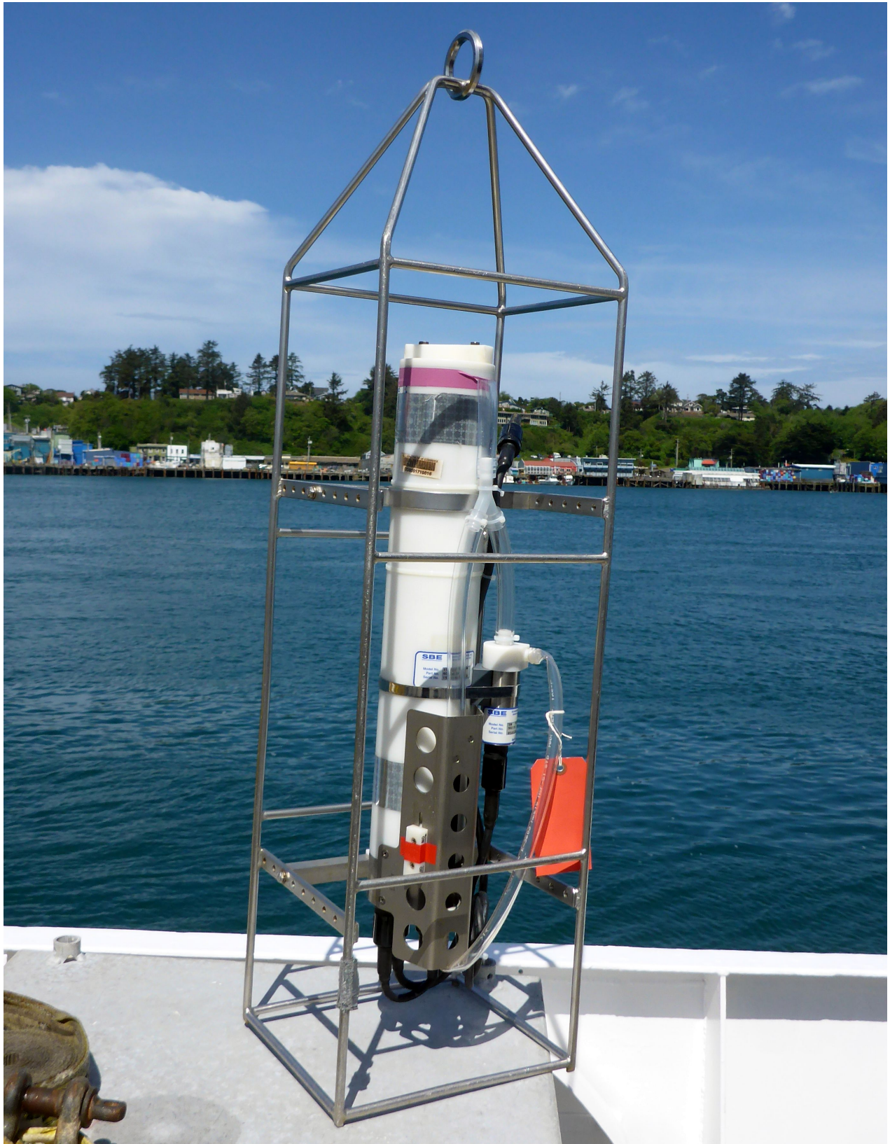
Figure 16: The SBE 19plus SEACAT profiler. Note the band of electrical tape around the housing at the top of profiler marking this as the "purple" CTD.
