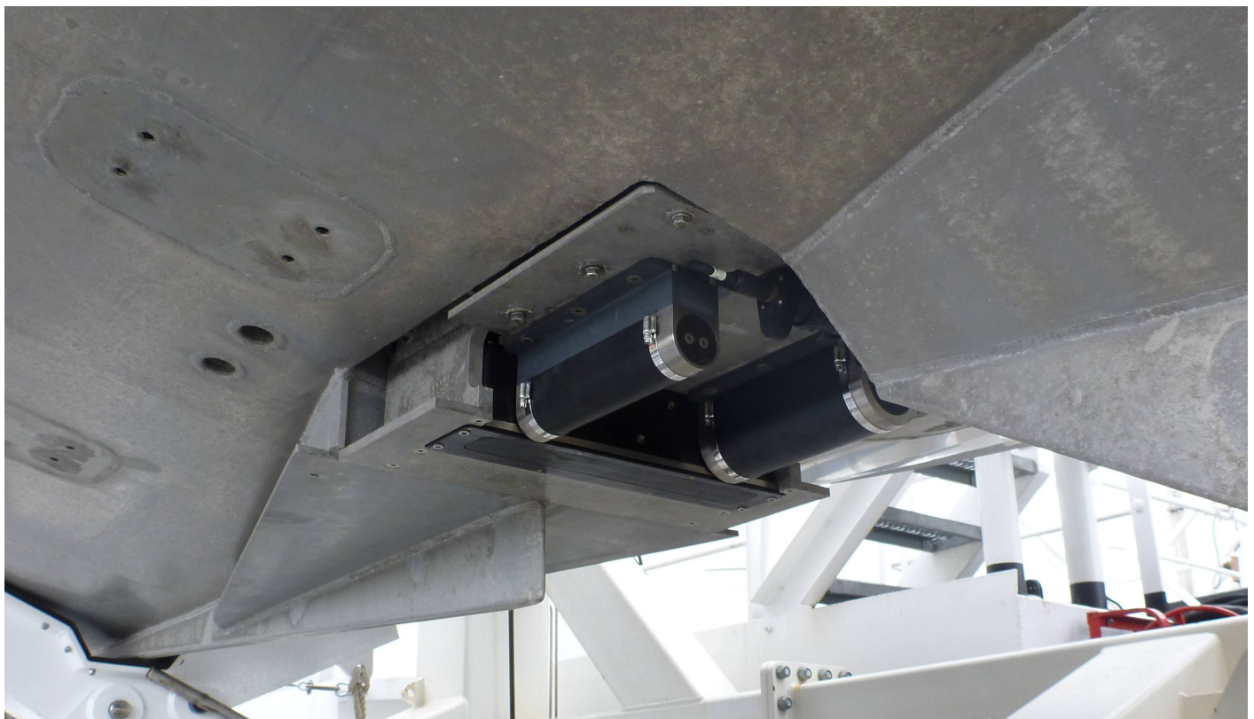
Figure 11: Reson SeaBat 7125-B mounted on survey launch 2801.
