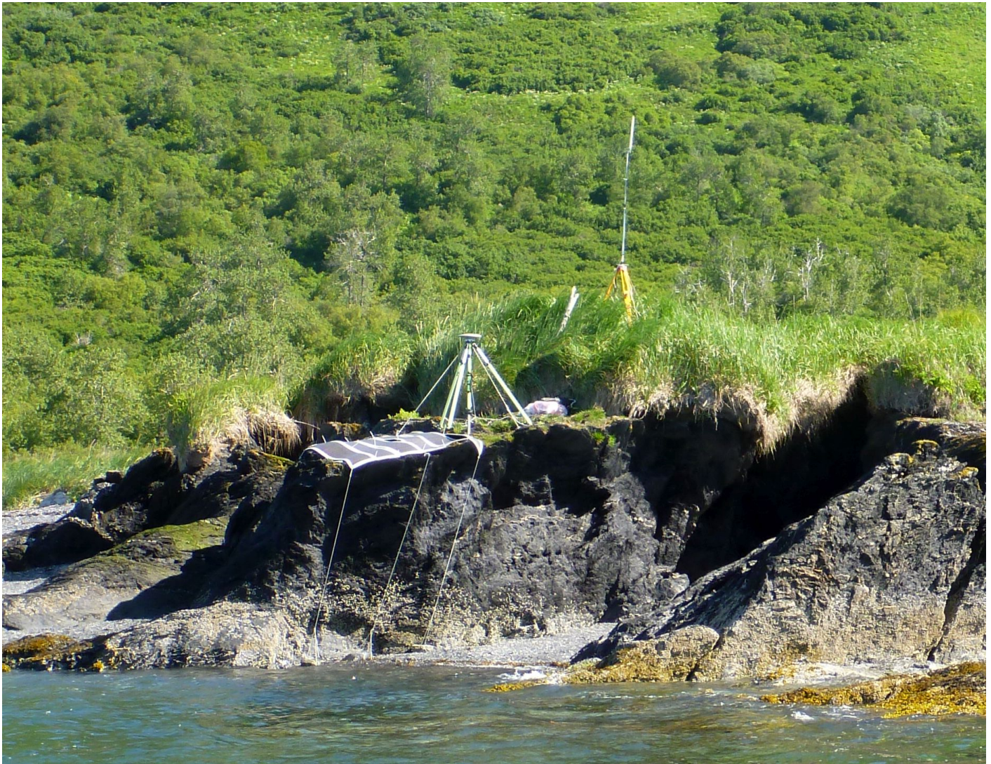
Figure 26: A Rainier base station installed in Uganik Bay, Alaska.
