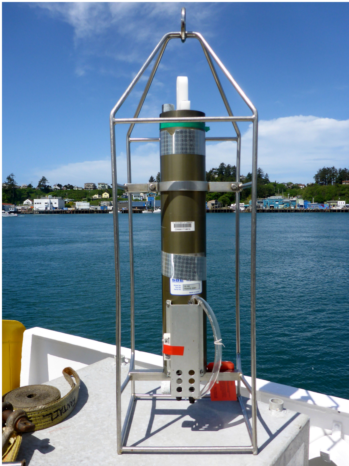
Figure 15: The SEACAT SBE 19 profiler. Note the band of electrical tape around the housing at the top of profiler marking this as the "green" CTD.
