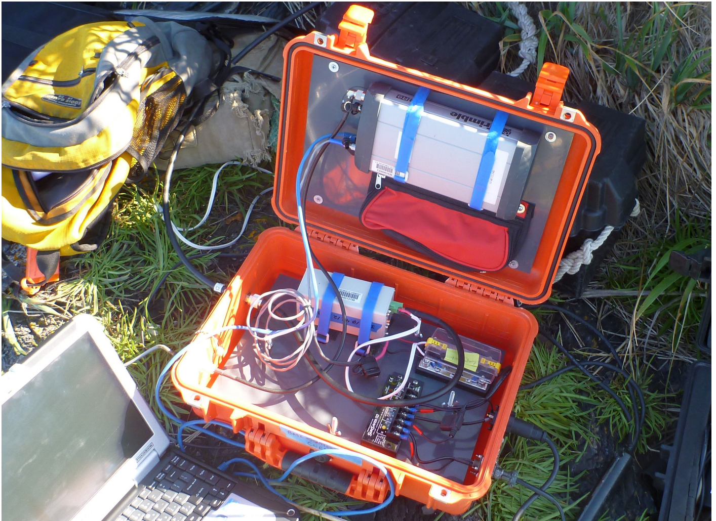
Figure 20: Base station "Curly" consisting of a Trimble NetR5 receiver interfaced with a Freewave Ethernet radio and associated power control electronics all sealed in a watertight Pelican plastic case.
