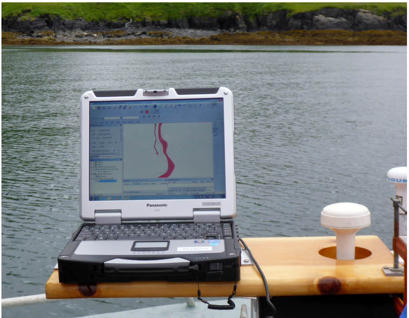
Figure 13: A Toughbook laptop computer Field5 in use on a skiff collecting shoreline data.
