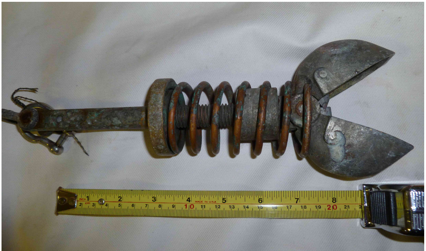
Figure 21: The “Nibbler”, a foot-trip clam shell style bottom sampler.
