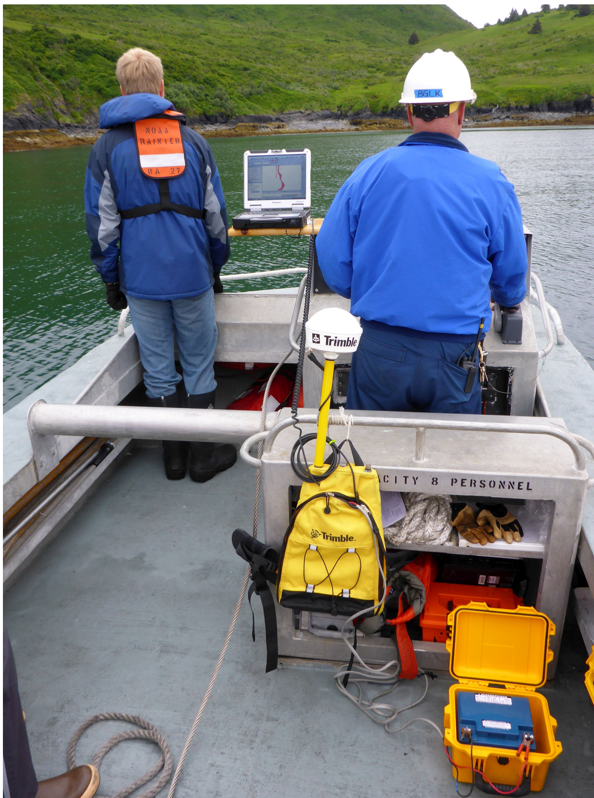
Figure 27: Survey skiff RA8 collecting the along-shore buffer line using a Trimble GPS backpack system connected to an external battery and a Toughbook computer.
