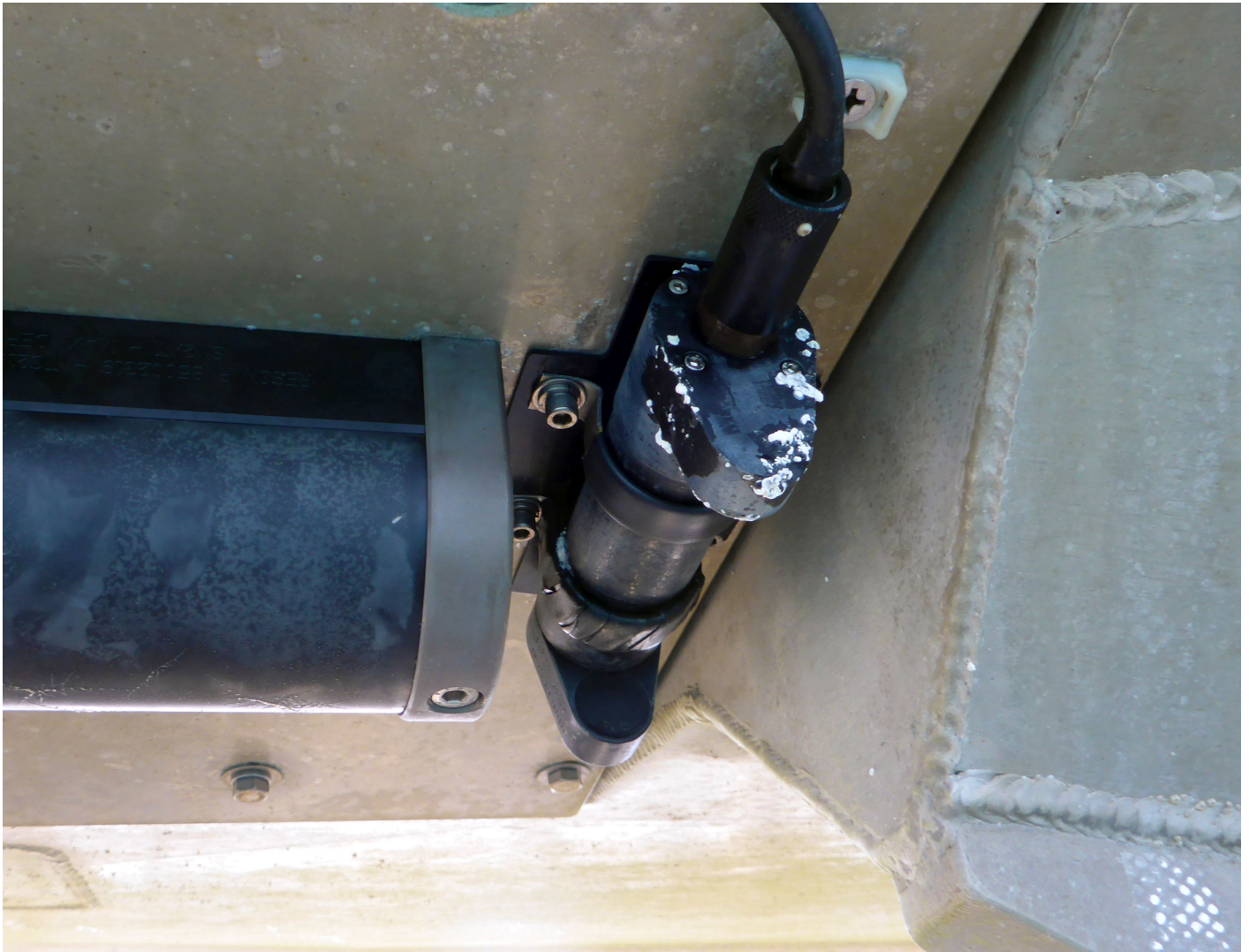
Figure 19: A SVP 71 mounted just aft of a Reson multibeam transducer on a survey launch.
