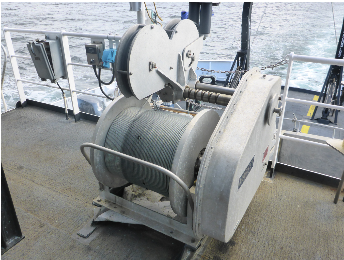
Figure 8: The Markey COM-7X Compact CTD Winch as mounted on the boat deck of Rainier.
