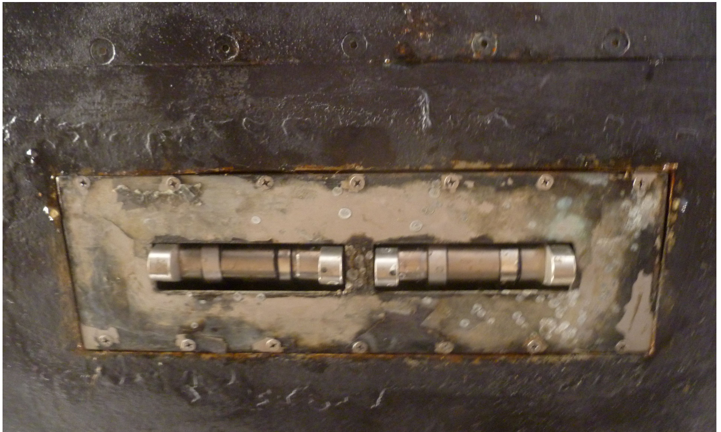
Figure 18: Dual SVP 70s mounted in Rainier's multibeam sonar transducer gondola.
