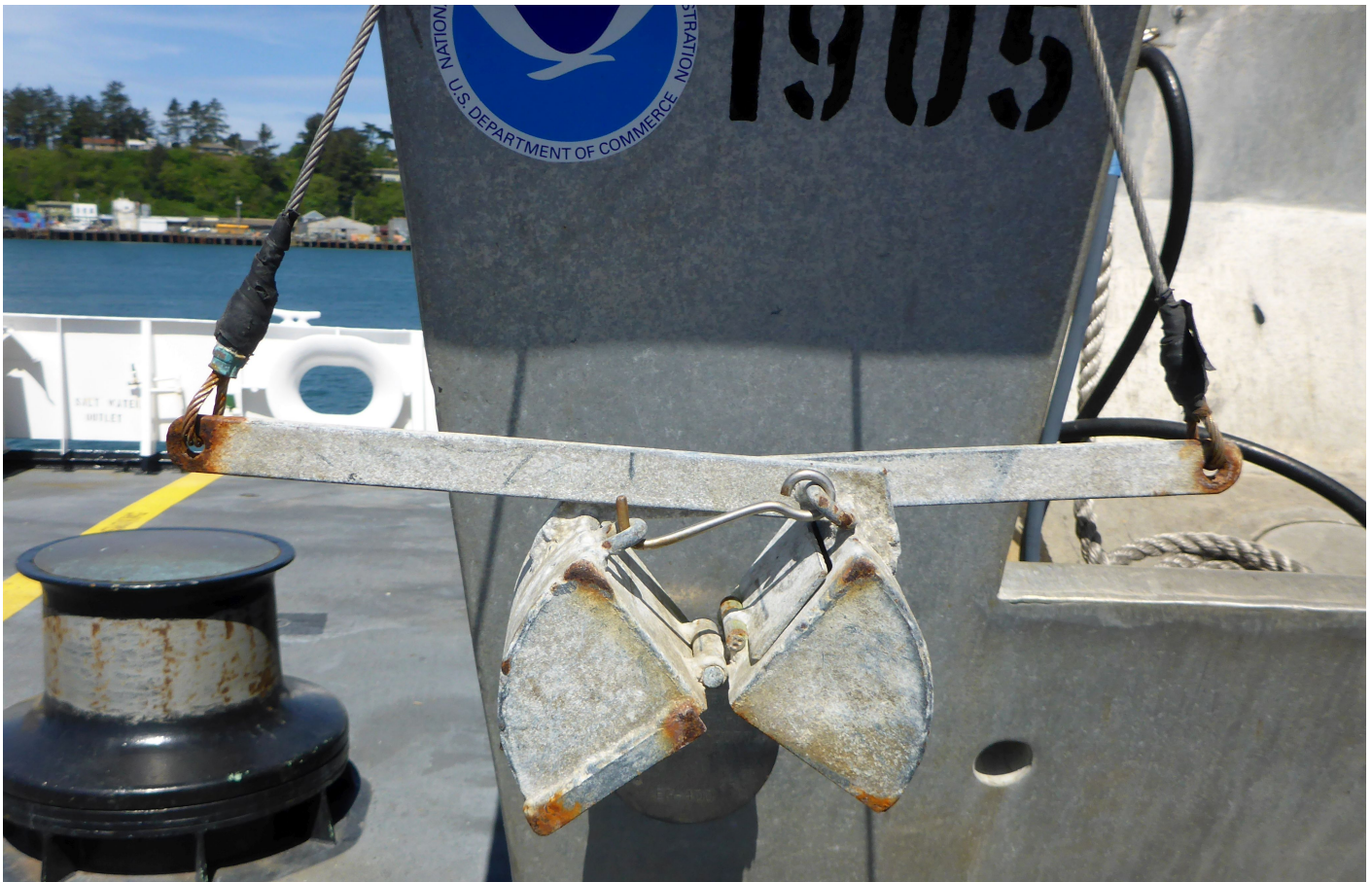
Figure 23: The Van Veen grab sampler configured ready to deploy.
