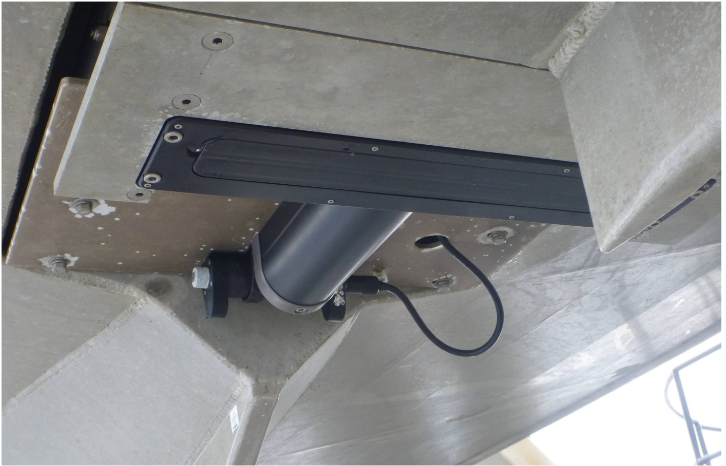
Figure 12: Reson SeaBat 7125 SV2 mounted on survey launch 2804.
