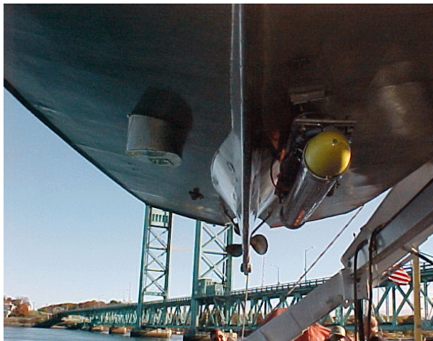
Figure 5: Hull mounted Klein towfish under Launch 1014
