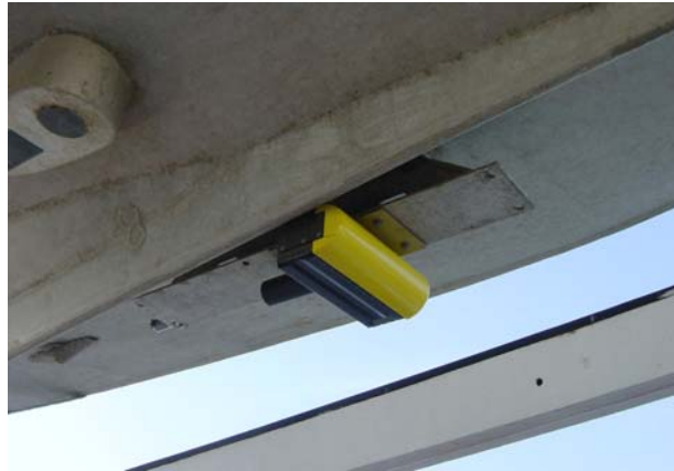
Figure 2: Hull-mounted Reson 8125 transducer attached; yellow facing towards the bow.
