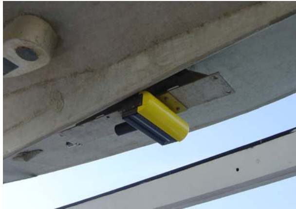
Figure 2: Hull-mounted Reson 8125 transducer attached; yellow fairing facing towards the bow.
