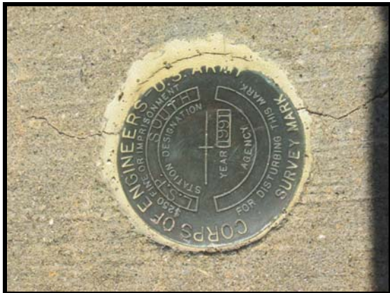
Fig 8: USACE bench mark KV6856 and setup overview
