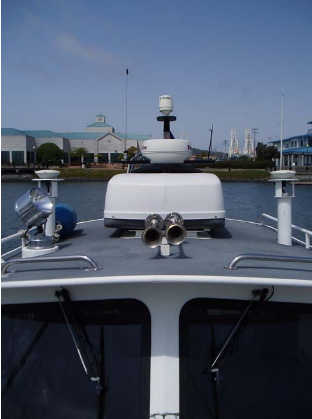
Figure 2: View of top of house on Launch S3003. Center GPS antenna is used by Trimble DSM 132 receiver, and two lower antennae are used by the POS/MV.
