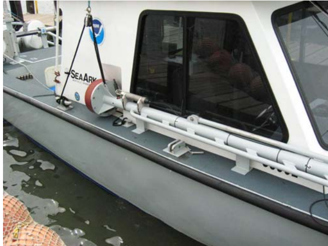
Figure 2: Pole-mounted Simrad EM3000
