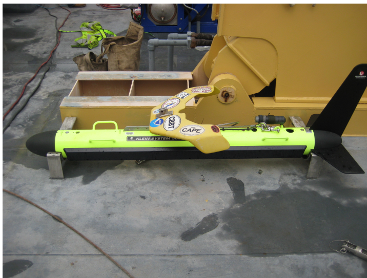
Figure : Klien 5000 V2 configured for towing
