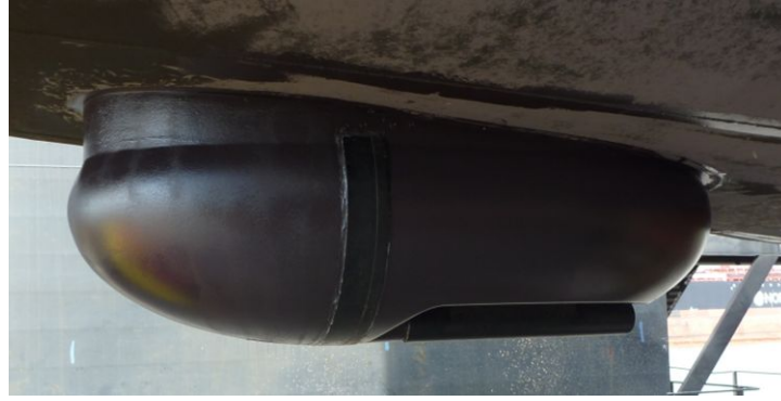
Figure : 7111 mount and fairing. Sonar is located forward on the starboard hull.
