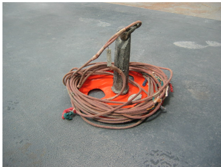
Figure : Leadline fitted with custom mud-shoe to limit penetration of soft bottoms.
