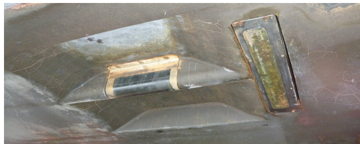
Figure : 7125 Housing flush mounted on hull
