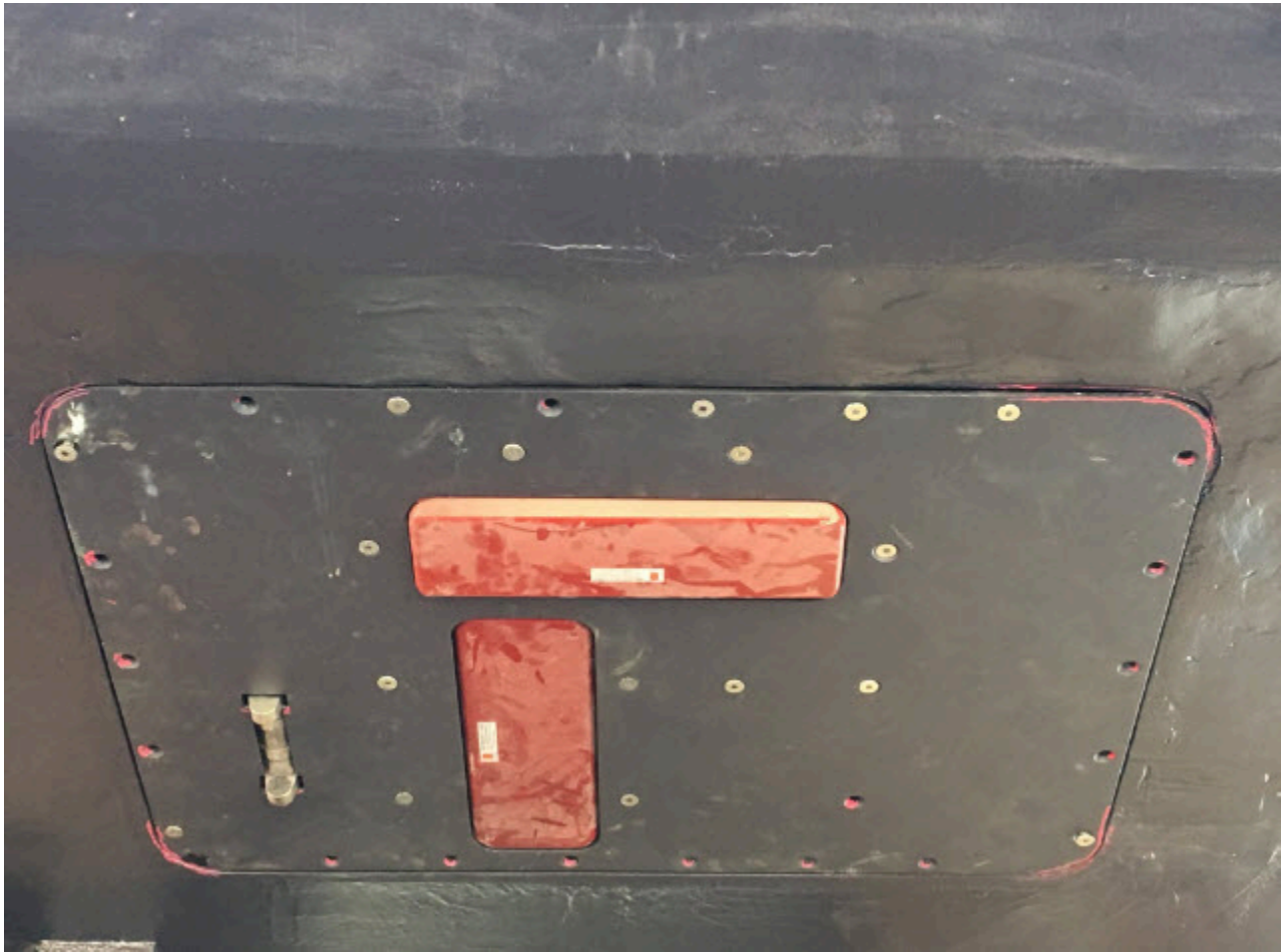
Figure 6: EM 2040 gondola installed in one hull of S250.
