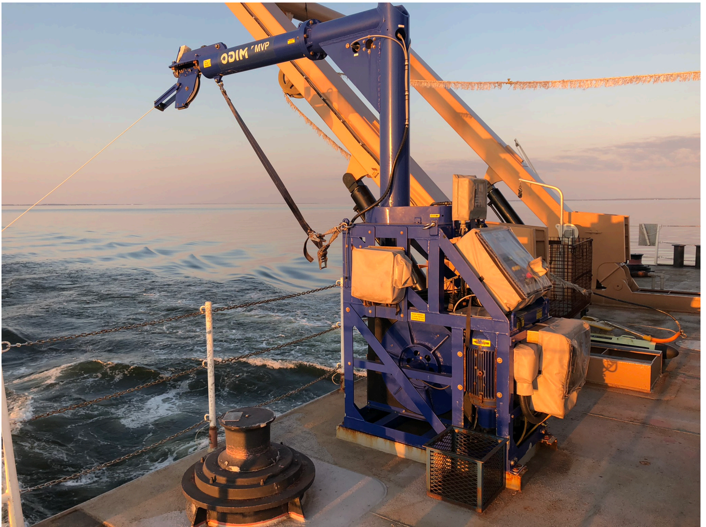
Figure 15: Moving Vessel Profiler on the starboard water of the ship
