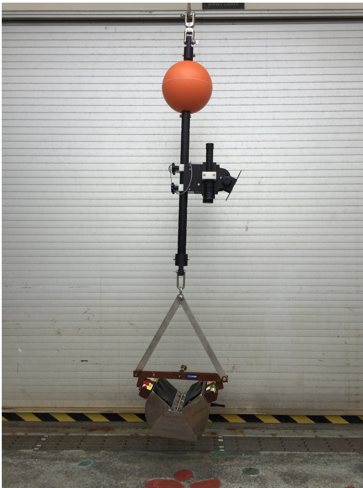
Figure 20: Camera with custom mount allowing for high quality video of the seafloor.
