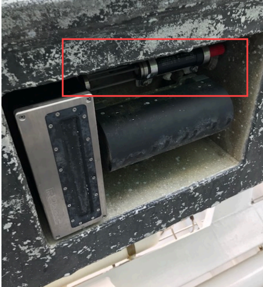
Figure 18: Valport Mini SVP sensor mounted locally near R2 Sonic transducer and receiver on board launch 2702
