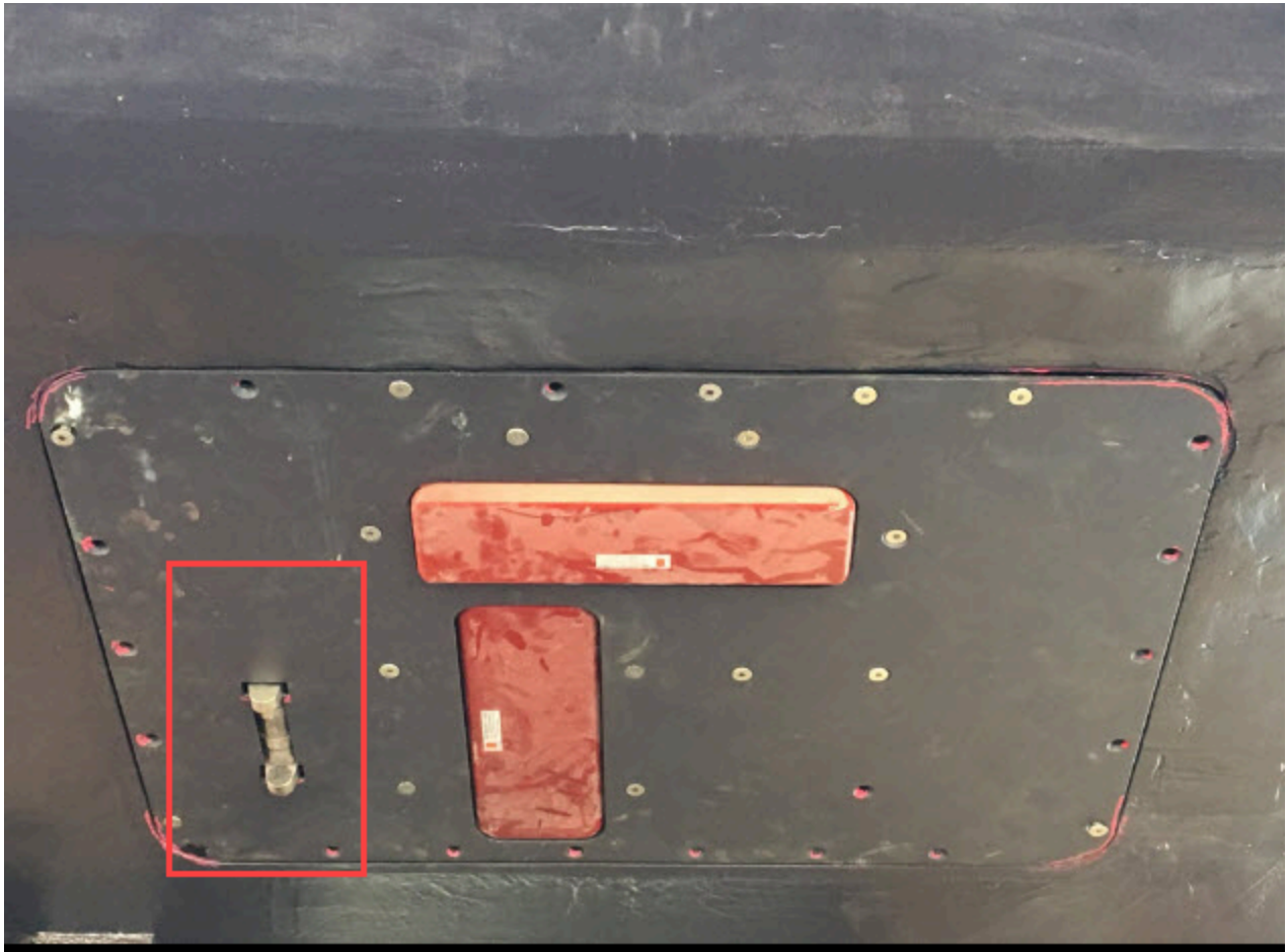
Figure 17: SVP-70 mounted locally at the 2040 transducer and receiver.
