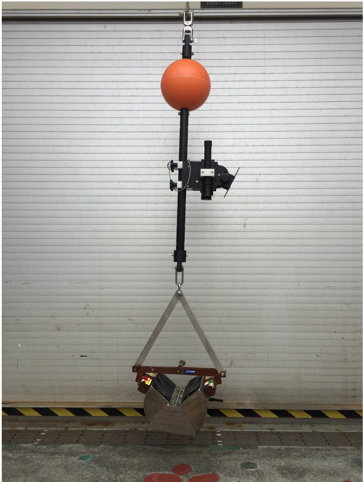
Figure 6: Camera with custom mount allowing for high quality video of the seafloor.
