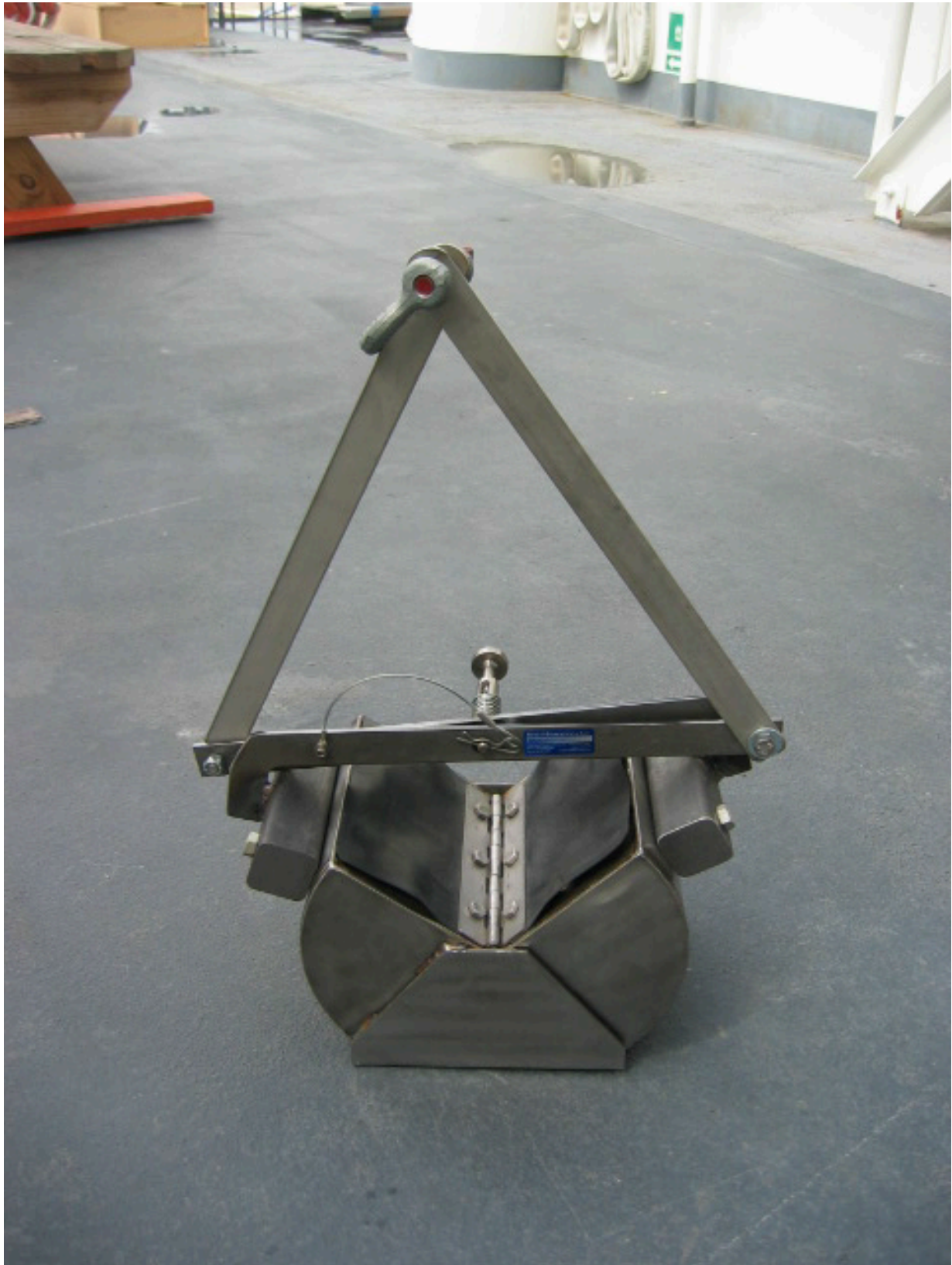
Figure 5: Ponar grab sampler.
