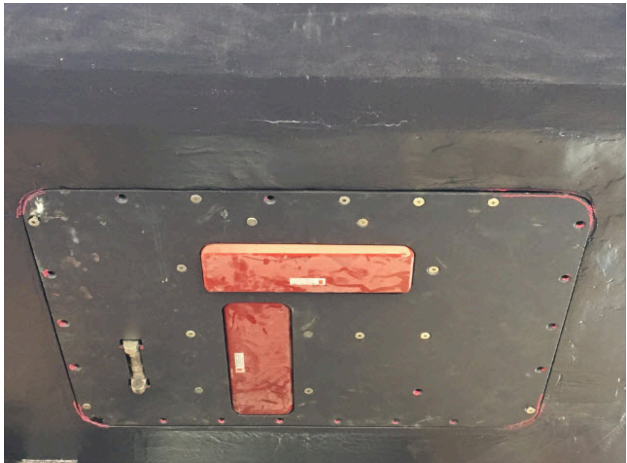
Figure 4: EM 2040 gondola installed in one hull of S250.
