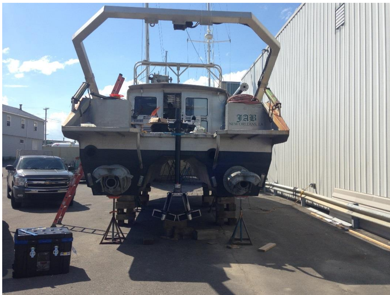
Figure 22 R/V JAB Dual 7125 with Underwater IMU
