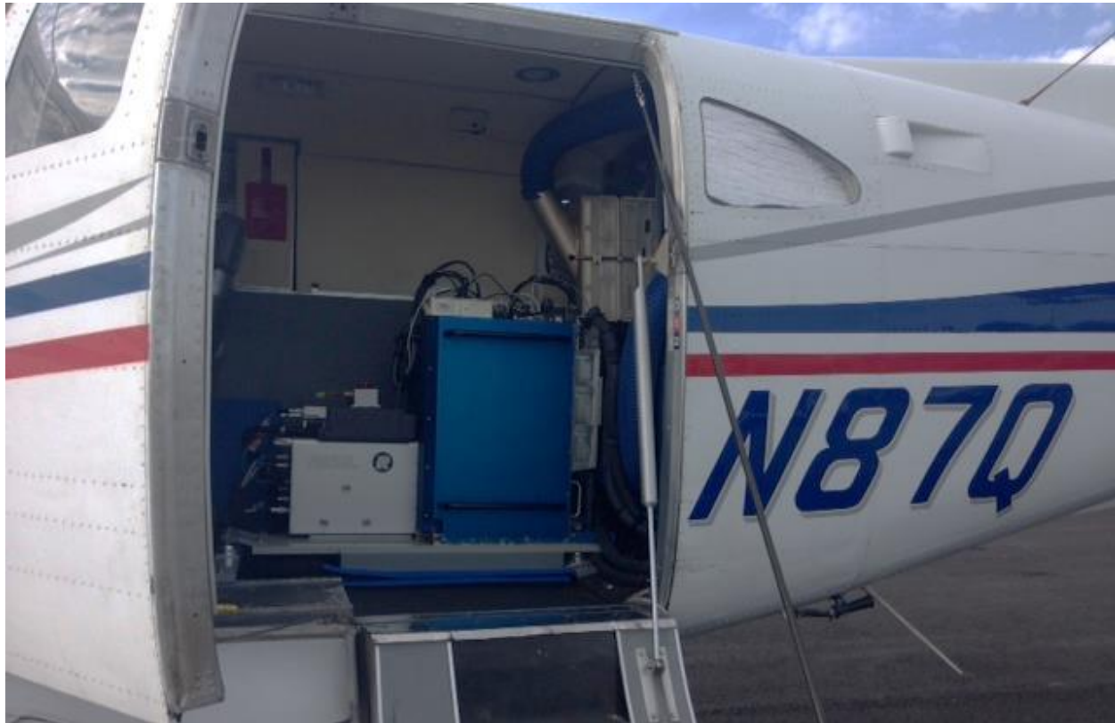
Figure 30 SHOALS and RIEGL 820 Installation in N87Q
