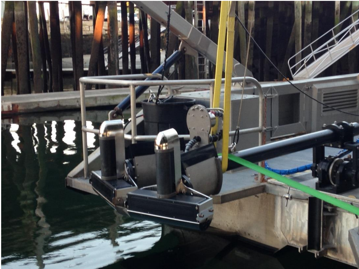
Figure 25 R/V Westerly Dual 7125 with Underwater IMU
