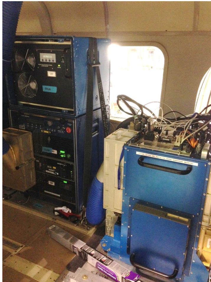
Figure 28 SHOALS-1000T modules. Equipment rack (left); sensor housing (right)
