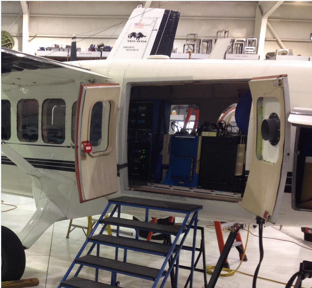
Figure 29 SHOALS Installation in DC-6 Twin Otter
