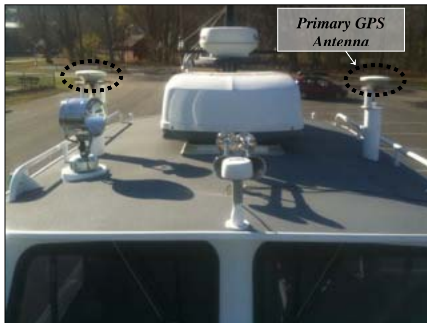
Figure 2: POS/MV Antenna Installation
