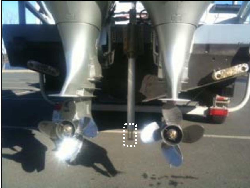
Figure 4: Surface Sound Speed Digibar Installation
