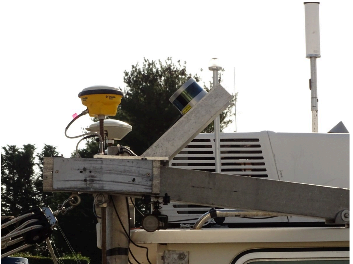
Figure 7: Velodyne VLP-16 LiDAR mounted on the RV Able 2.
