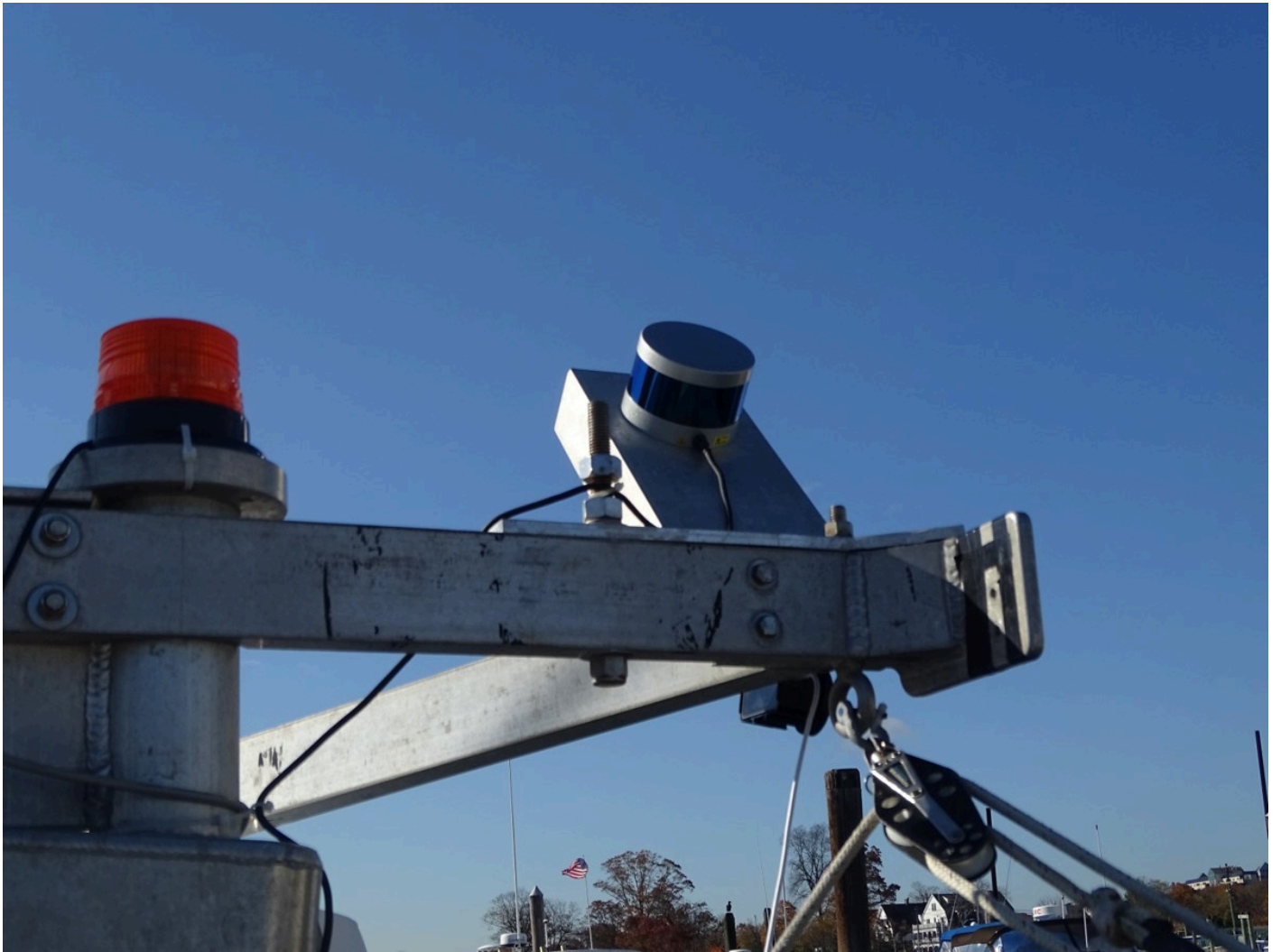
Figure 8: Velodyne VLP-16 LiDAR mounted on the RV Osprey.
