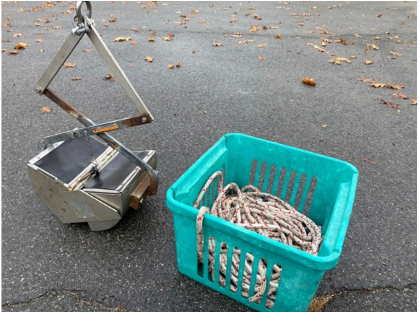
Figure 12: WILDCO Ponar Dredge Bottom Sampler used on the RV Osprey
