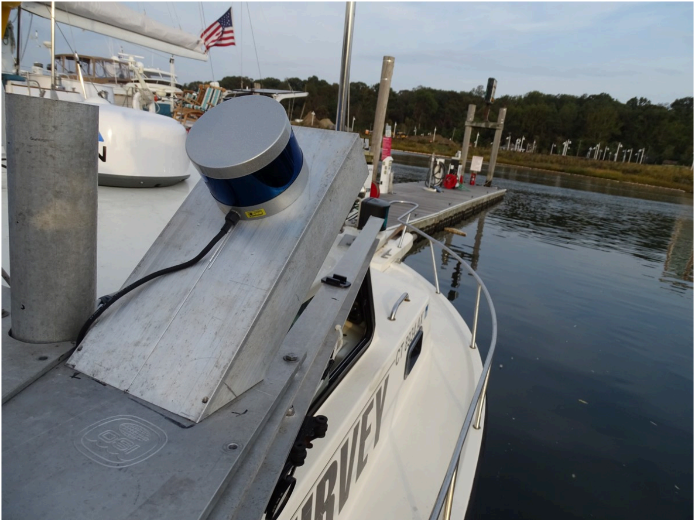
Figure 9: Velodyne VLP-16 LiDAR mounted on the RV Ready 2.
