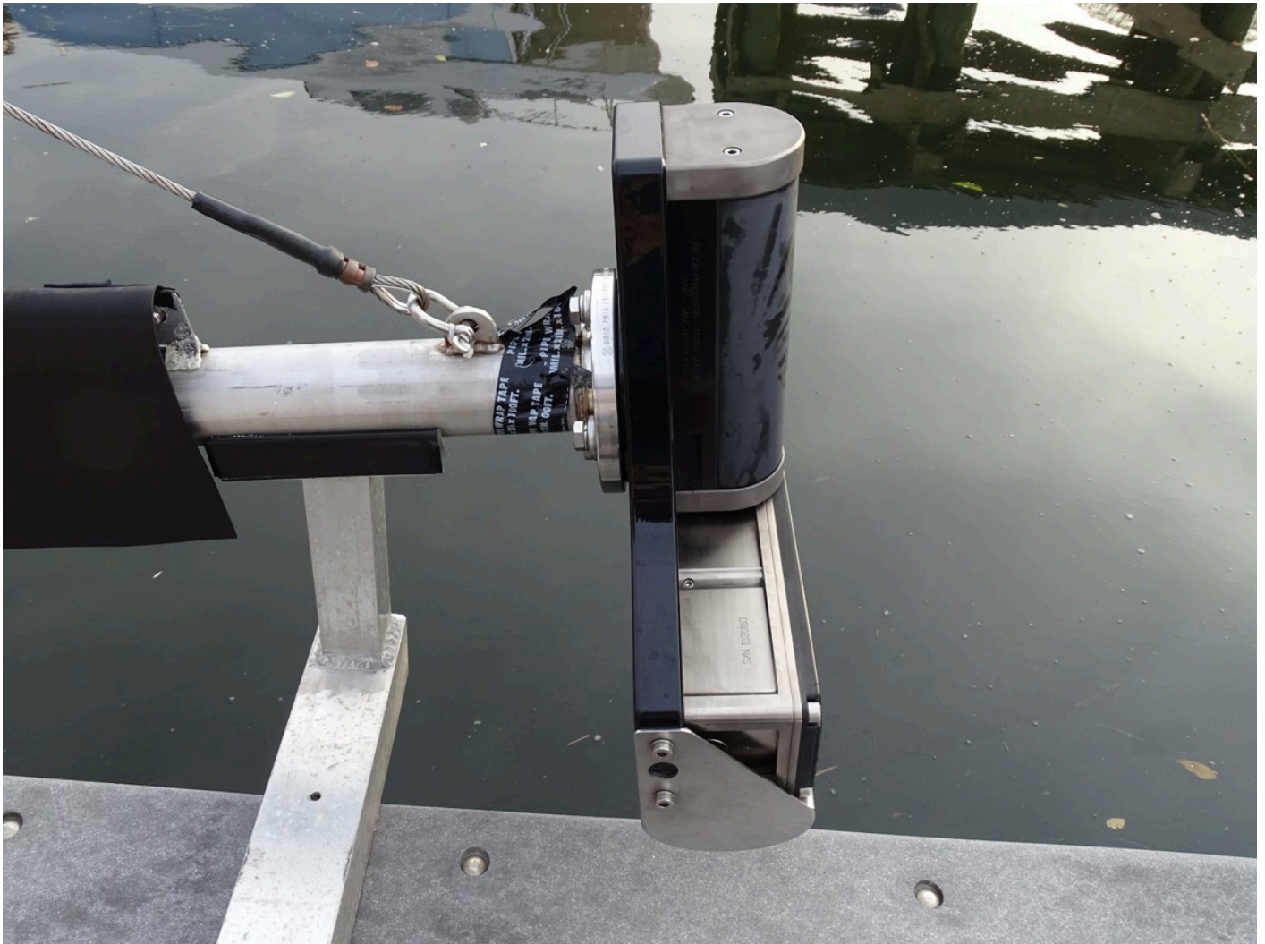
Figure 6: SeaBat T50-R transducer mounted on the RV Ready 2 transducer pole.
