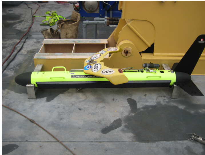
Figure : Klien 5000 V2 configured for towing
