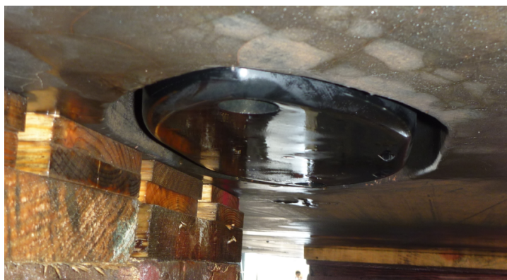
Figure : Hull mounted Odom Vertical Beam Echosounder
