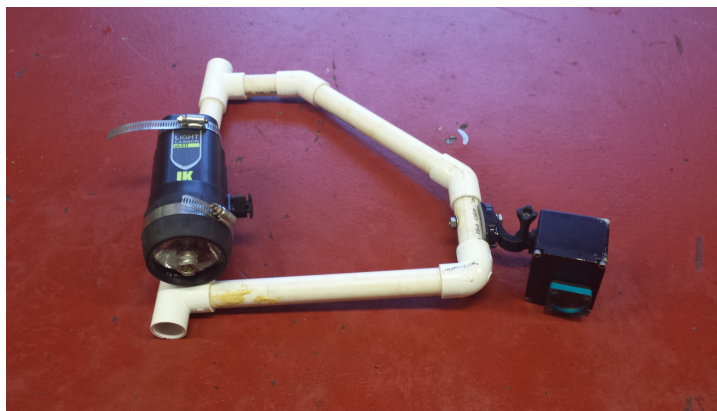
Figure : Camera with custom mount allowing for high quality video of the seafloor
