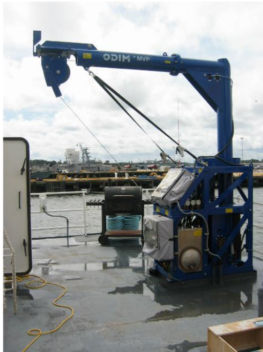
Figure : MVP control station & winch
