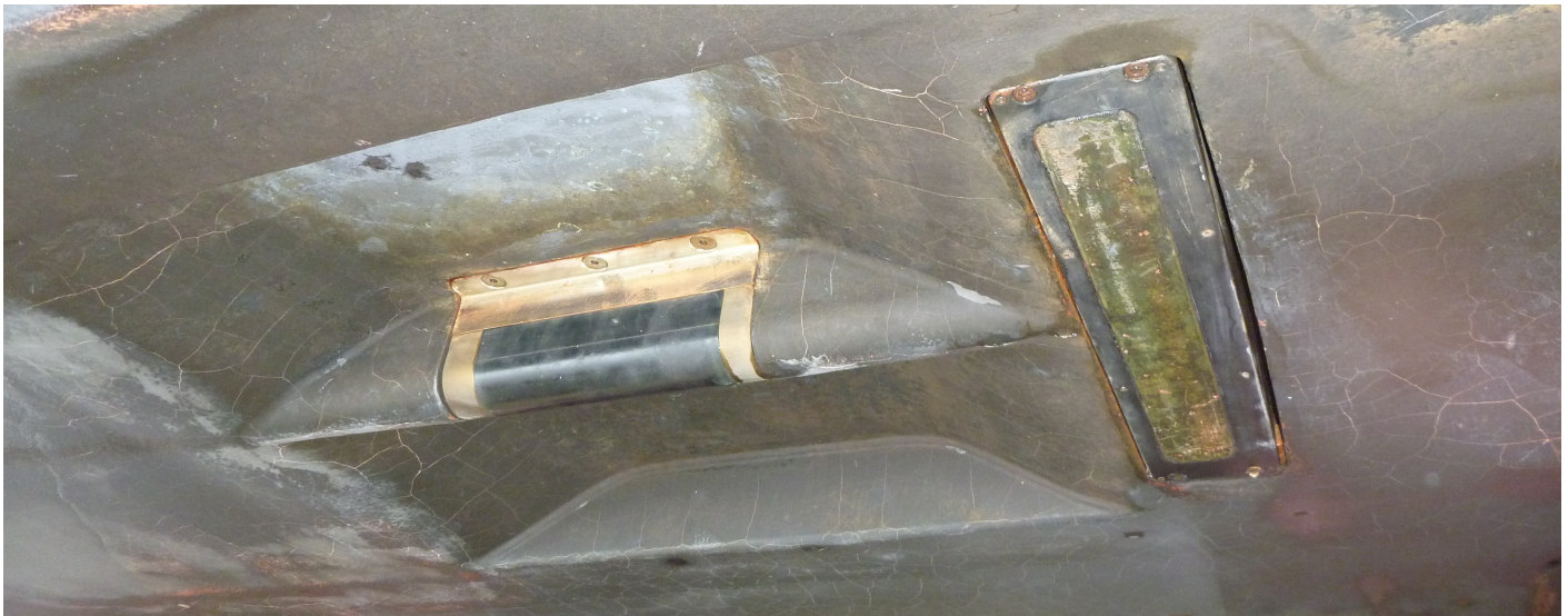
Figure 3: 7125 Housing flush-mounted on hull.
