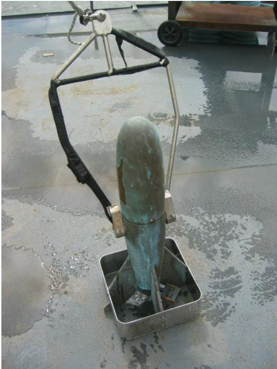
Figure 12: MVP single sensor free fall fish.
