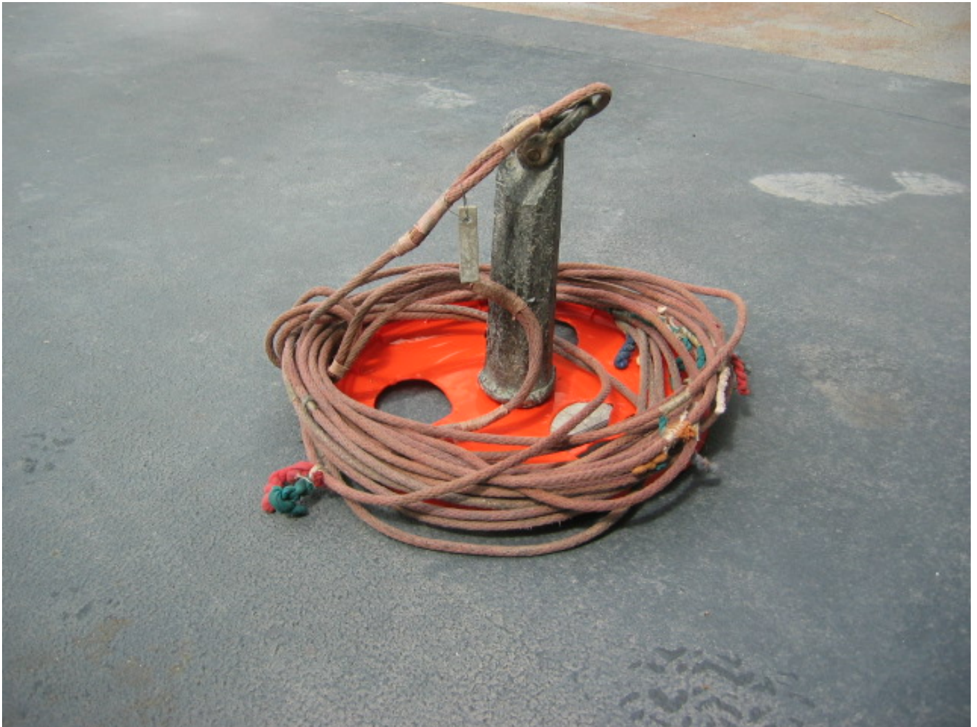
Figure 8: Leadline fitted with custom mud-shoe to limit penetration of soft bottoms.
