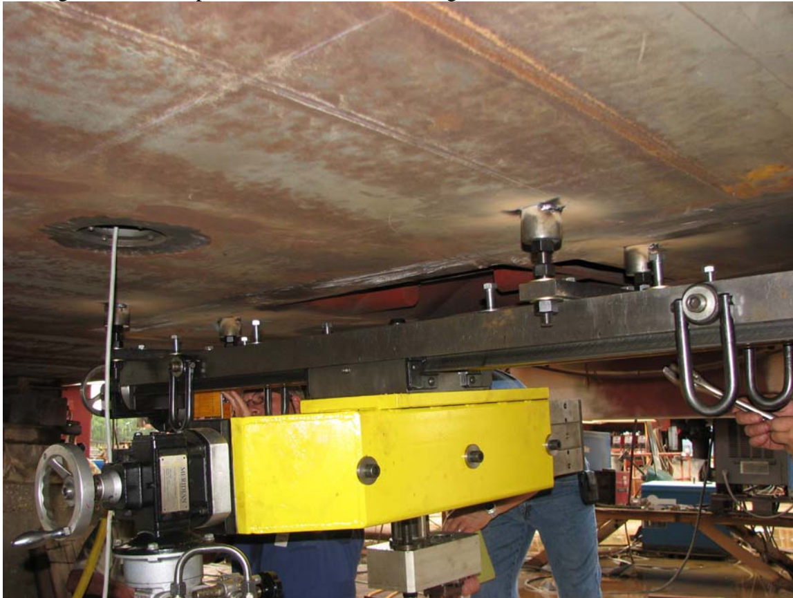
Milling machine set up on 7125 transducer housing
