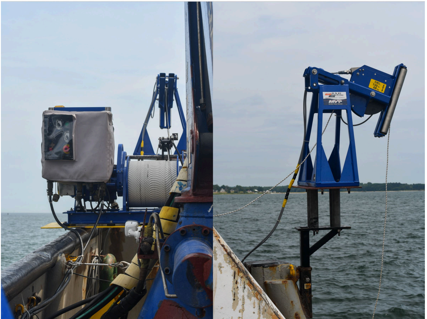
Figure 11: MVP30-350 Moving Vessel Profiler mounted on the starboard quarter of the MV Northstar Challenger.
