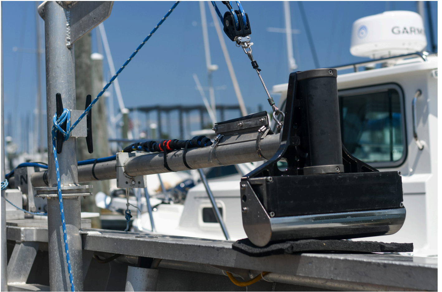
Figure 5: SeaBat T50-R transducer mounted on the RV North Cove transducer pole.
