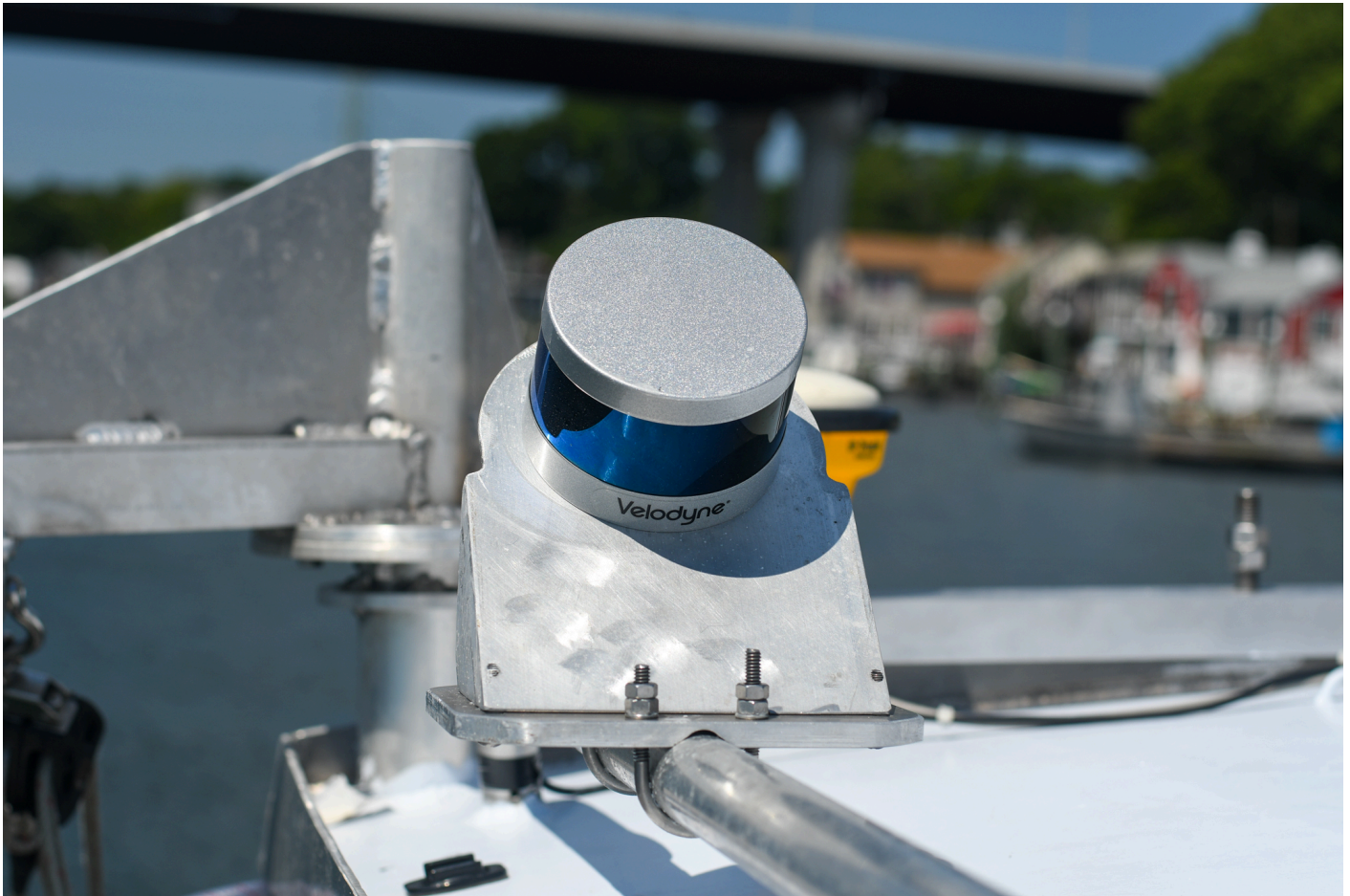
Figure 8: Velodyne VLP-16 LiDAR mounted on the RV South Cove.
