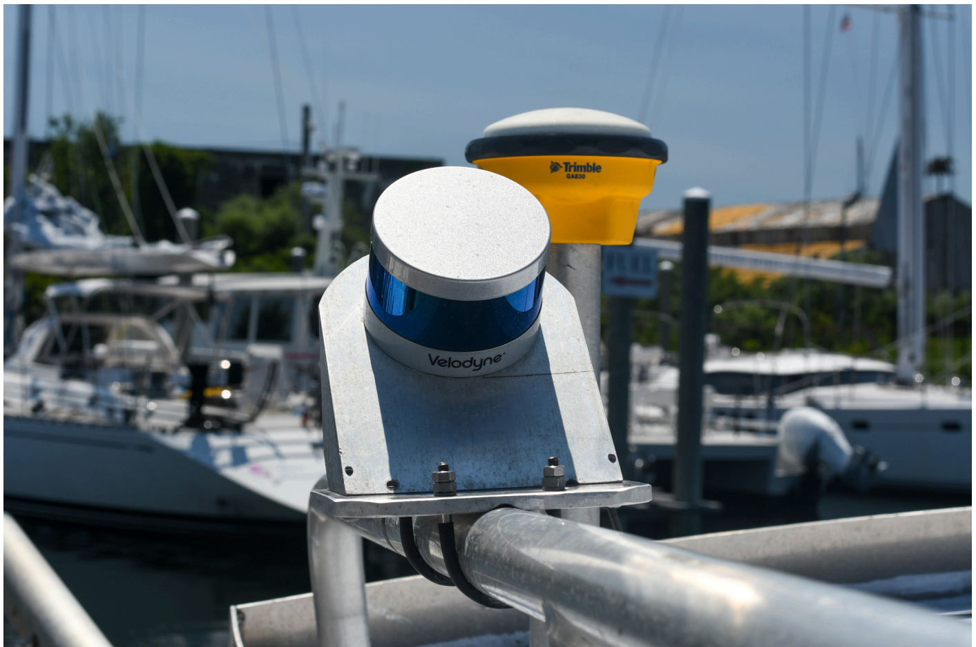
Figure 7: Velodyne VLP-16 LiDAR mounted on the RV North Cove.
