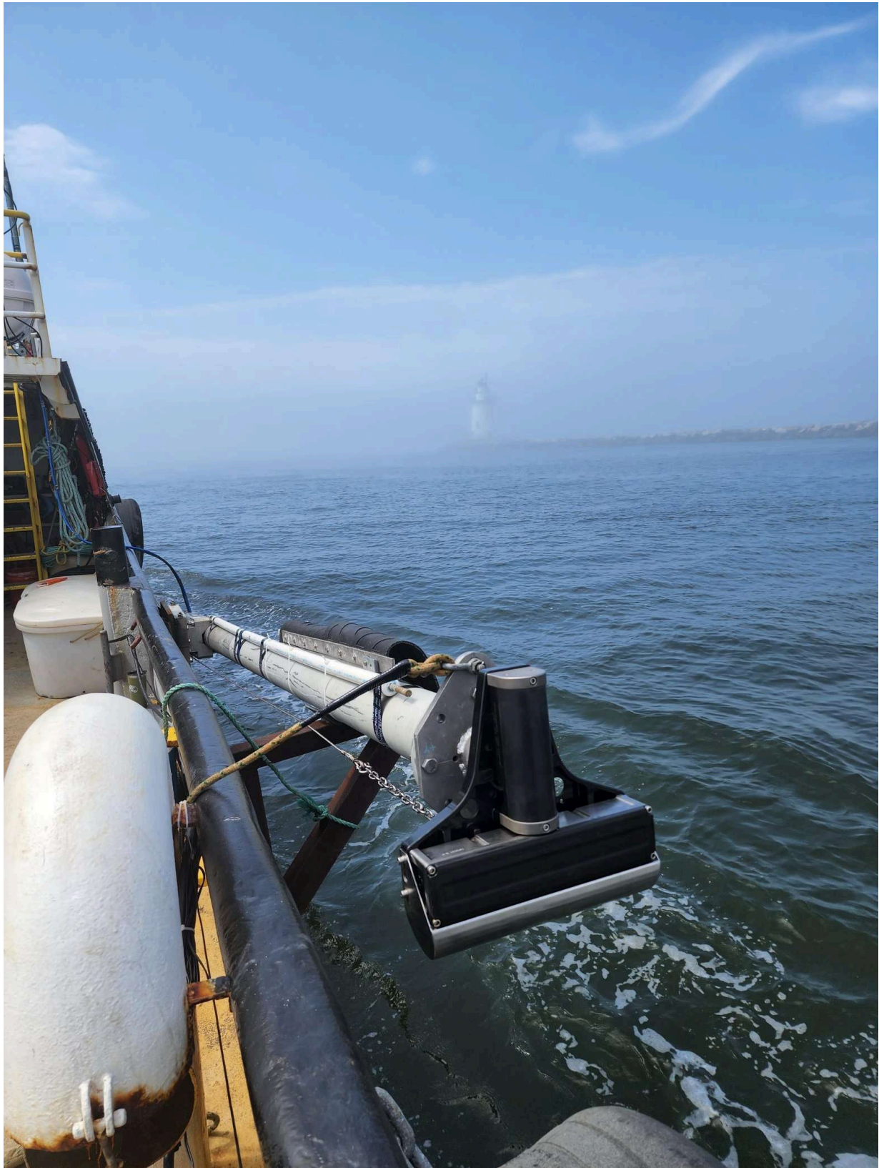
Figure 4: SeaBat T50-R transducer mounted on the MV Northstar Challenger transducer pole.
