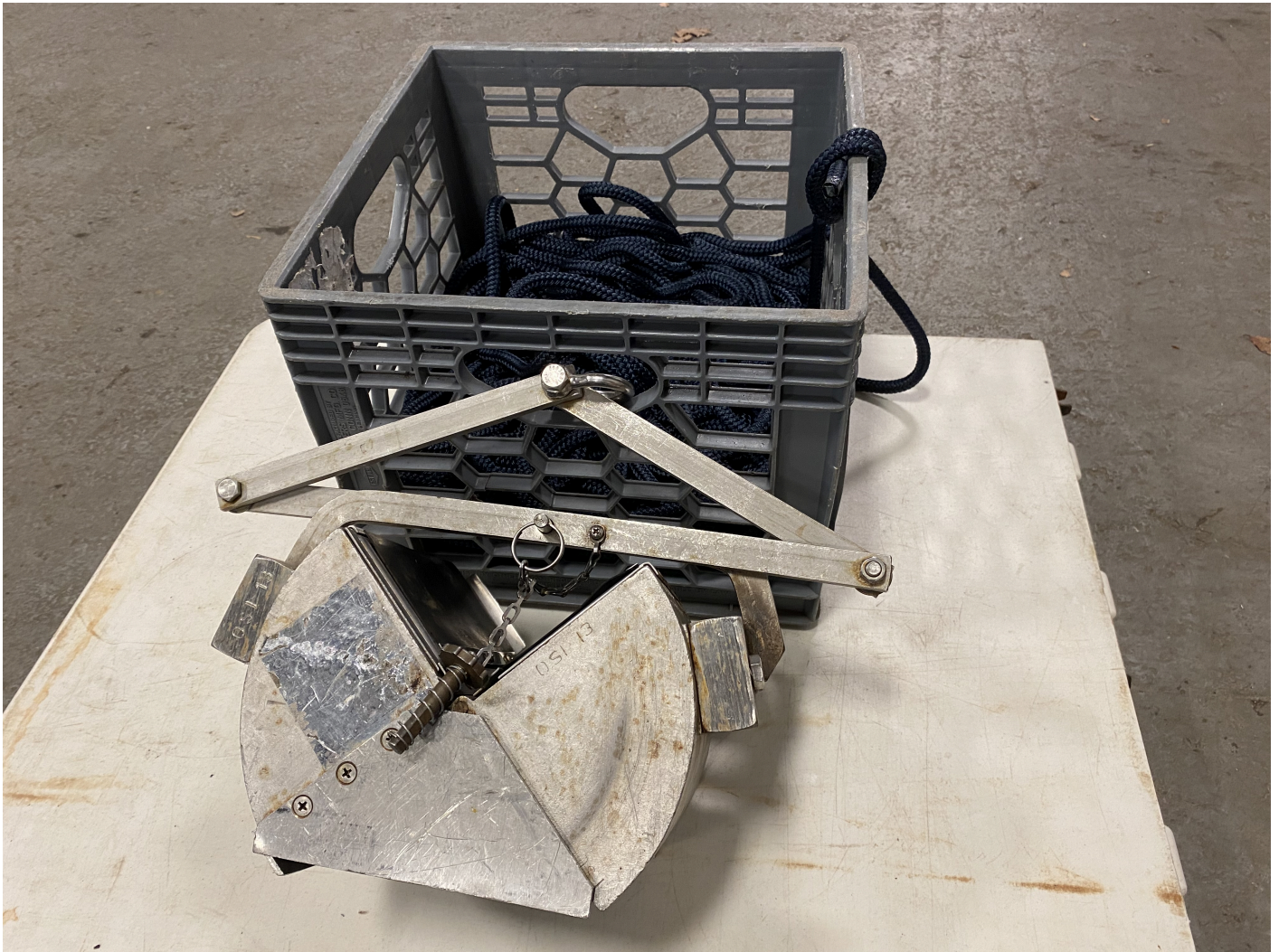
Figure 12: WILDCO Petite Ponar Dredge Bottom Sampler used on the RV North Cove and RV South Cove.
