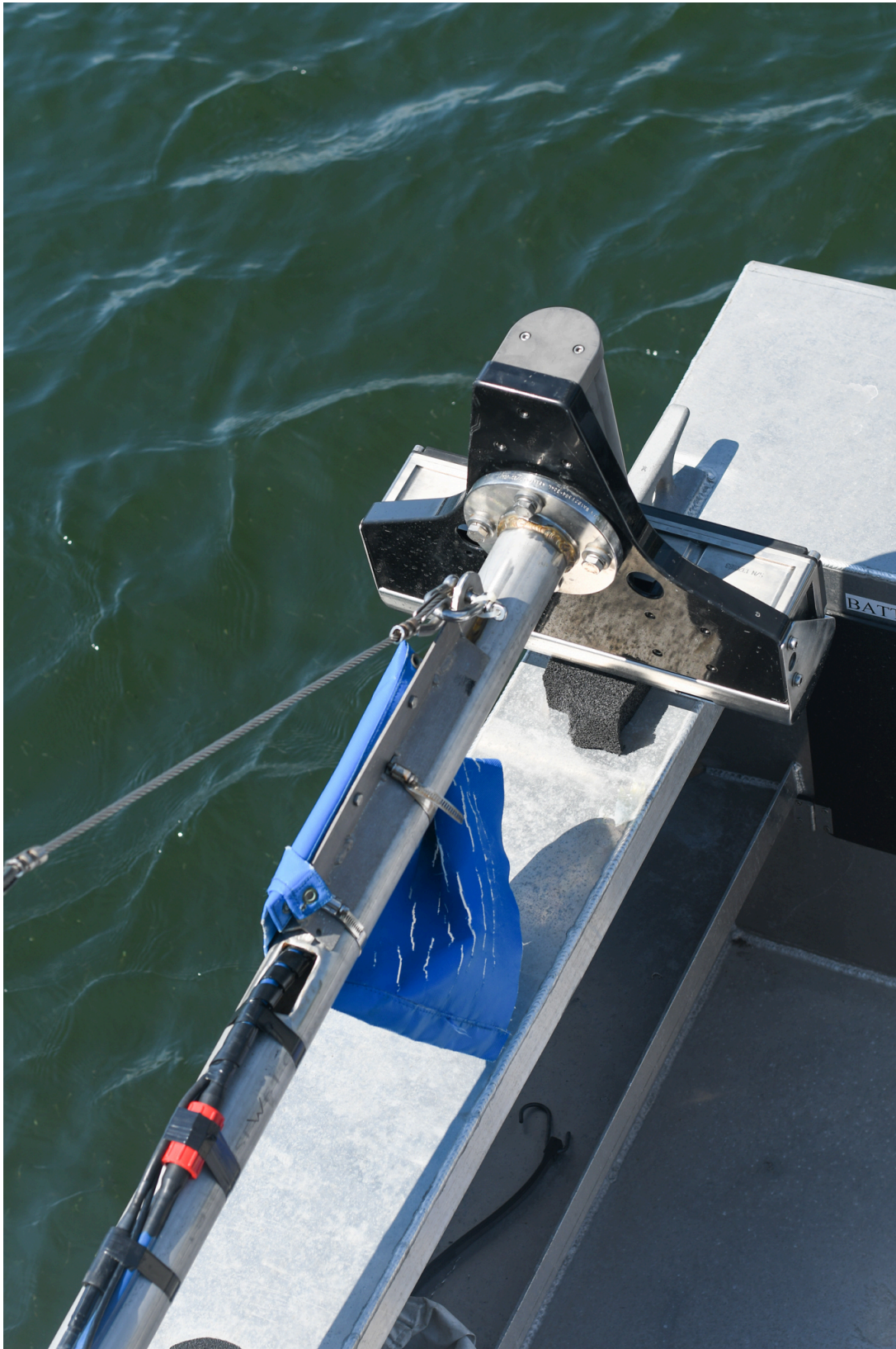
Figure 6: SeaBat T50-R transducer mounted on the RV South Cove transducer pole.
