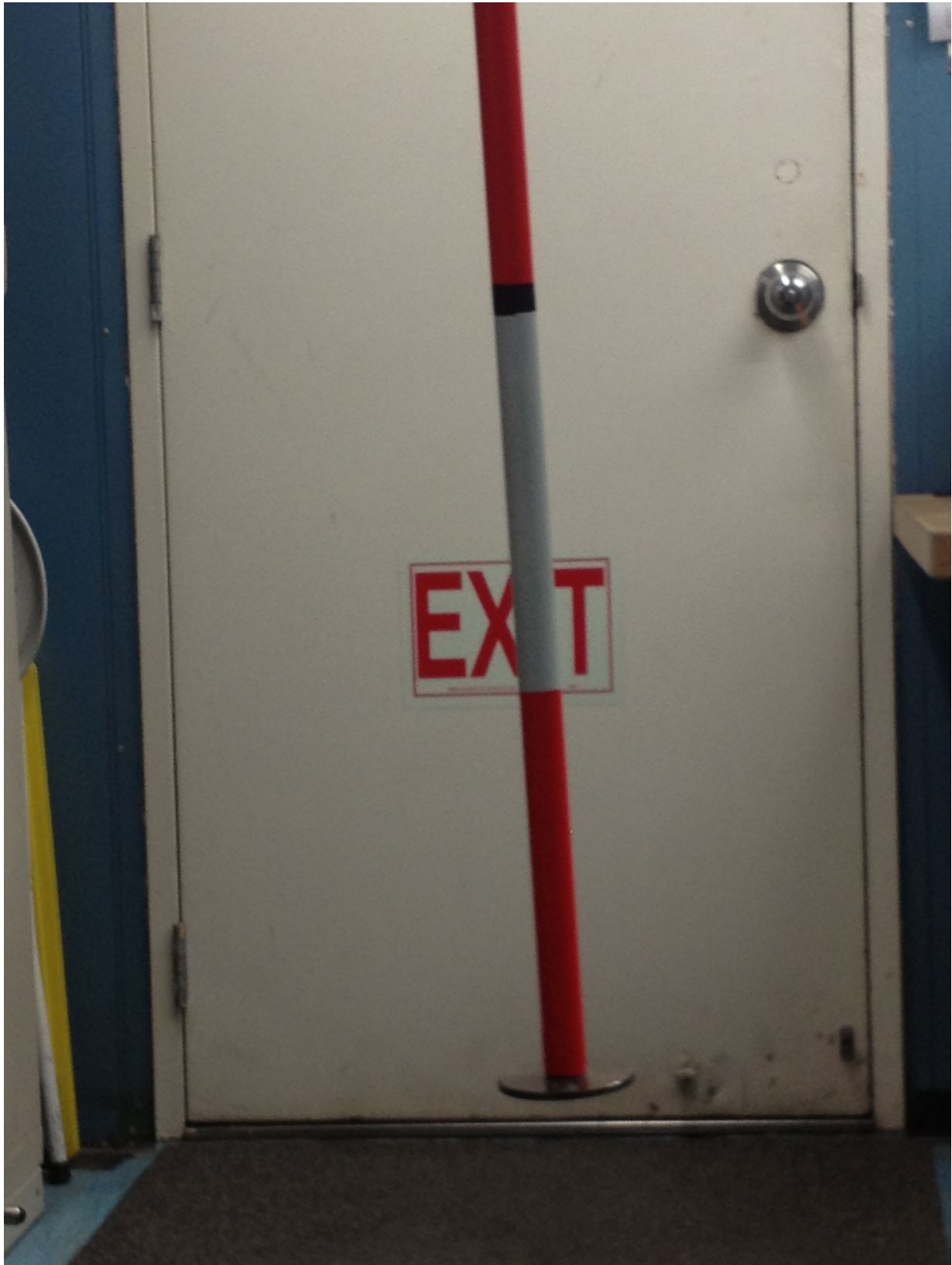
Figure : Sounding pole used aboard Thomas Jefferson and her survey launches.
