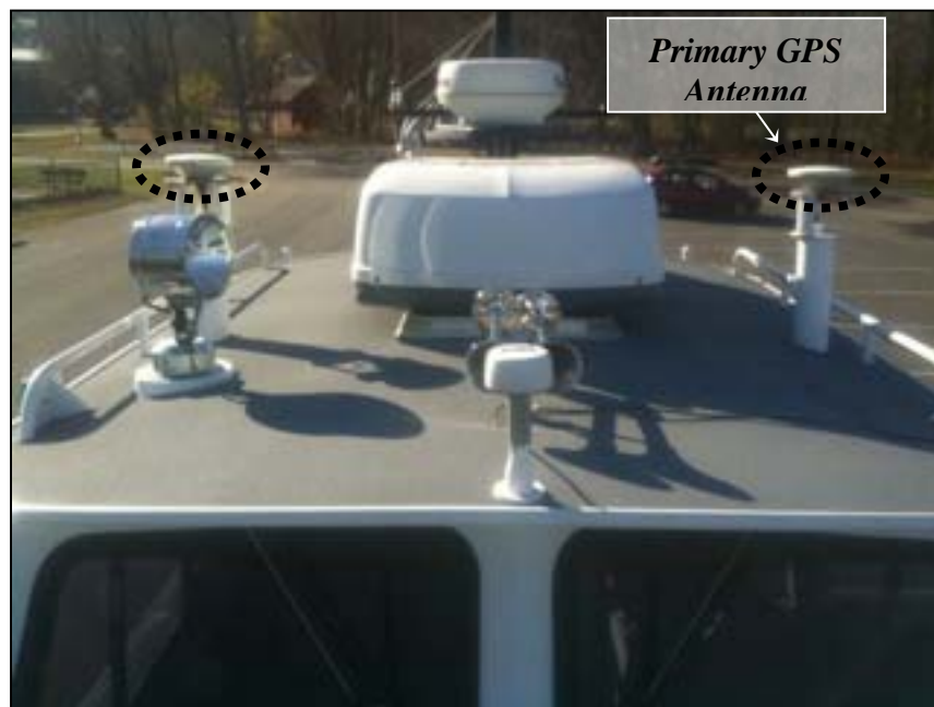
Figure 2: POS/MV Antenna Installation
