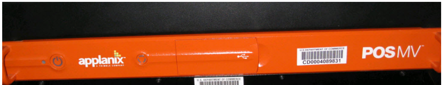
Figure 7: POS/MV computing system unit (orange) rack mounted aboard R/V BAY HYDRO II.
