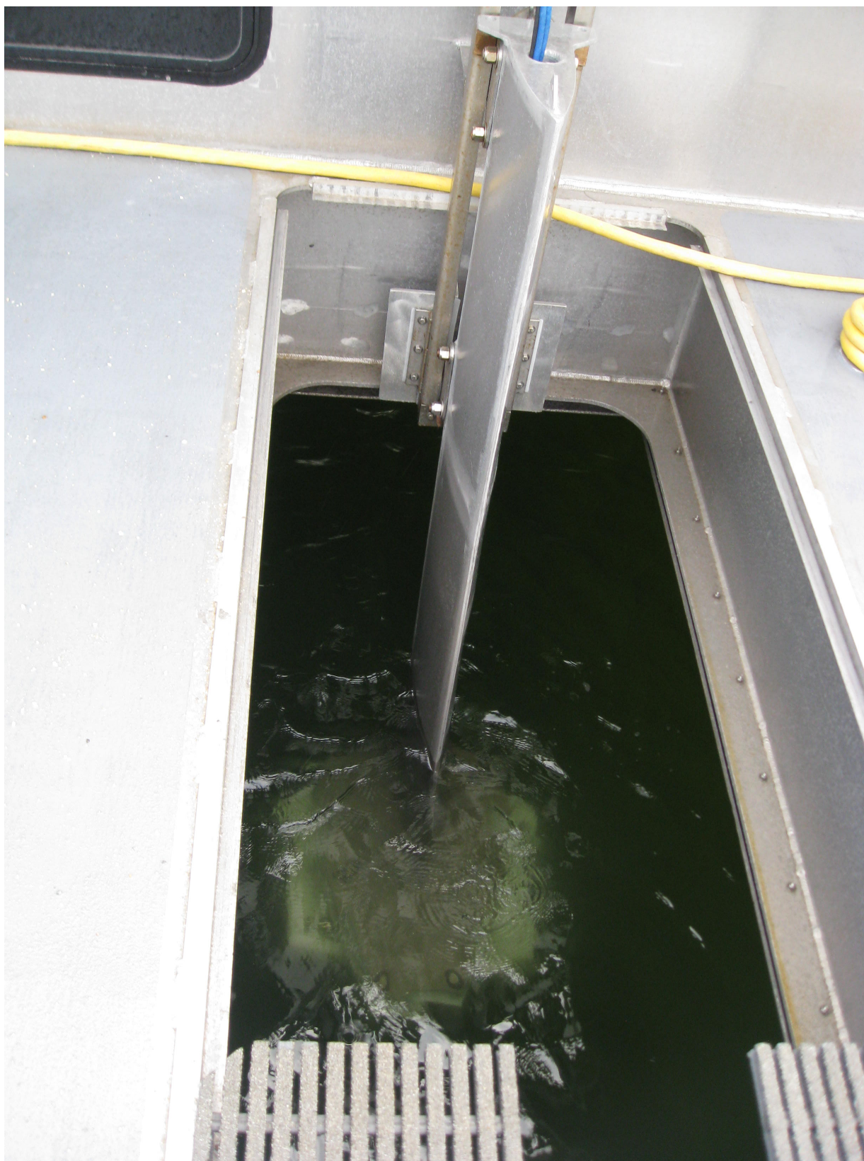
Figure 4: Kongsberg EM2040 housing and sonar in the deployed position.
