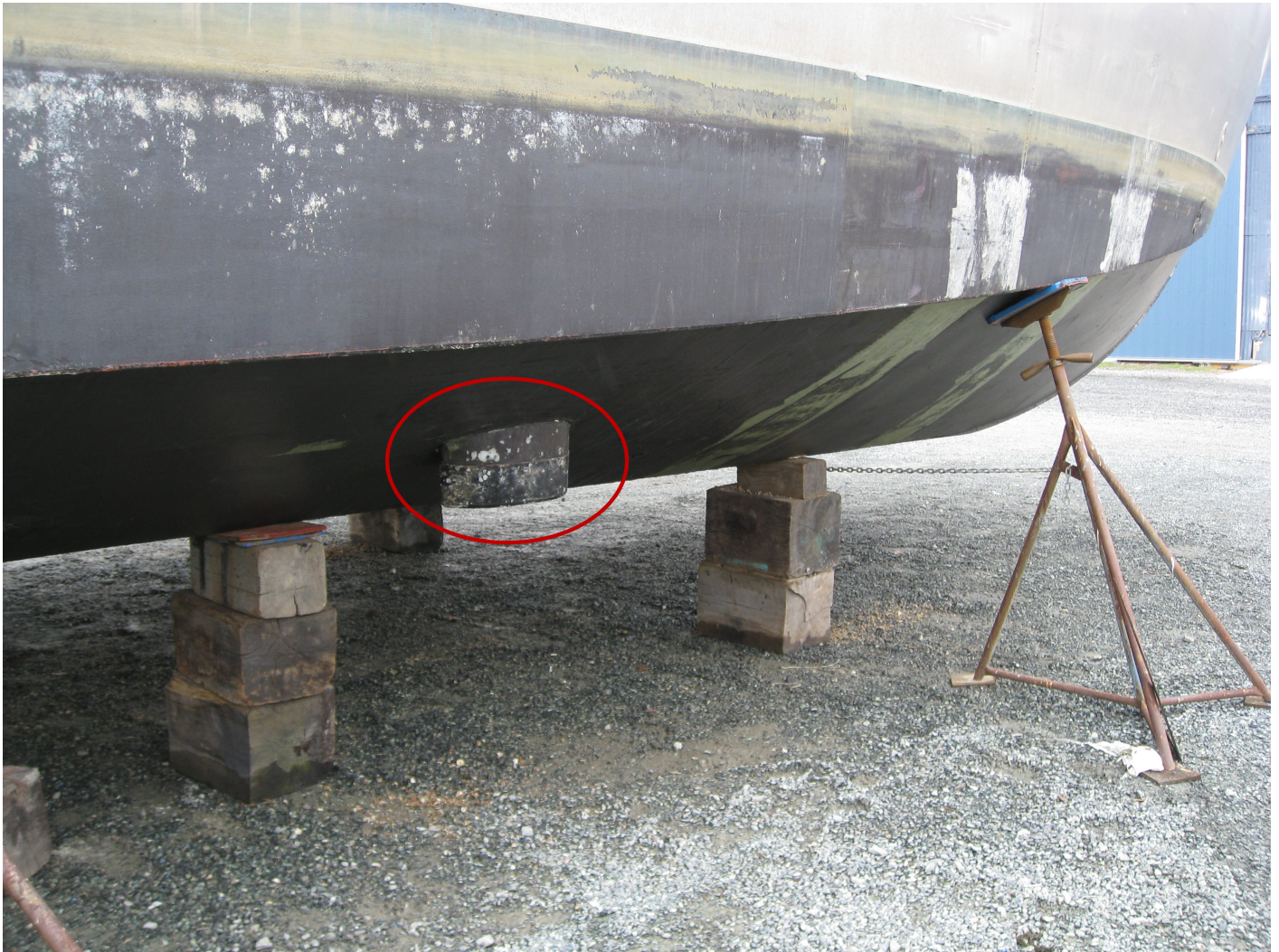
Figure 5: R/V Bay Hydro II's SBES sonar mounted outboard on the starboard hull.
