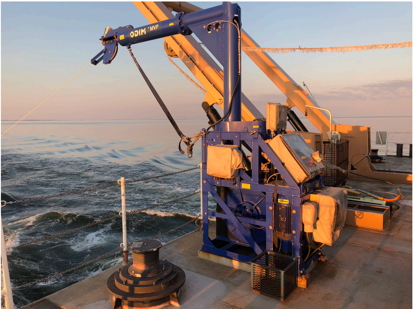
Figure 12: Moving Vessel Profiler on the starboard water of the ship
