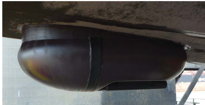
Figure 5: 7111 mount and fairing. Sonar is located forward on starboard hull.
