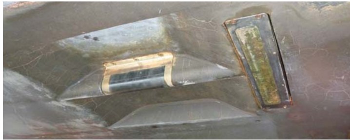
Figure 4: 7125 Housing flush mounted on hull
