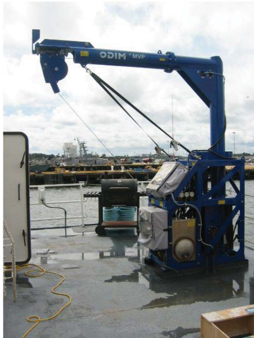
Figure 9: MVP control station & winch
