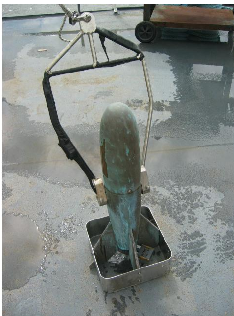
Figure 20: MVP single sensor free fall fish.
