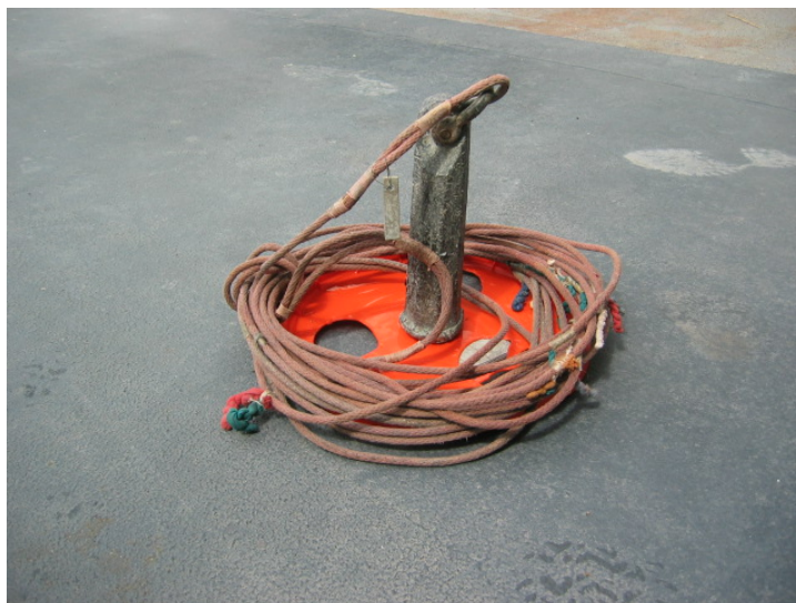
Figure 17: Leadline fitted with custom mud-shoe to limit penetration of soft bottoms.
