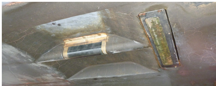
Figure 4: 7125 Housing flush mounted on hull
