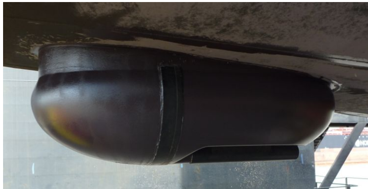
Figure 13: 7111 mount and fairing. Sonar is located forward on the starboard hull.
