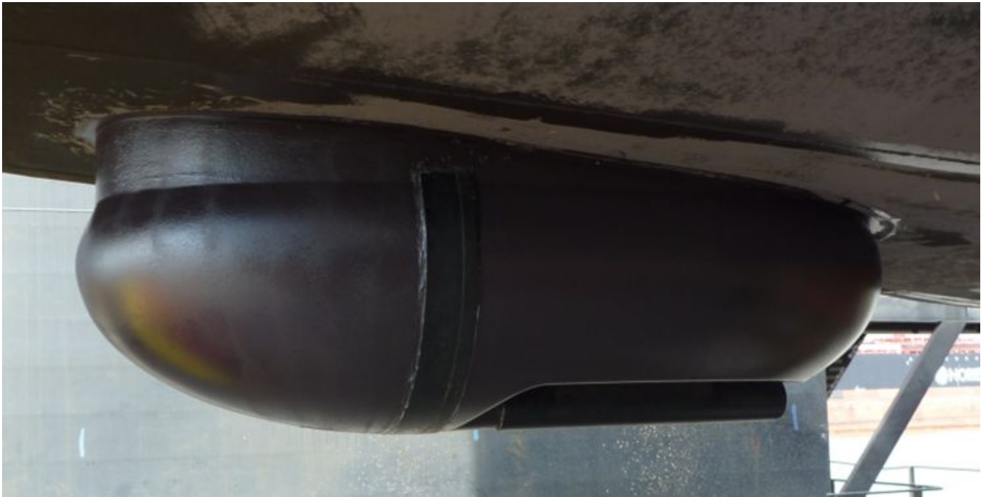
Figure 11: 7111 mount and fairing. Sonar is located forward on the starboard hull.
