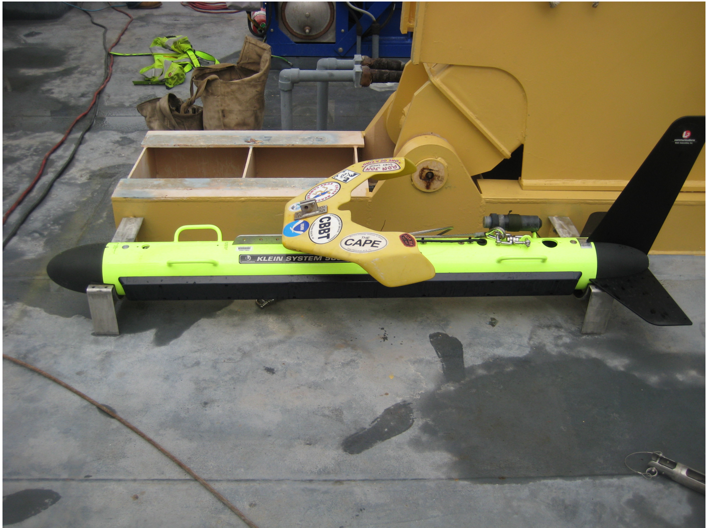
Figure 3: Klein 5000 V2 configured for towing
