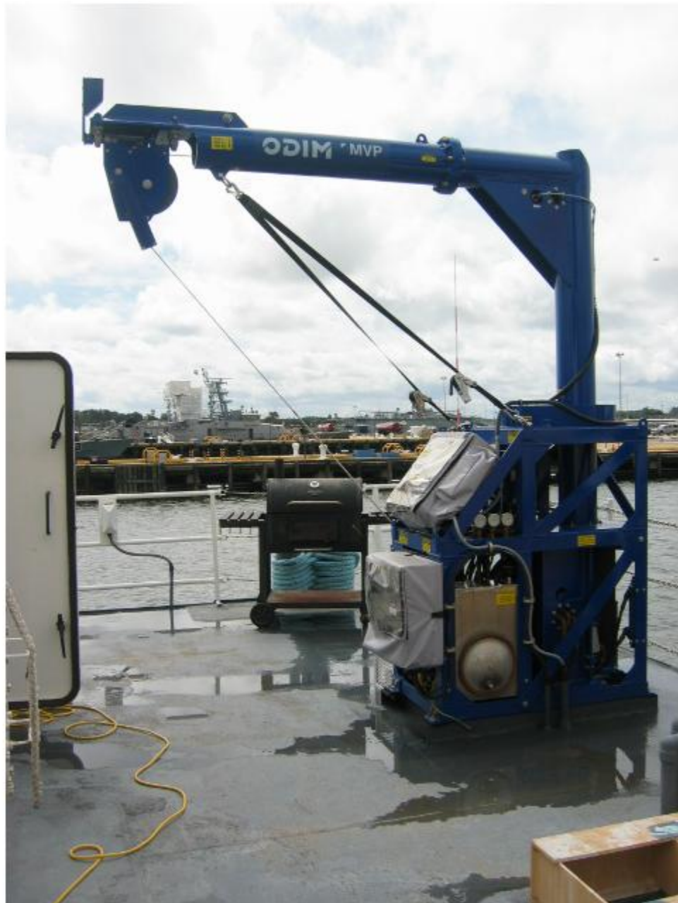
Figure 19: MVP control station & winch
