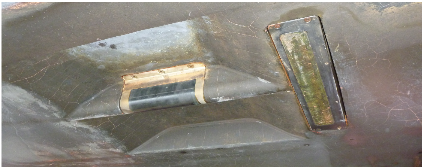
Figure 4: 7125 Housing flush mounted on hull
