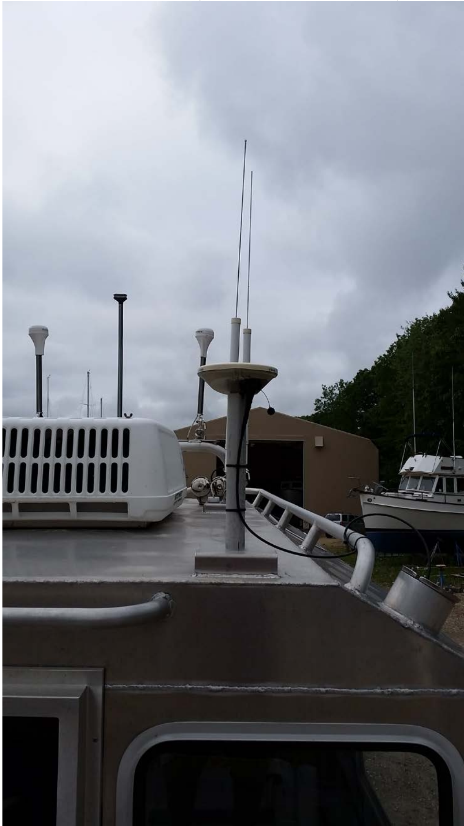
STARBOARD GPS ARP (BOTTOM OF ANTENNA)
