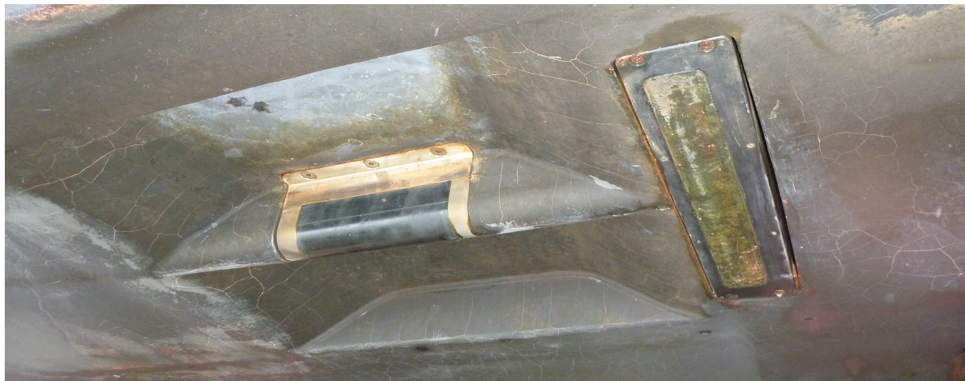
Figure 5: 7125 Housing flush-mounted on hull.
