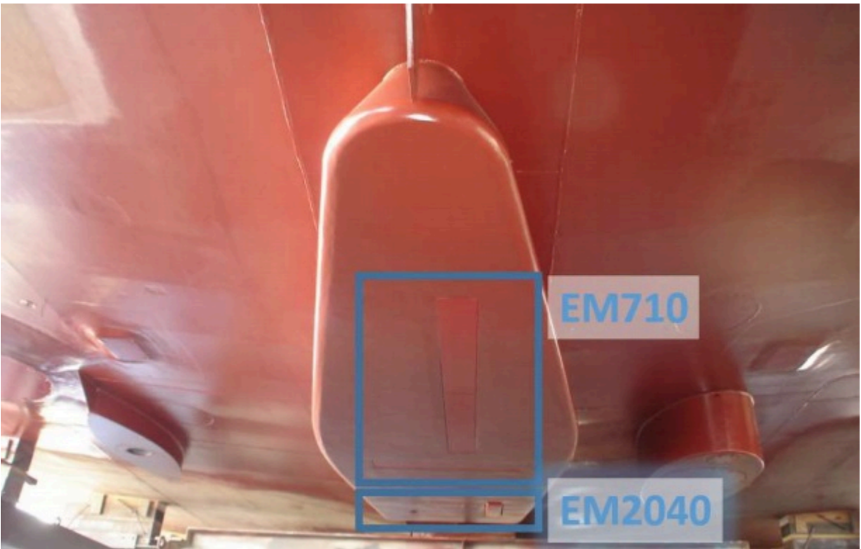
Figure 9: Kongsberg EM2040 and EM710 mounting configuration on S222
