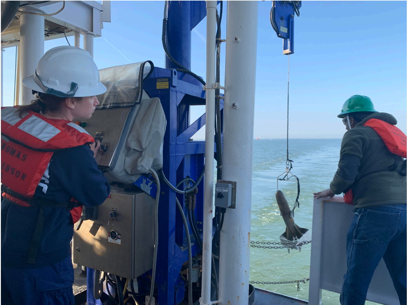
Figure 12: MVP winch and towfish during towfish deployment
