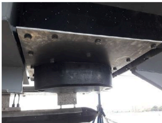
Figure 10: Installation of transducer for Odom Echotrac CV200 on the hull of 2903.
