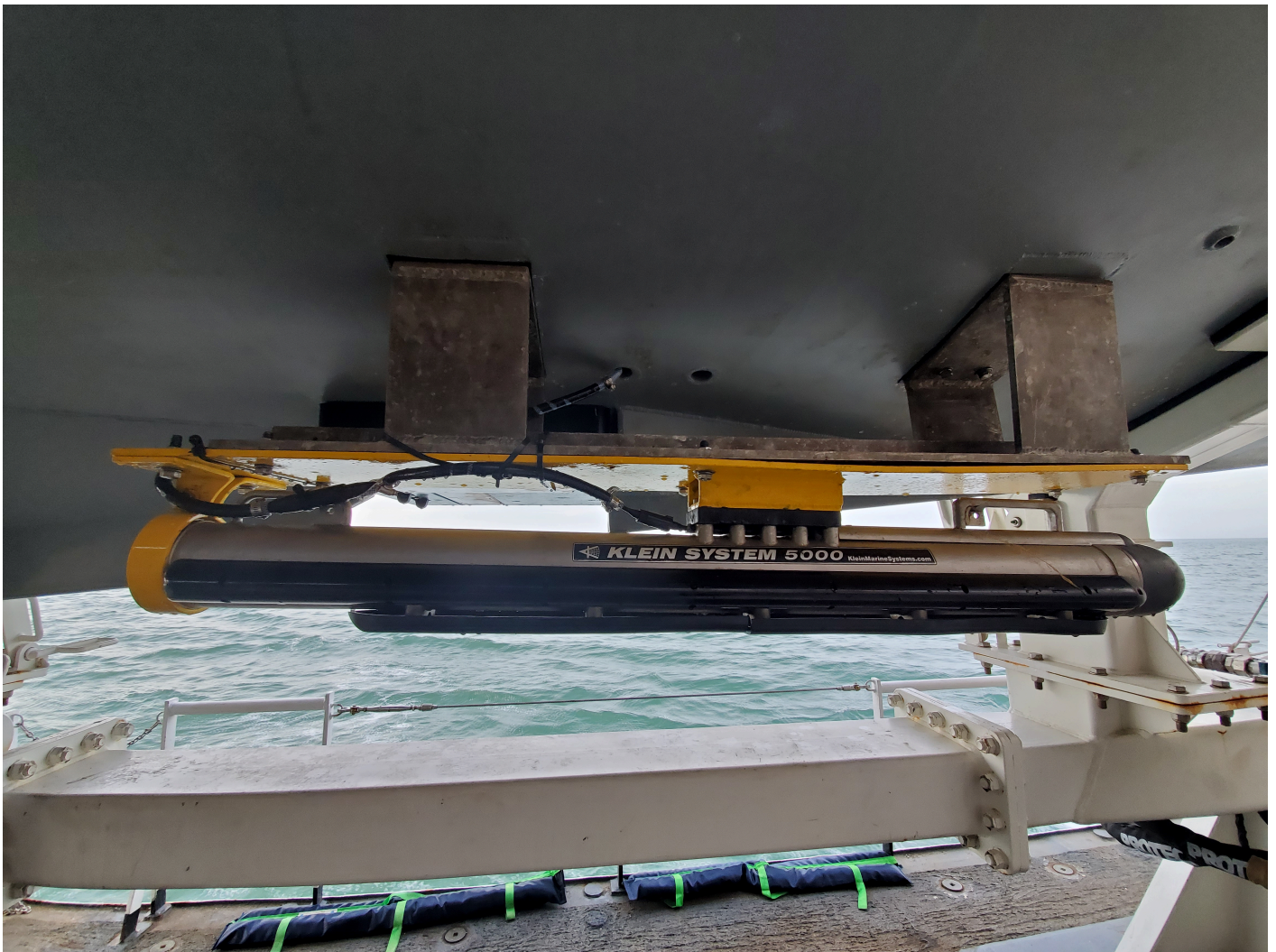
Figure 11: Klein 5000 MKII-B installed on the launch.
