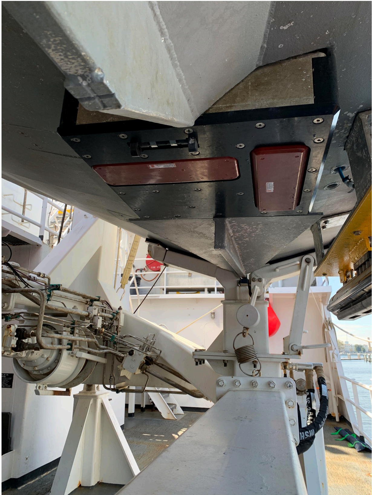
Figure 8: Kongsberg EM2040 mounting configuration on 2903 and 2904
