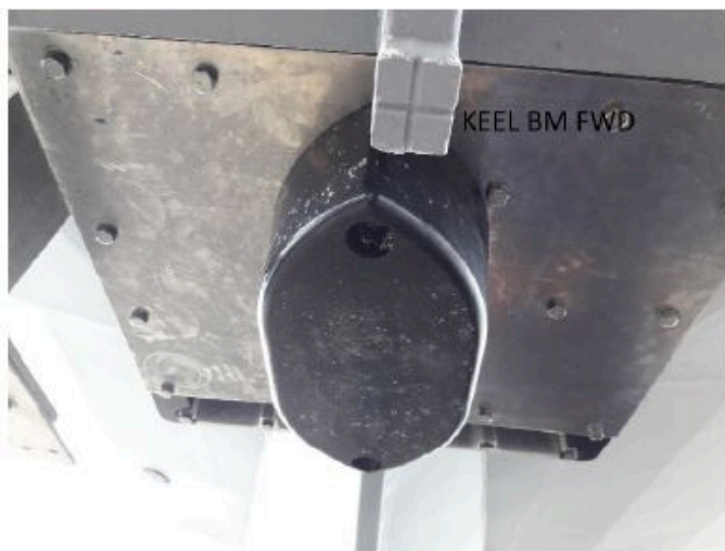
Figure 10: Installation of transducer for Odom Echotrac CV200 on the hull of 2903.
