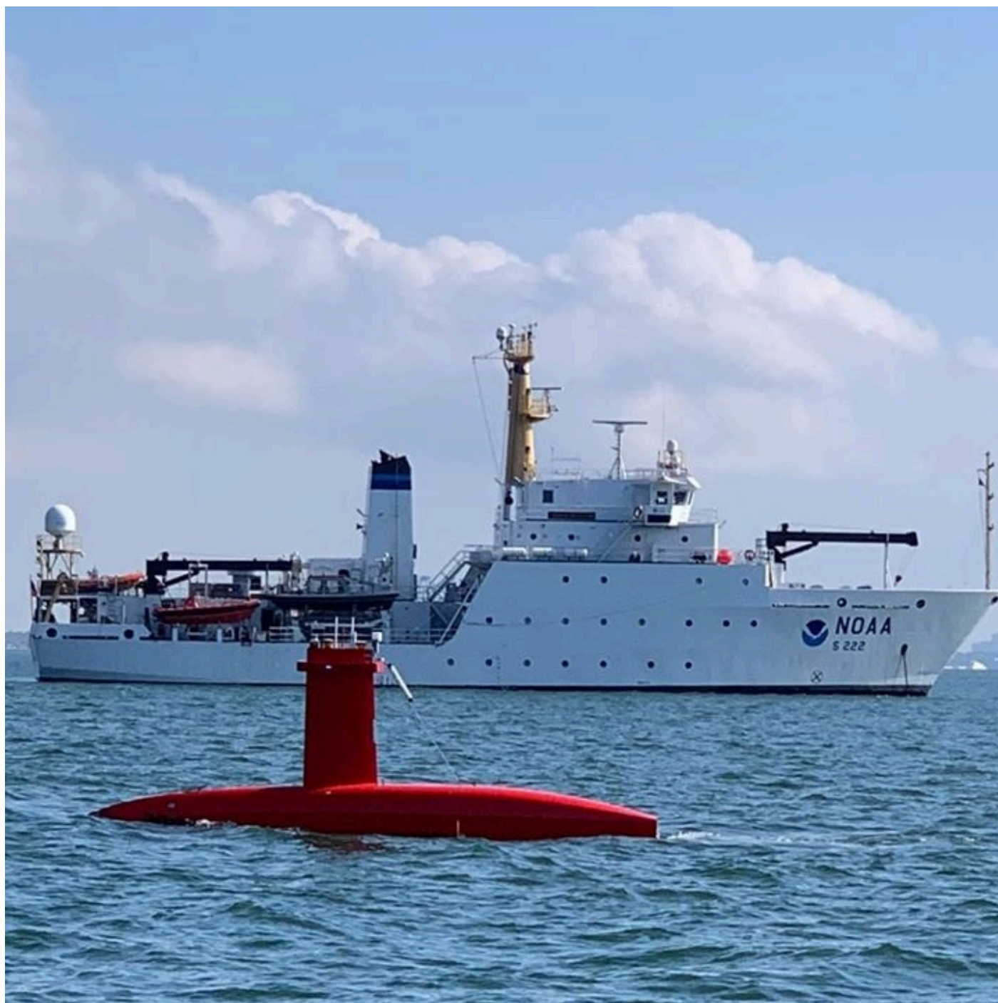
Figure 6: DriX operating through direct remote control in Norfolk, VA with NOAA Ship THOMAS JEFFERSON in the background.
