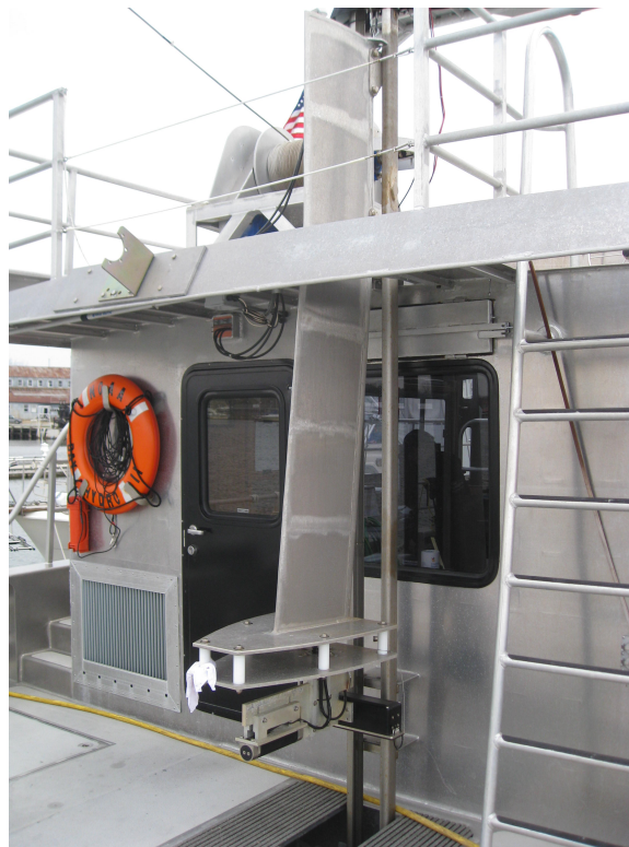
Figure 3: Mills cross multibeam projector and receiver configuration on retractable arm
