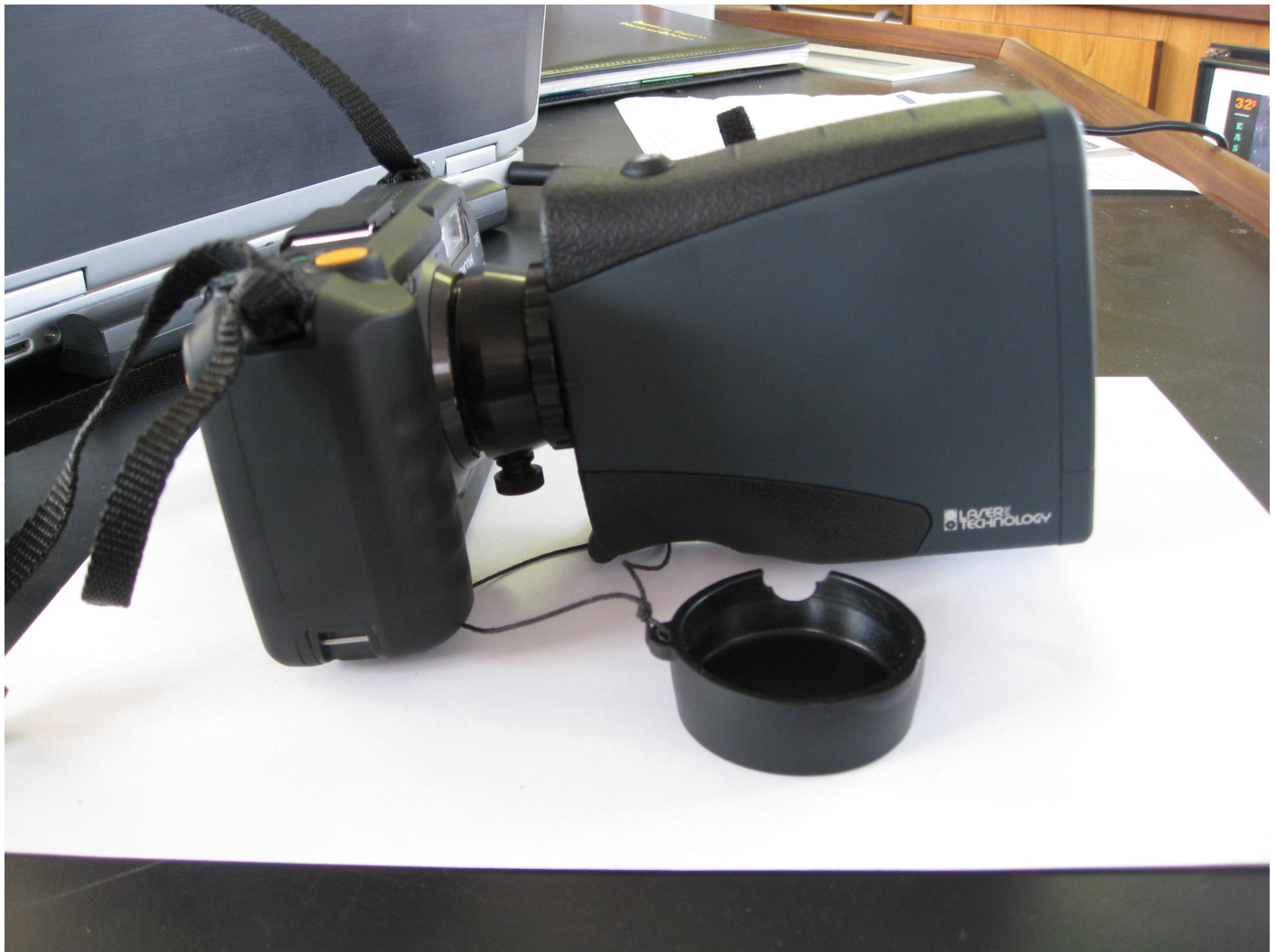
Figure 10: TruPulse 360B laser range finder configuration with Ricoh G700SE GPS camera.
