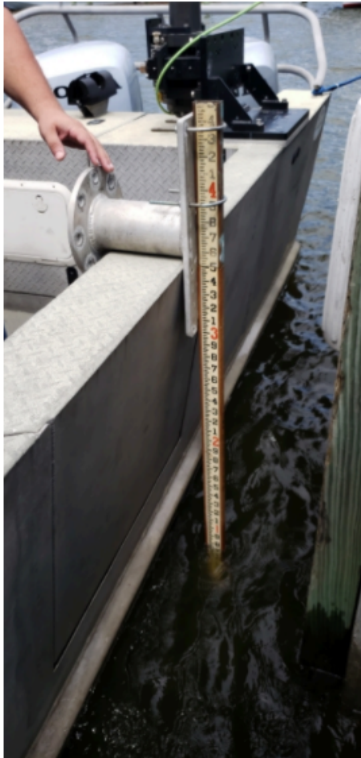
Figure 16: Static Draft Gauge made from tide staff
