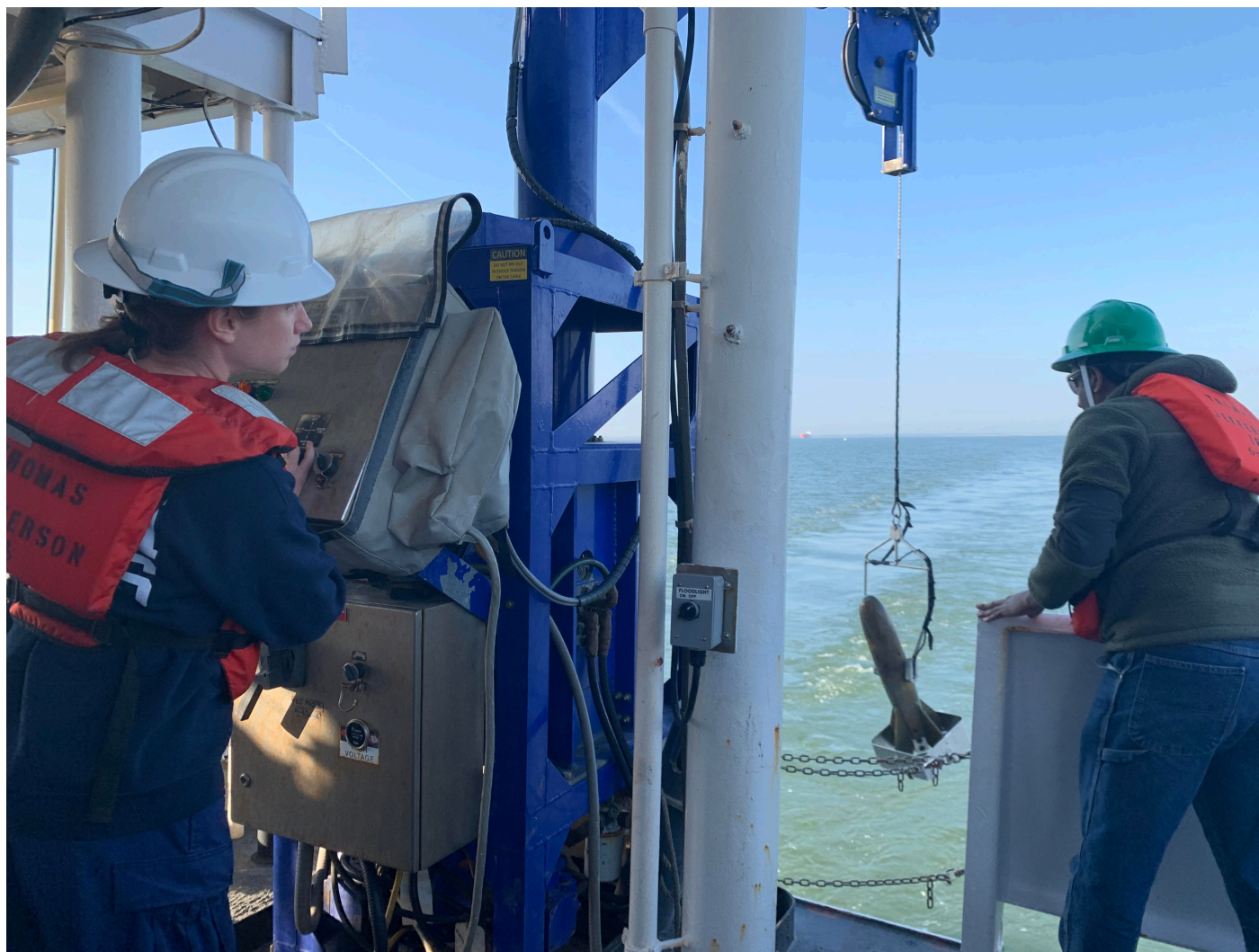
Figure 10: MVP winch and towfish system during deployment
