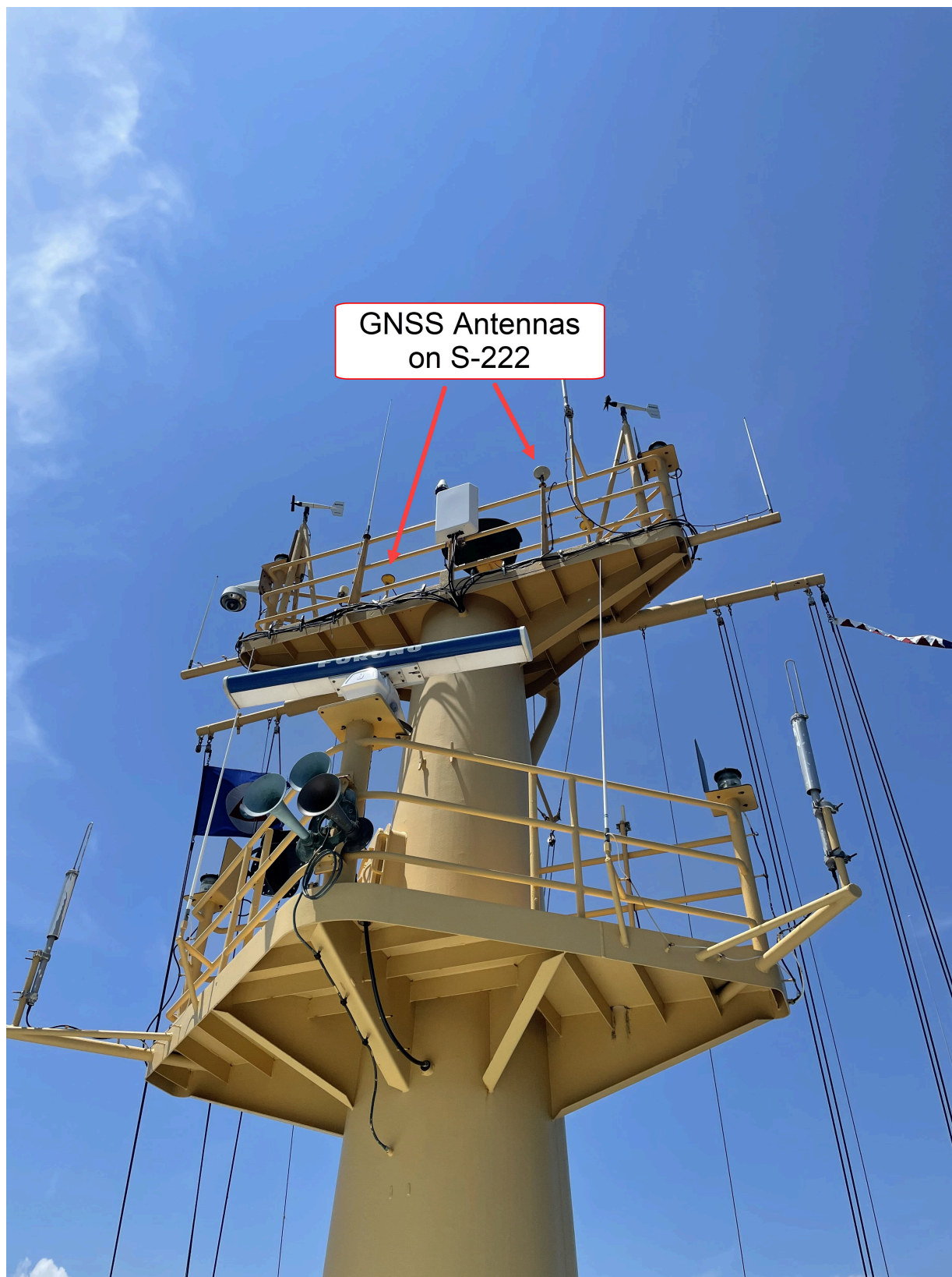
Figure 7: GNSS Antennas set up on the forward mast of S222
