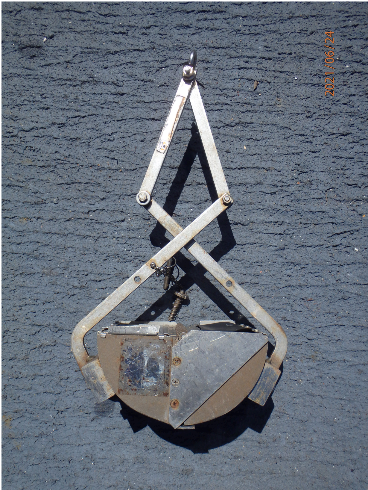
Figure 17: Petite Ponar bottom sampler in closed position
