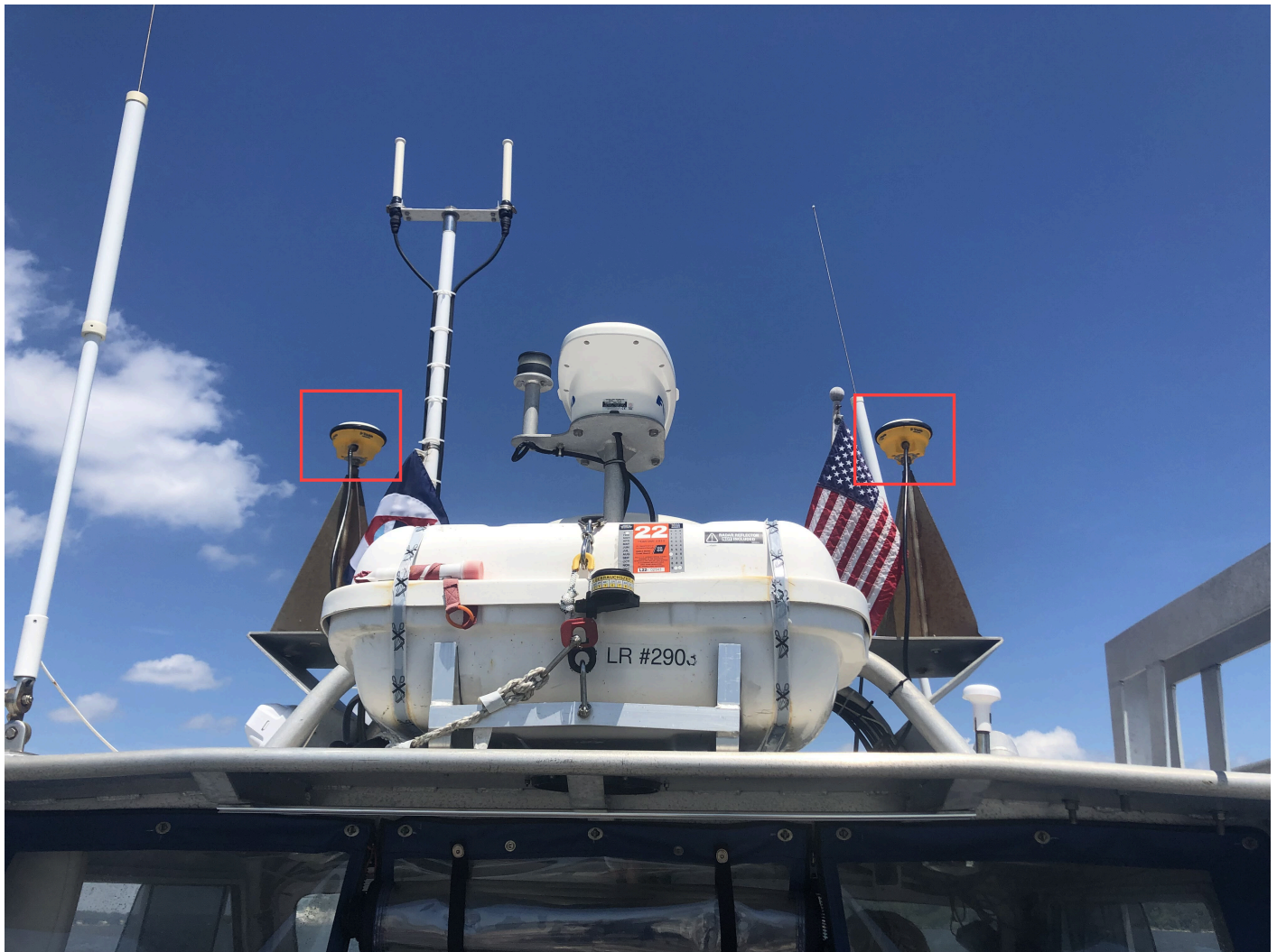
Figure 9: GNSS Antennas set up on 2903
