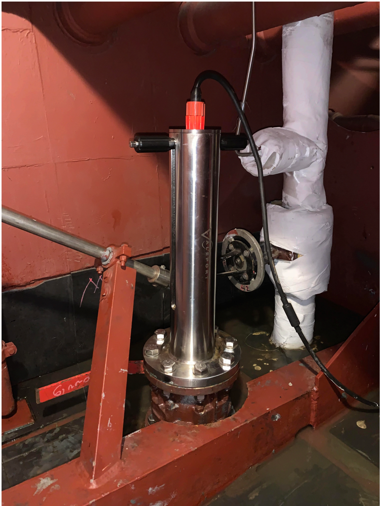
Figure 15: Valeport SVS installed in thru-hull fitting in the 'recovered' position
