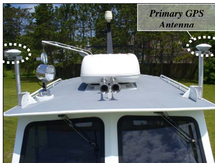
Figure 9: POS/MV Antenna Installation
