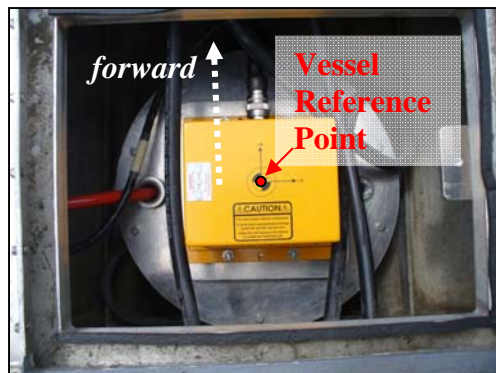
Figure 10: IMU Installation (a)
