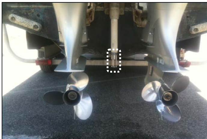
Figure 12: Surface Sound Speed Digibar Installation
