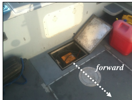
Figure 11: IMU Installation (b)
