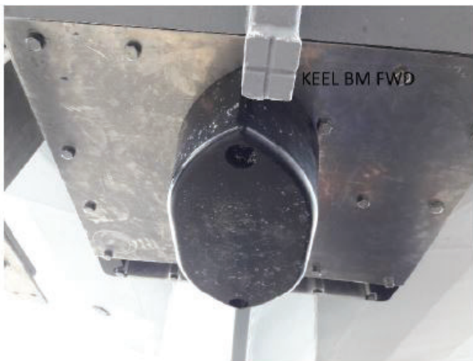
Figure 6: Installation of transducer for Odom Echotrac CV200 on the hull of 2903.
