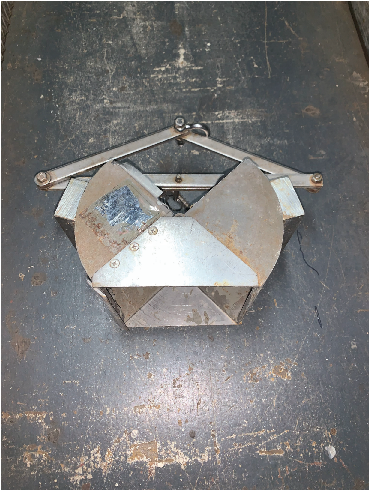
Figure 8: Ponar Wildco bottom sampler
