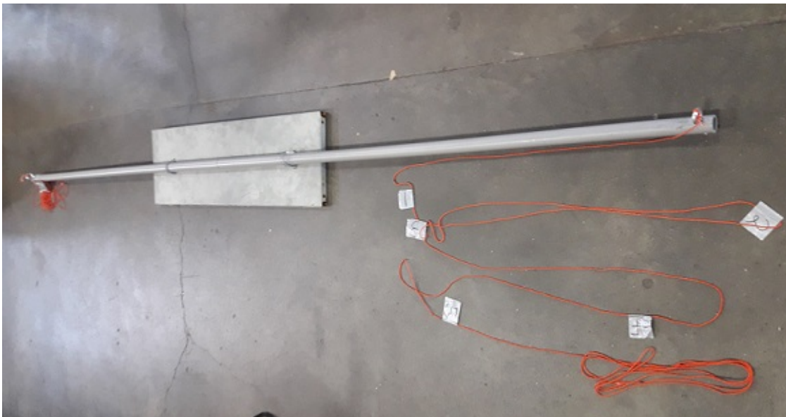
Figure 2: Bar used for bar check calibration.
