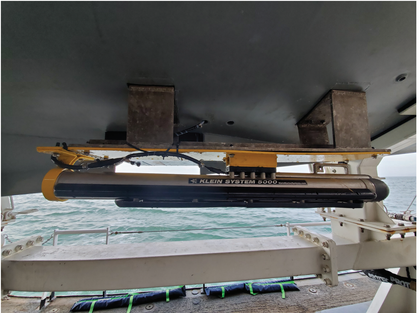
Figure 7: Klein 5000 MKII-B installed on the launch.
