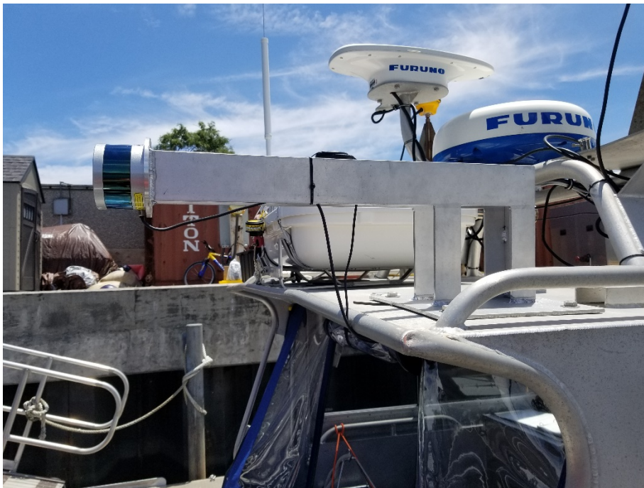
Figure 1: Installation of the Velodyne LiDAR VLP-16
