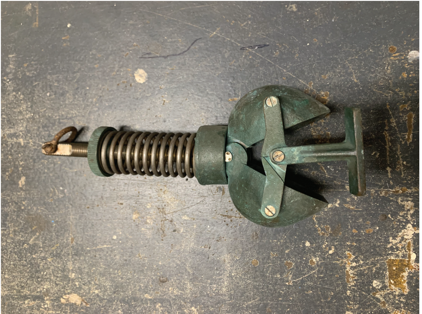
Figure 9: Kahlisco Mud Snapper bottom sampler
