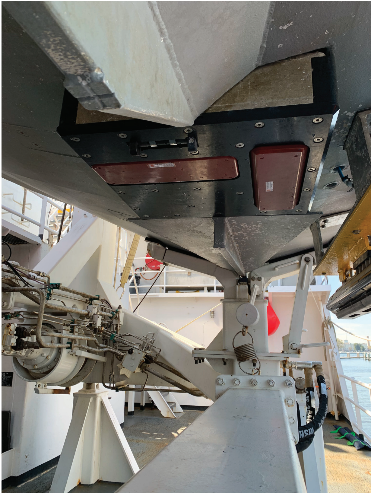
Figure 5: Kongsberg EM2040 mounting configuration on 2903 and 2904
