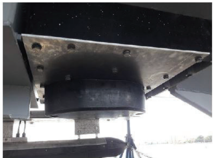
Figure 6: Installation of transducer for Odom Echotrac CV200 on the hull of 2903.
