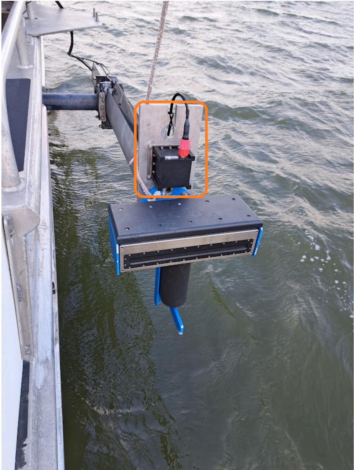
Figure 16: I2NS IMU (pole mounted)
