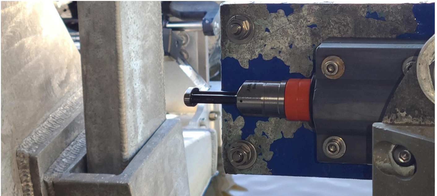
Figure 18: AML 1-RT installed on a R2Sonic 2024
