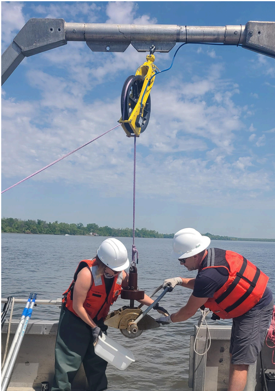
Figure 29: Shipek Grab in use for Bottom Sample Collection on R/V Endeavor
