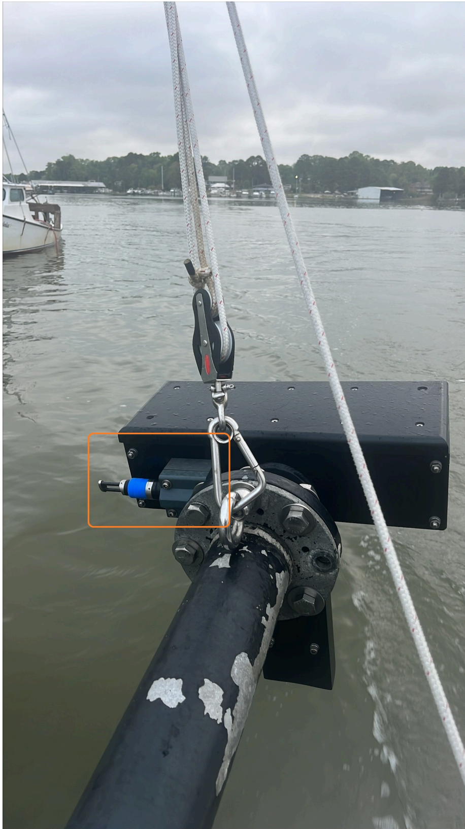
Figure 17: AML Micro•X installed on a R2Sonic 2024
