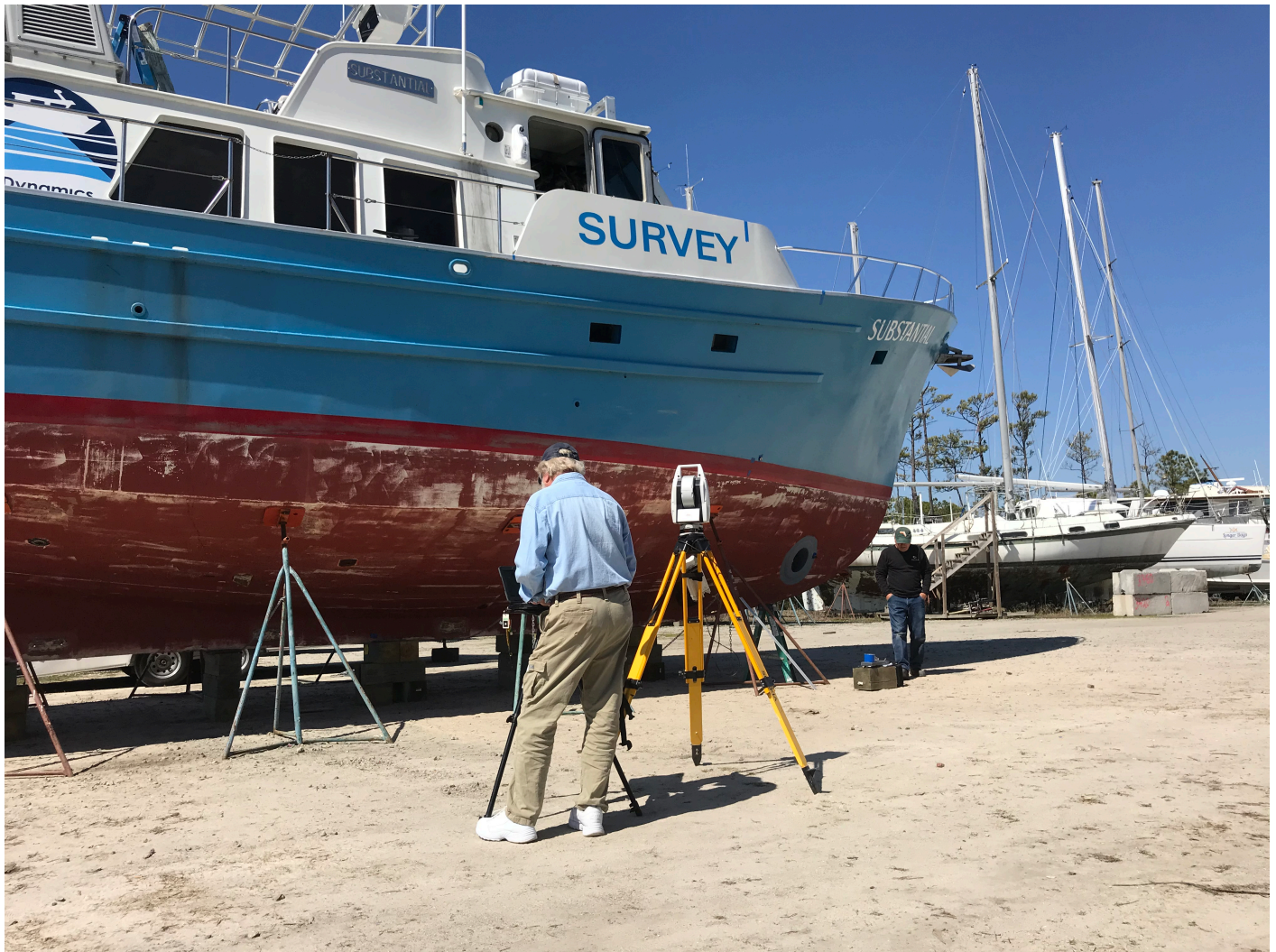
Figure 27: Static survey of R/V Substantial
