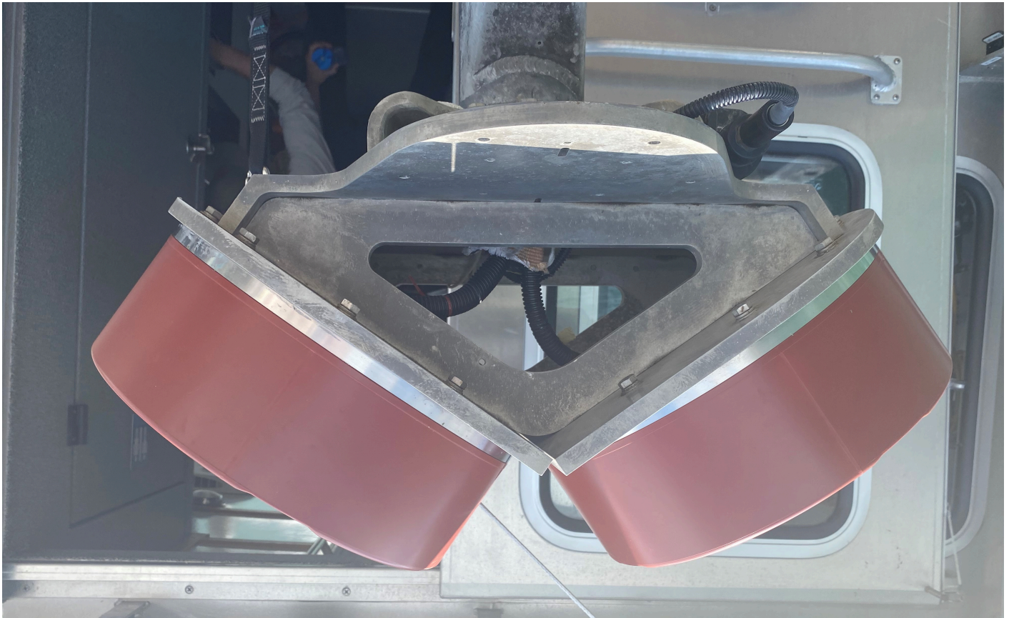
Figure 7: Kongsberg EM2040C dual-head sonar on a pole mount
