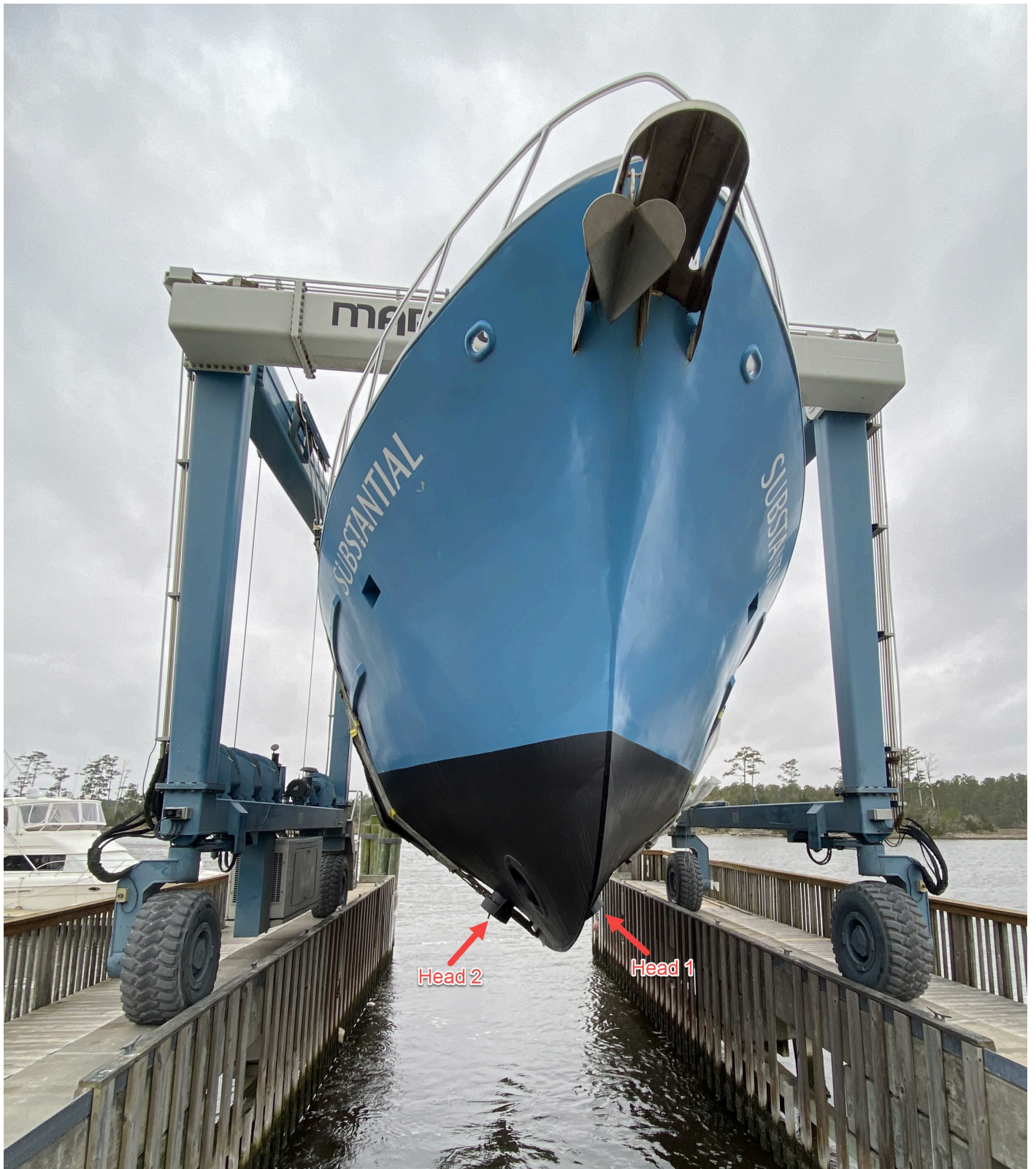
Figure 8: Kongsberg EM2040C dual-head sonar hull mounted on the R/V Substantial with each transducer labeled
