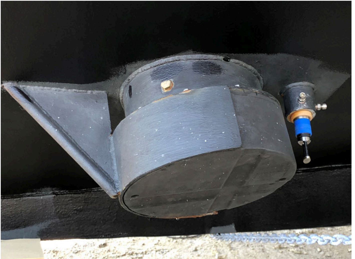
Figure 9: Kongsberg EM2040C hull mount on the R/V Substantial
