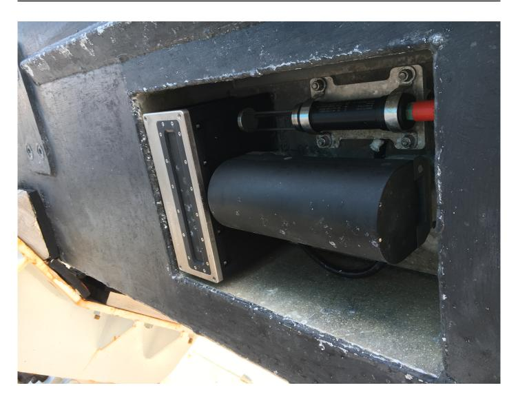
Figure 9: R2Sonic 2022 flush-mounted on hull.
