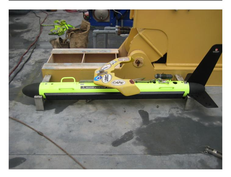
Figure 4: Klien 5000 V2 configured for towing
