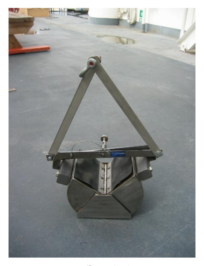
Figure 15: Ponar grab sampler
