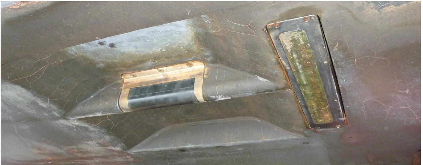
*Figure 5: 7125 Housing flush-mounted on hull.*
