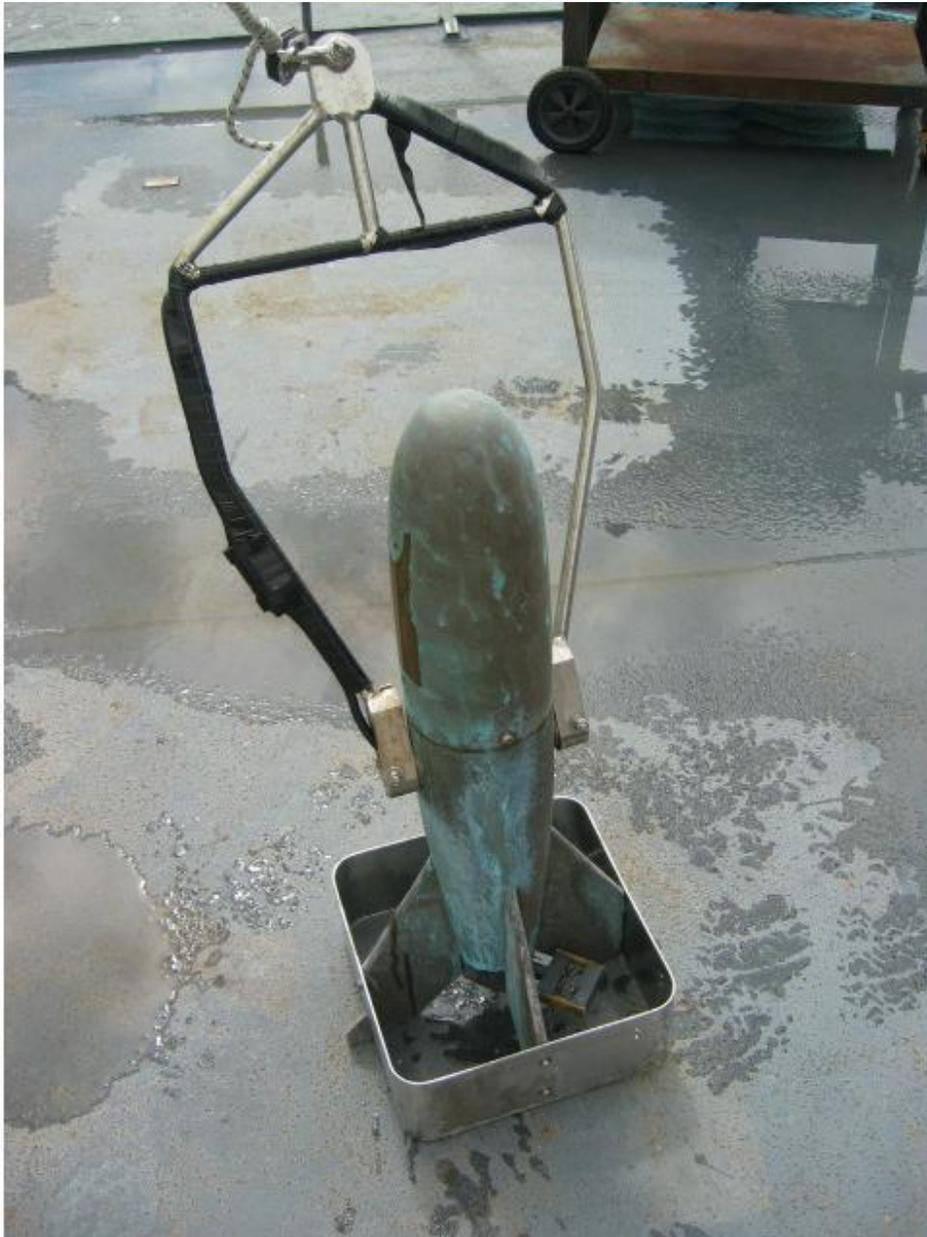
*Figure 14: MVP single sensor free fall fish.*
