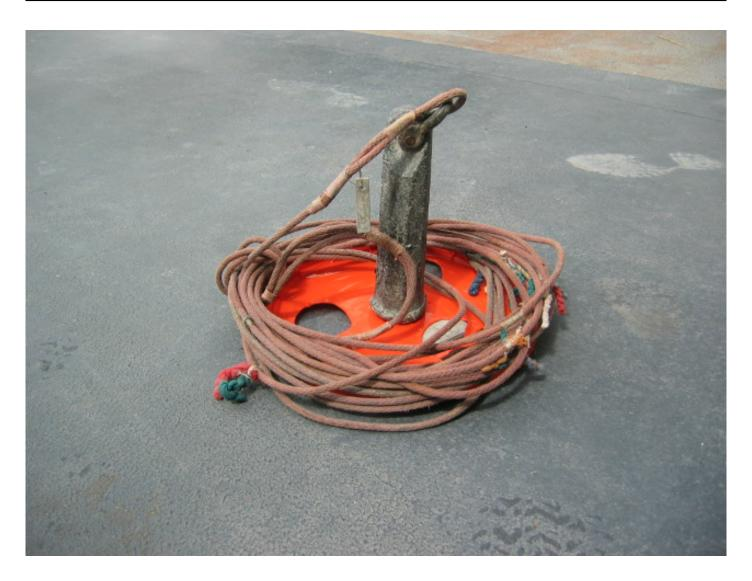
Figure 10: Leadline fitted with custom mud-shoe to limit penetration of soft bottoms.
