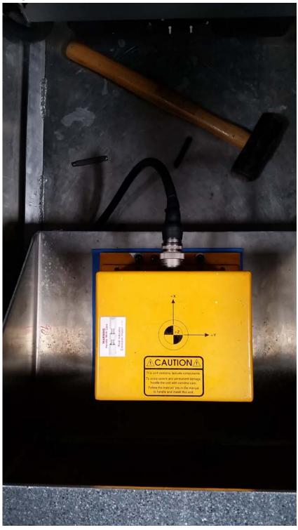
NOTE: The four corners of the IMU were observed, but presented a challenge due to low overhead above the IMU and the rounded corners of the IMU. The best attempt was made using a plumb bob and prism.
