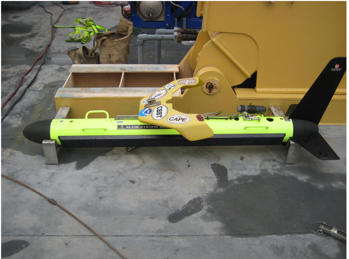
Figure 4: Klein 5000 V2 configured for towing
