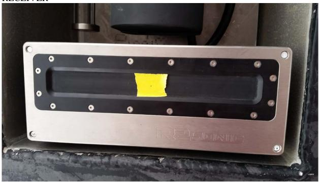
STARBOARD GPS ARP (BOTTOM OF ANTENNA)
