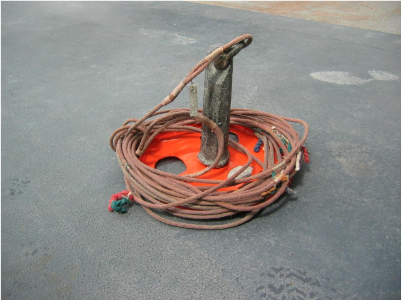
*Figure 10: Leadline fitted with custom mud-shoe to limit penetration of soft bottoms.*
