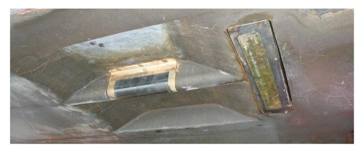
Figure 5: 7125 Housing flush-mounted on hull.
