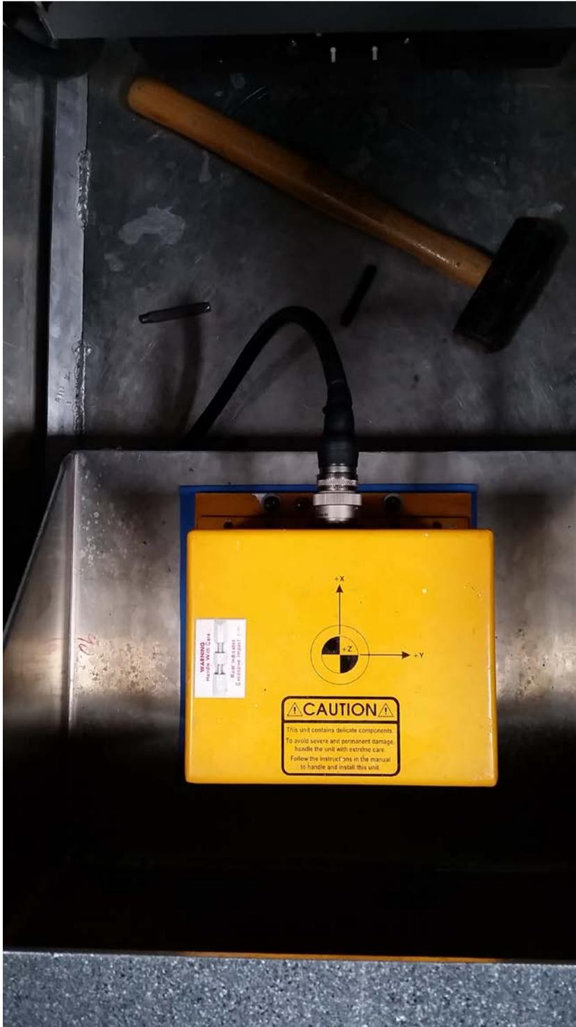
NOTE: The four corners of the IMU were observed, but presented a challenge due to low overhead above the IMU and the rounded corners of the IMU. The best attempt was made using a plumb bob and prism.
