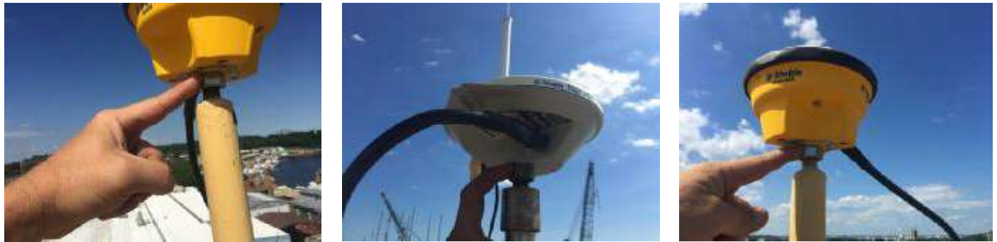
Figure 8-GPS Antenna Elevations at bottom of Mount
