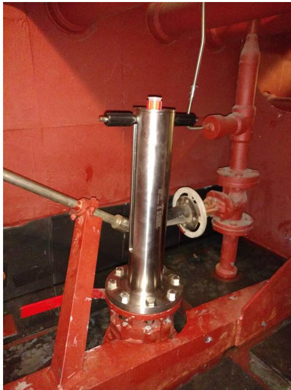
Figure 9 – The Valeport in the retracted position as mounted on a closed seacock. When the valve is open the sensor is deployed by pushing down on the black handles.
