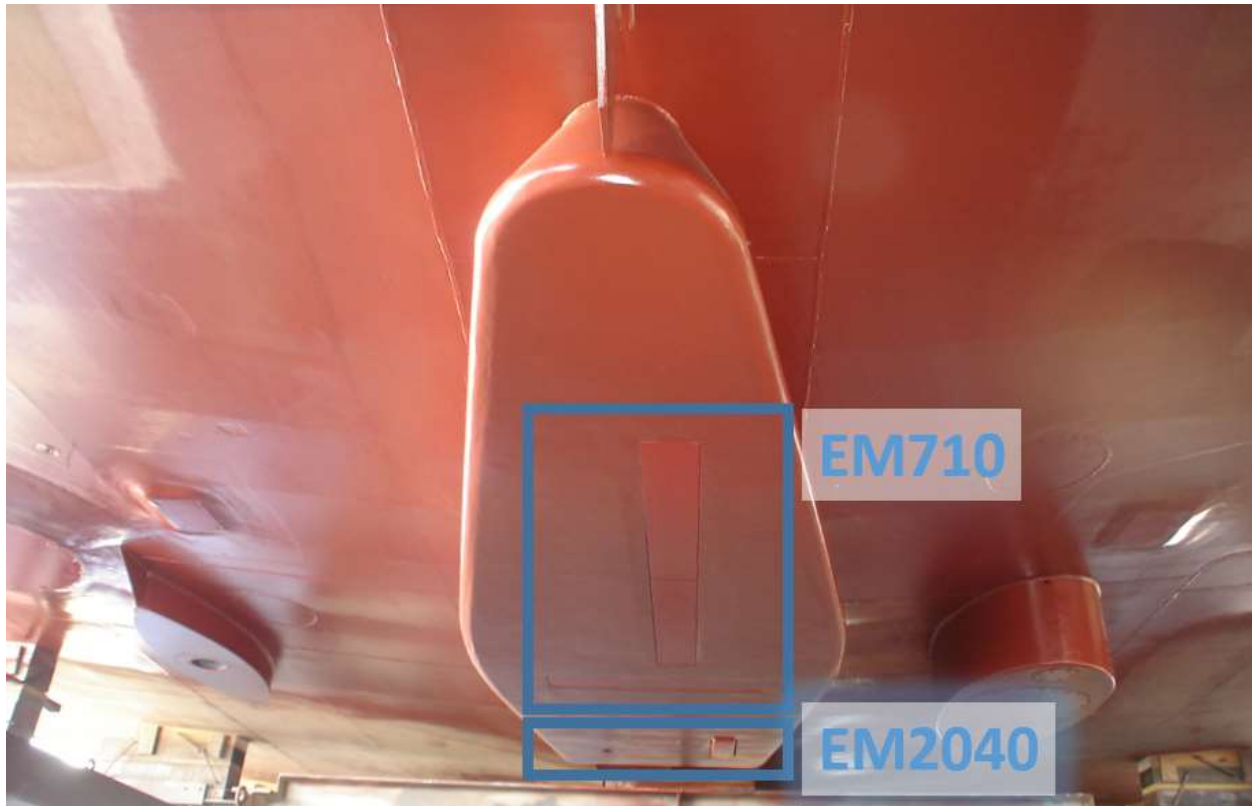
Figure 2- NOAA Ship Thomas Jefferson survey transducers from below and looking aft. The Kongsberg EM710 MKII 1° x 0.5° system includes the top two transducers in center pod, while the EM2040 system includes the bottom two. Also visible are the ES60 transducers in the pod on the right (port). The left (starboard) pod has an intake for an inboard surface sound speed sensor.
